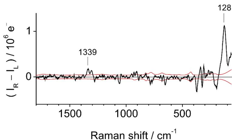
**Figure S4.** Experimental ROA spectrum of PLA dissolved in solvent DCA as accumulated for 1.1 h without intensity correction. The red lines are photon-shot-noise calculated from the parent Raman spectrum.
