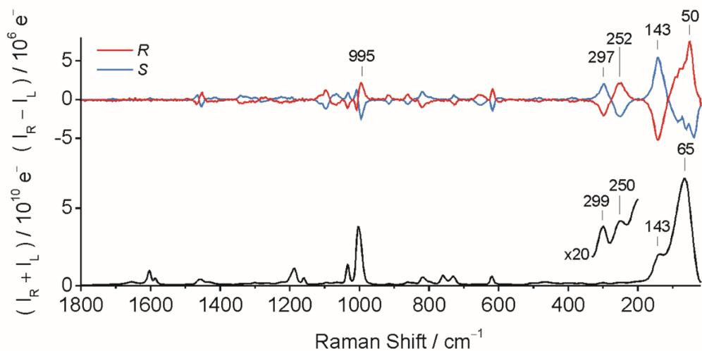
**Figure S2.** Instrumental test: Experimental ROA (top) and Raman (bottom) spectra of neat (*R*)- and (*S*)-2-phenylpropionic acid. Relative intensities were not corrected. The ROA spectra show a good “mirror image” for two enantiomers in the entire region but slightly distorted close to the filter-cut-off  $\sim 65 \text{ cm}^{-1}$ . At  $65 \text{ cm}^{-1}$ , the ROA intensity of the *R* enantiomer is 123 % of that of the *S*-enantiomer, at  $143 \text{ cm}^{-1}$  the ratio is 96 %, etc.
