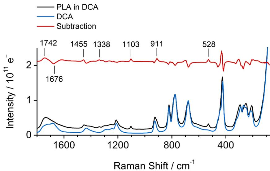
**Figure S6.** Experimental Raman spectra of PLA in solvent DCA (black), neat DCA (blue), and subtraction of the two (red, baseline was shifted for clarity). Peak frequencies indicated are those from PLA except for a decreased DCA peak at 1676  $\text{cm}^{-1}$ . Due to the solvation, the peak of DCA at 1676  $\text{cm}^{-1}$  decreased its intensity by 0.70 times compared to the neat DCA. The concentration of PLA 75 g/L corresponds to about 11 DCA molecules per one alanine residue.
