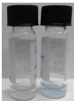
Figure S24 A solution of Cu(II)Cl 2 in D 2 O (12.5 mM) left compared to solution of Cu(II)Cl 2 in D 2 O (12.5 mM) with G5-PAMAM-GGA-NH 2 (100 \mu M).
