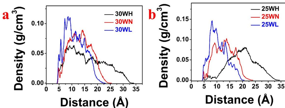
Figure S1. Density of polymer by z-axis at temperatures 300 K and 250 K with models – (a) 30WH, 30WN, 30WL; (b) 25WH, 25WN, 25WL.
