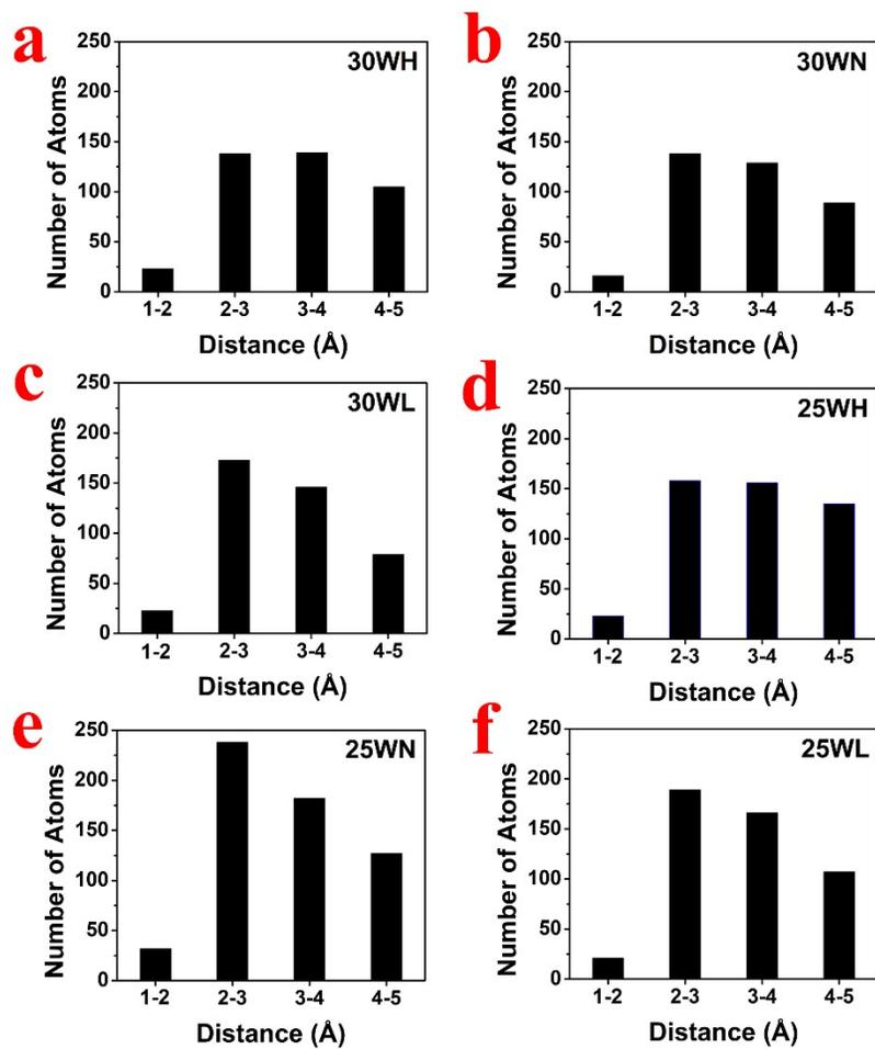
Figure S4. Number of oxygen atoms around polyrotaxane in the last frame at 300 K and 250 K for WH, WN, and WL systems.
