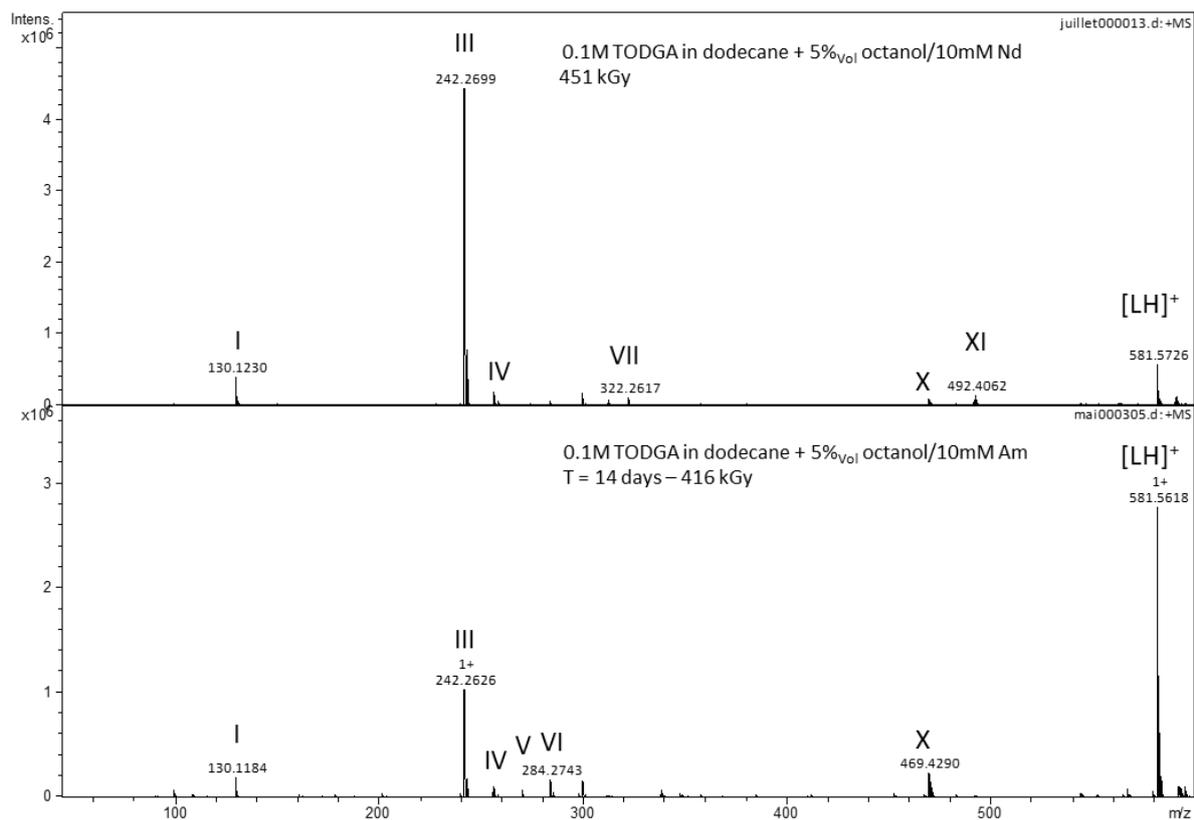
Figure S2: ESI-MS spectra (low mass range) of TODGA solutions (top) loaded with 10 mmol L<sup>-1</sup> of Nd (gamma ex-situ irradiation at  $\approx$  450 kGy) or (bottom) 10 mmol L<sup>-1</sup> of Am (alpha in-situ irradiation at  $\approx$  420 kGy). Conditions: Org phase: 0.1 mol L<sup>-1</sup> TODGA in dodecane + 5% octanol Aq Phase: Nd(III) or Am(III) in 2.5 mol L<sup>-1</sup> HNO<sub>3</sub>.
