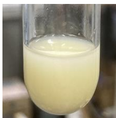
Fig. S1 Reaction mixture of pyridine, THF, TFA, H 2 O 2 , and the pristine TiO 2 photocatalyst (JRC-TIO-6).
