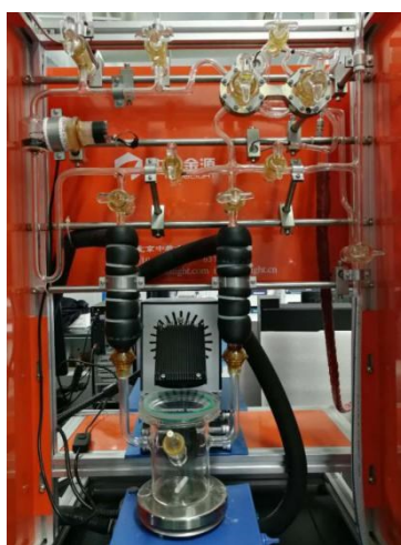
Figure S1. Schematic diagram of the photocatalytic reduction CO 2 system.
