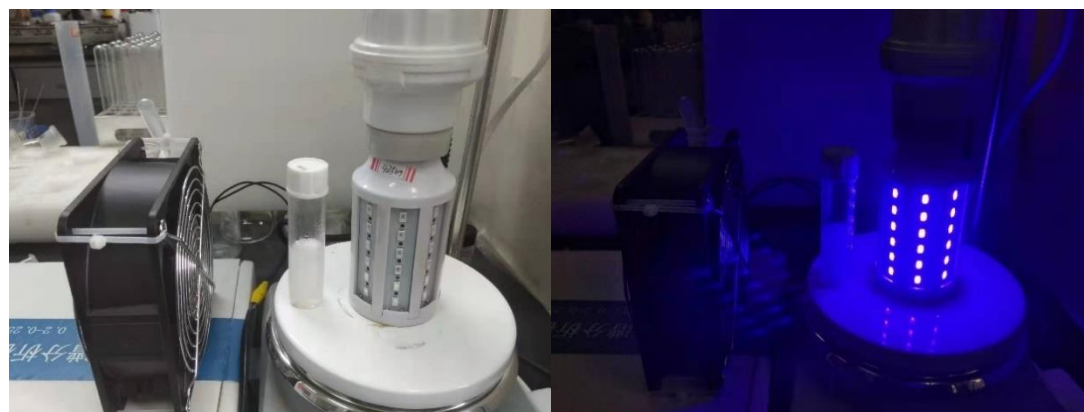
Fig. S12 The spectrum of (a) simulated solar spectrum, (b) solar spectrum, (c) light spectrum; (d) The picture of the reaction under the purple lamp (15 W, 425 nm, 13.4\text{mW}/\text{cm}^2 ).
