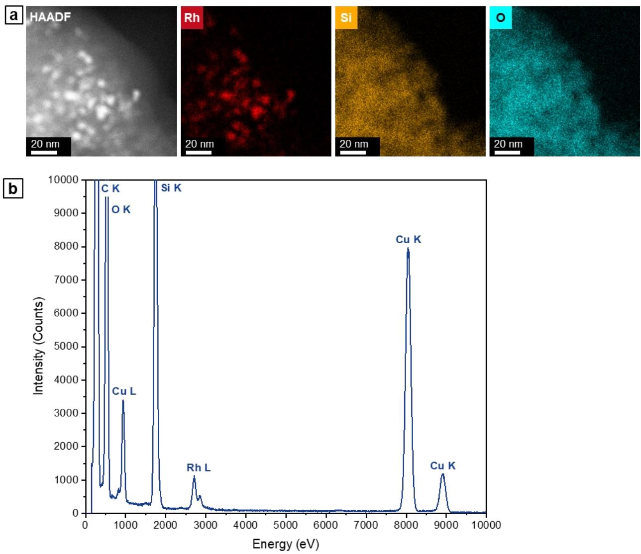
**Figure S4.** STEM-EDX analysis of reduced Rh/SiO<sub>2</sub> catalyst: (a) HAADF micrograph, single-element maps (Rh L, Si K, O K), and (b) corresponding EDX spectrum.
