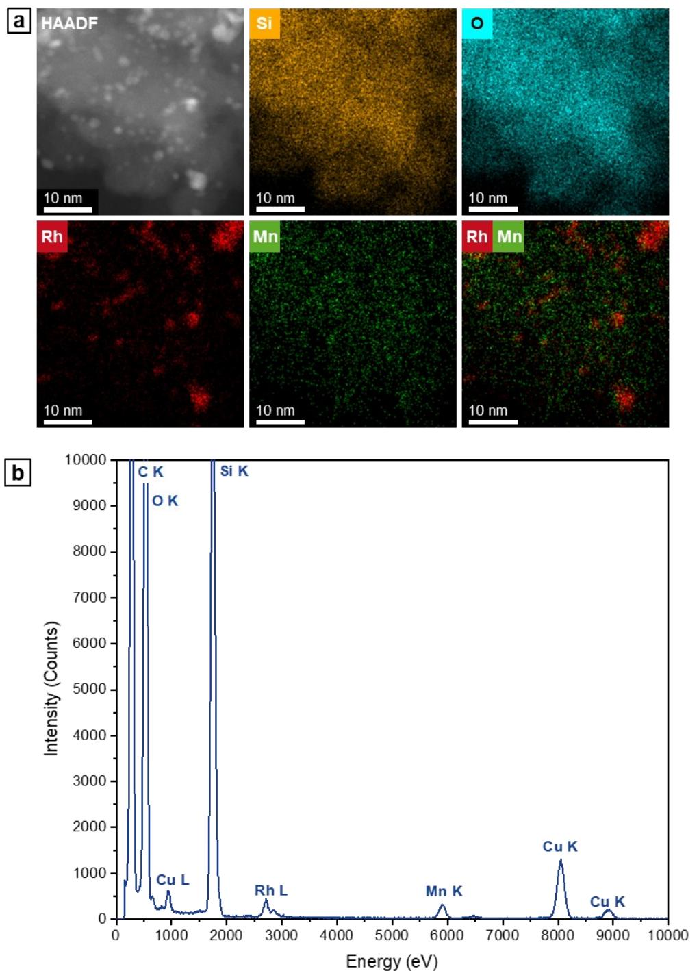
**Figure S6.** STEM-EDX analysis of RhMn/SiO<sub>2</sub> catalyst after long-term catalytic study: (a) HAADF micrograph, single-element maps (Rh L, Si K, O K, Mn K), superimposed map of Rh L and Mn K, and (b) corresponding EDX spectrum.
