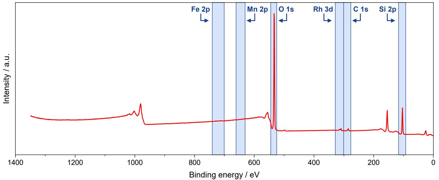
**Figure S28.** XP survey spectrum of calcined RhFe/SiO<sub>2</sub> catalyst. Regions selected for high-resolution spectra are highlighted in blue.
