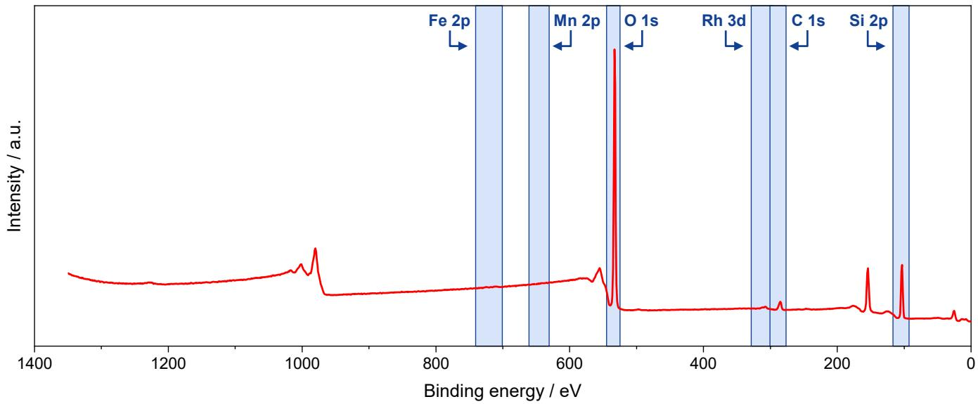
**Figure S30.** XP survey spectrum of RhFe/SiO<sub>2</sub> catalyst after high temperature investigation. Regions selected for high-resolution spectra are highlighted in blue.
