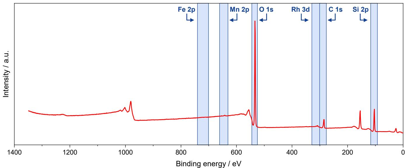
**Figure S33.** XP survey spectrum of reduced RhMnFe/SiO<sub>2</sub> catalyst. Regions selected for high-resolution spectra are highlighted in blue.
