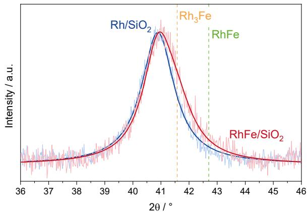
**Figure S13.** X-ray diffractograms after long-term catalytic study of  $\text{Rh/SiO}_2$  (blue) and  $\text{RhFe/SiO}_2$  (red) in the region of the (111) reflections. For the full X-ray diffractograms see Figure 1.  $\text{RhFe}$  reference (green; C25-1408) has been taken from ICDD database.  $\text{Rh}_3\text{Fe}$  reference (orange; 347421) has been calculated from Open Quantum Materials Database (OQMD).
