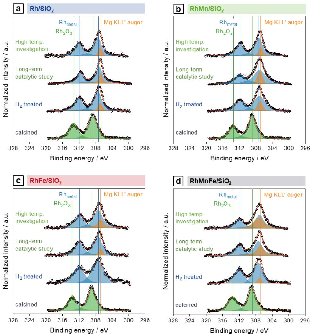
**Figure S1.** Rh 3d XP spectra of (a) Rh/SiO<sub>2</sub>, (b) RhMn/SiO<sub>2</sub>, (c) RhFe/SiO<sub>2</sub>, and (d) RhMnFe/SiO<sub>2</sub> in four different states: calcined, reduced, after long-term catalytic study, and after high temperature stability investigation.
