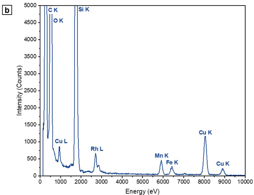
**Figure S15.** STEM-EDX analysis of RhMnFe/SiO<sub>2</sub> catalyst after long-term catalytic study: (a) HAADF micrograph, single-element maps (Rh L, Si K, O K, Fe K, Mn K), superimposed maps of Rh L, Mn K, and Fe K, and (b) corresponding EDX spectrum.
