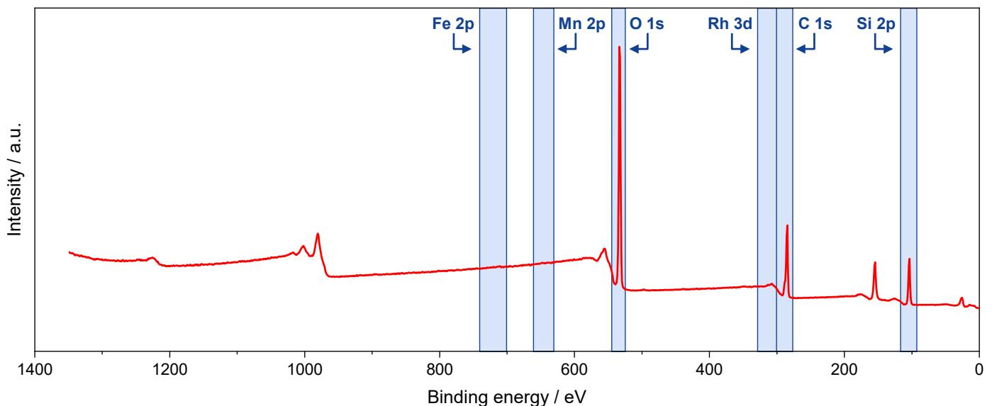
**Figure S29.** XP survey spectrum of reduced RhFe/SiO<sub>2</sub> catalyst. Regions selected for high-resolution spectra are highlighted in blue.
