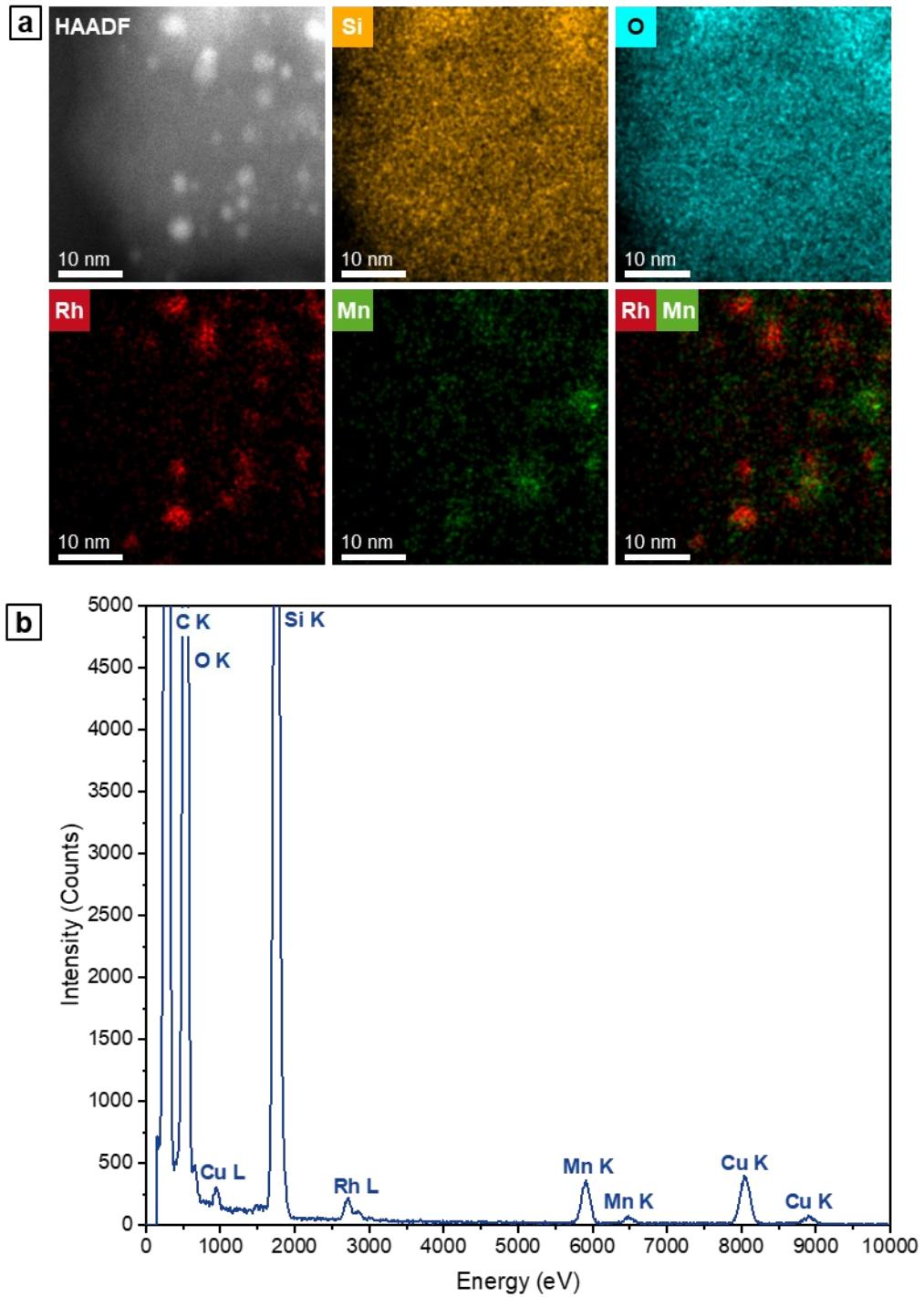
**Figure S5.** STEM-EDX analysis of reduced RhMn/SiO<sub>2</sub> catalyst: (a) HAADF micrograph, single-element maps (Rh L, Si K, O K, Mn K), superimposed map of Rh L and Mn K, and (b) corresponding EDX spectrum.
