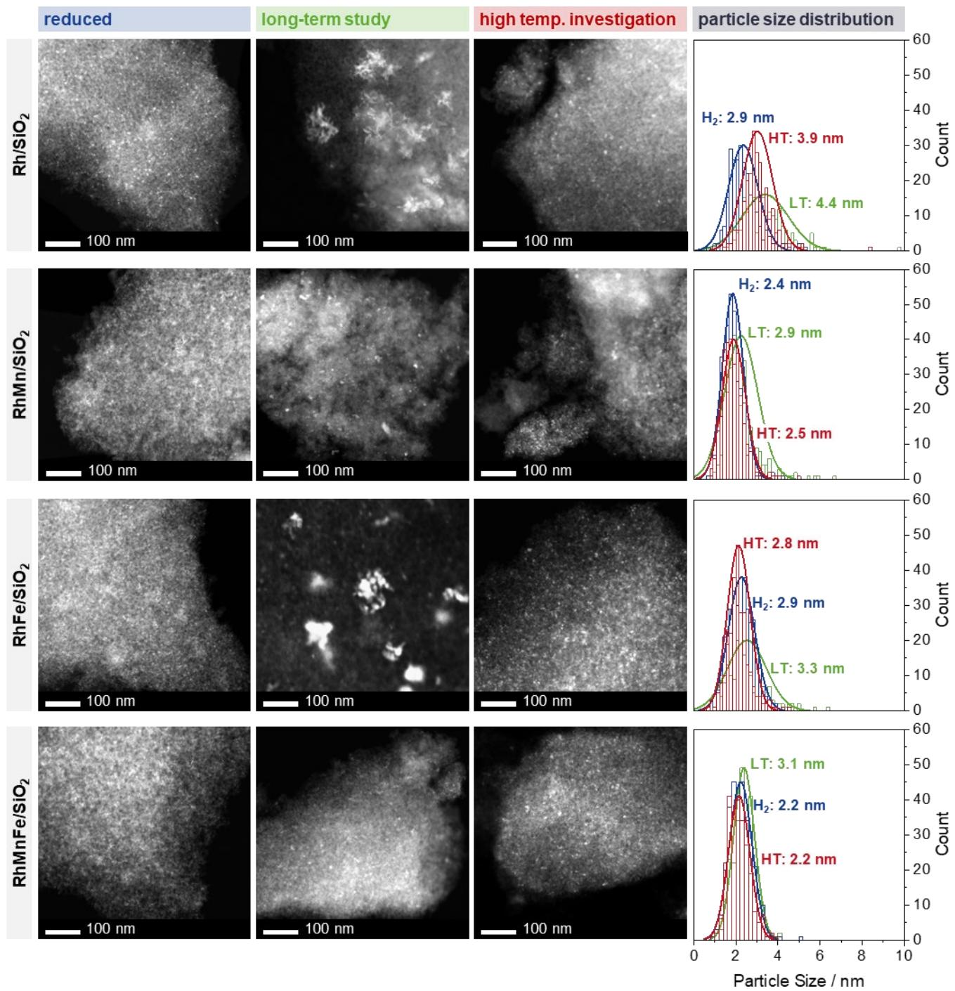
**Figure S3.** Overview HAADF-STEM images of Rh/SiO<sub>2</sub>, RhMn/SiO<sub>2</sub>, RhFe/SiO<sub>2</sub>, and RhMnFe/SiO<sub>2</sub> and corresponding particle size distributions.
