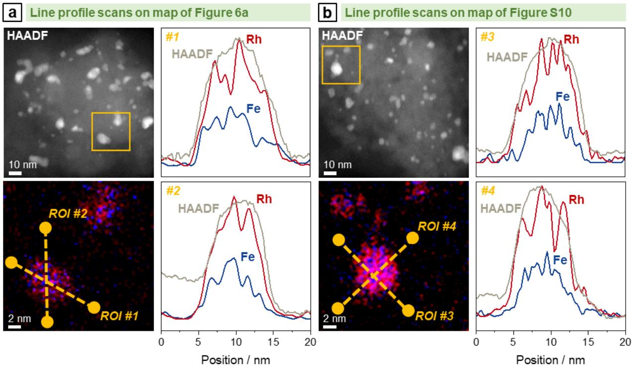
**Figure S11.** Additional STEM-EDX line profile analysis of RhFe/SiO<sub>2</sub> catalyst after long-term catalytic study from two different domains. For additional single-element maps and corresponding EDX spectrum of (a) see Figure S8 and (b) see Figure S10.
