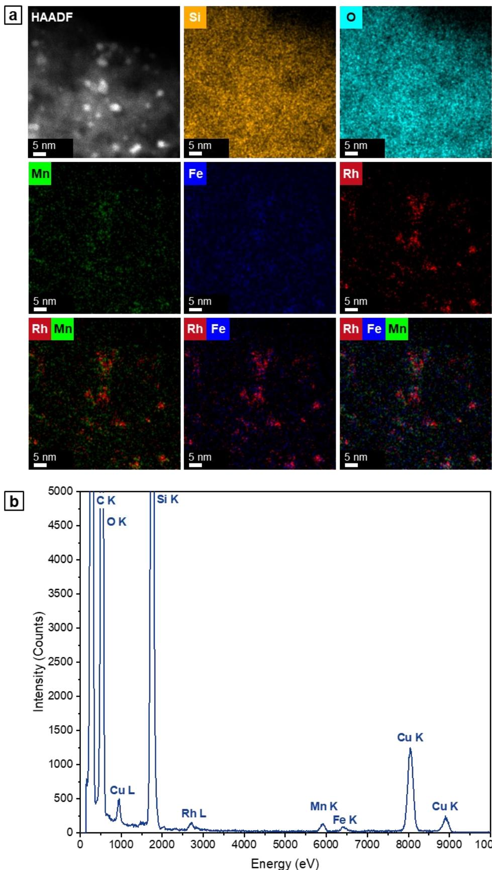
**Figure S14.** STEM-EDX analysis of reduced RhMnFe/SiO<sub>2</sub> catalyst: (a) HAADF micrograph, single-element maps (Rh L, Si K, O K, Fe K, Mn K), superimposed maps of Rh L, Mn K, and Fe K, and (b) corresponding EDX spectrum.
