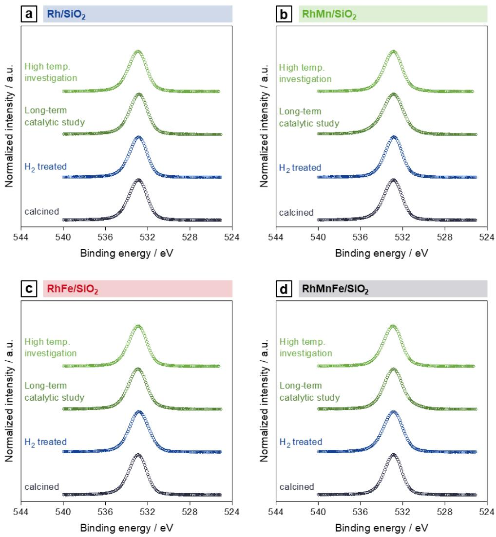
**Figure S19.** O 1s XP spectra of (a) Rh/SiO<sub>2</sub>, (b) RhMn/SiO<sub>2</sub>, (c) RhFe/SiO<sub>2</sub>, and (d) RhMnFe/SiO<sub>2</sub> in four different states: calcined, reduced, after long-term catalytic study, and after high temperature stability investigation.
