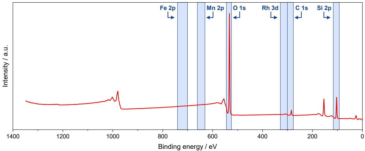
**Figure S25.** XP survey spectrum of reduced RhMn/SiO<sub>2</sub> catalyst. Regions selected for high-resolution spectra are highlighted in blue.
