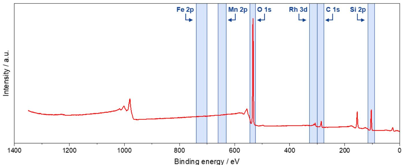
**Figure S23.** XP survey spectrum of Rh/SiO<sub>2</sub> catalyst after long-term study. Regions selected for high-resolution spectra are highlighted in blue.
