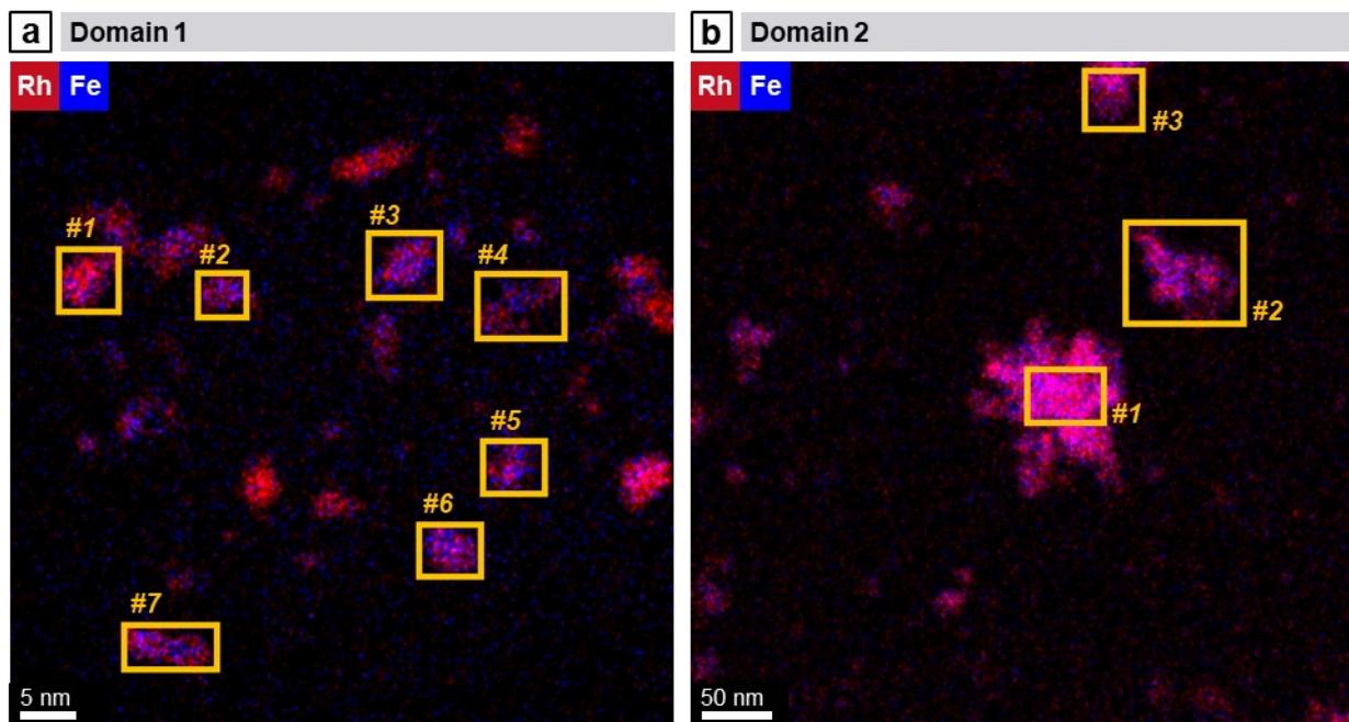
**Figure S12.** STEM-EDX area-selective analysis of RhFe/SiO<sub>2</sub> after long-term catalytic study. Investigated areas are highlighted in yellow. Corresponding elemental compositions area provided in Table S2.
