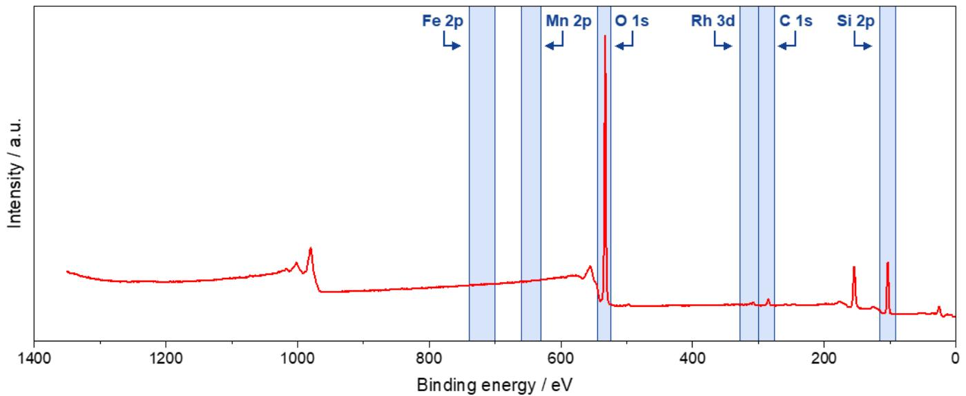
**Figure S22.** XP survey spectrum of Rh/SiO<sub>2</sub> catalyst after high temperature investigation. Regions selected for high-resolution spectra are highlighted in blue.
