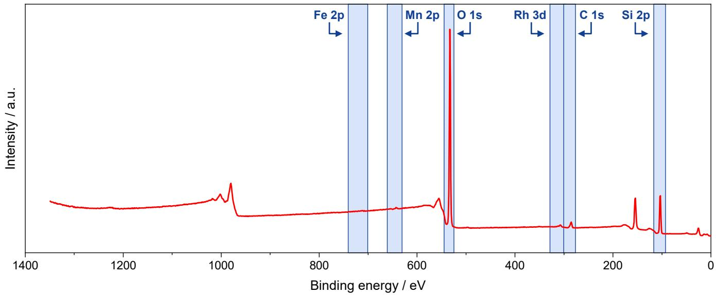
**Figure S34.** XP survey spectrum of RhMnFe/SiO<sub>2</sub> catalyst after high temperature investigation. Regions selected for high-resolution spectra are highlighted in blue.
