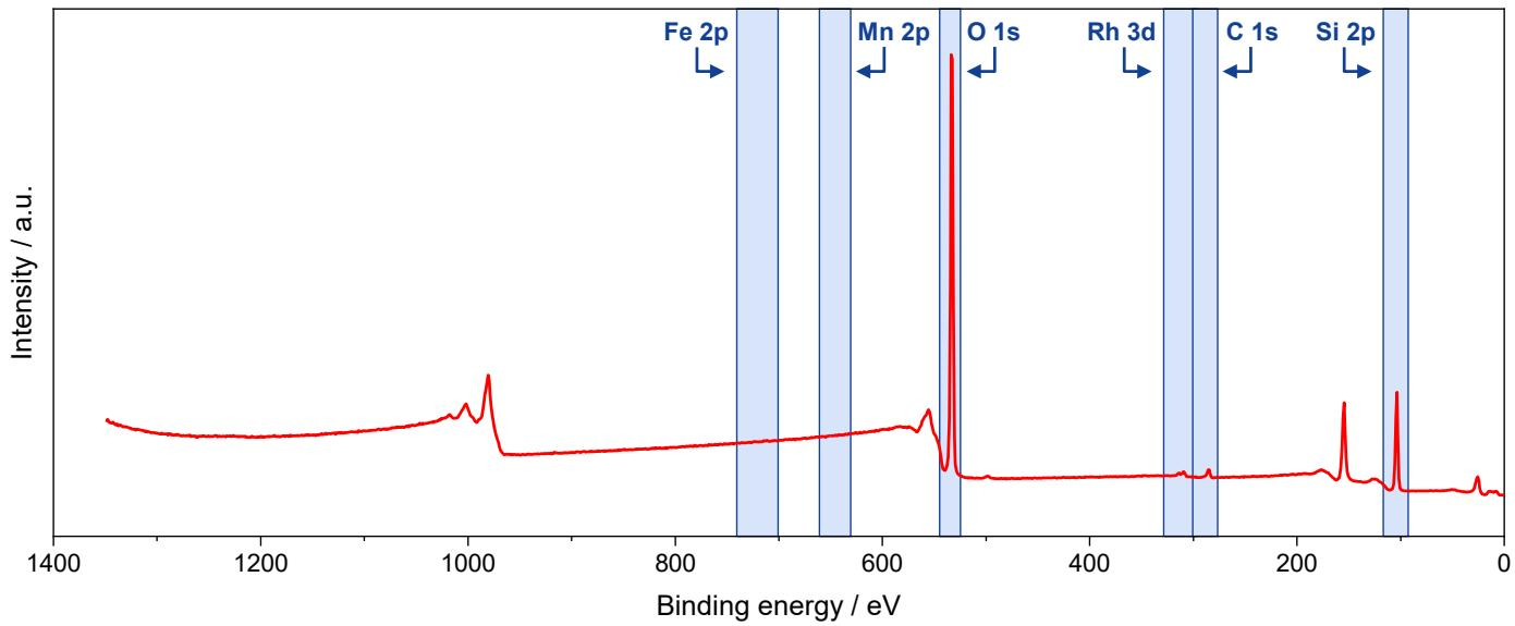
**Figure S24.** XP survey spectrum of calcined RhMn/SiO<sub>2</sub> catalyst. Regions selected for high-resolution spectra are highlighted in blue.
