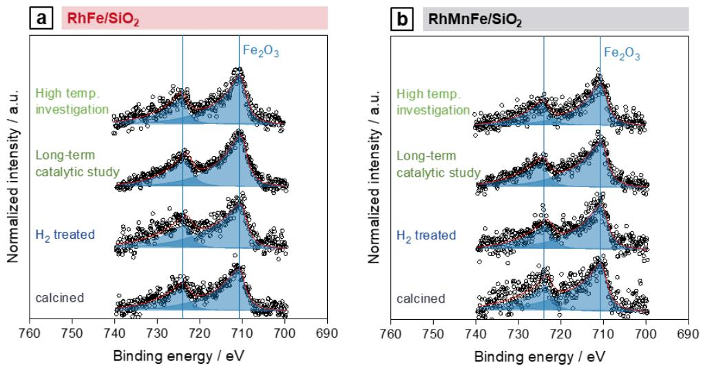
**Figure S2.** Fe 2p XP spectra of (a) RhFe/SiO<sub>2</sub> and (b) RhMnFe/SiO<sub>2</sub> in four different states: calcined, reduced, after long-term catalytic study, and high temperature stability investigation.
