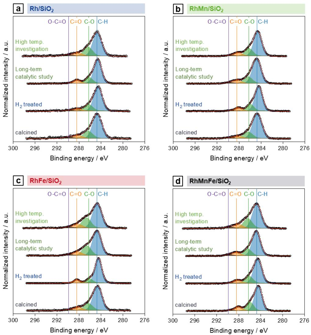
**Figure S17.** C 1s XP spectra of (a) Rh/SiO<sub>2</sub>, (b) RhMn/SiO<sub>2</sub>, (c) RhFe/SiO<sub>2</sub>, and (d) RhMnFe/SiO<sub>2</sub> in four different states: calcined, reduced, after long-term catalytic study, and after high temperature stability investigation.
