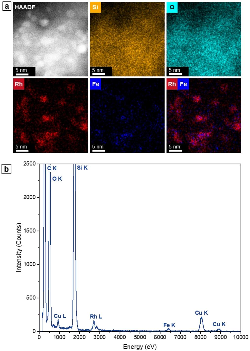
**Figure S7.** STEM-EDX analysis of reduced RhFe/SiO<sub>2</sub> catalyst: (a) HAADF micrograph, single-element maps (Rh L, Si K, O K, Fe K), superimposed map of Rh L and Fe K, and (b) corresponding EDX spectrum.
