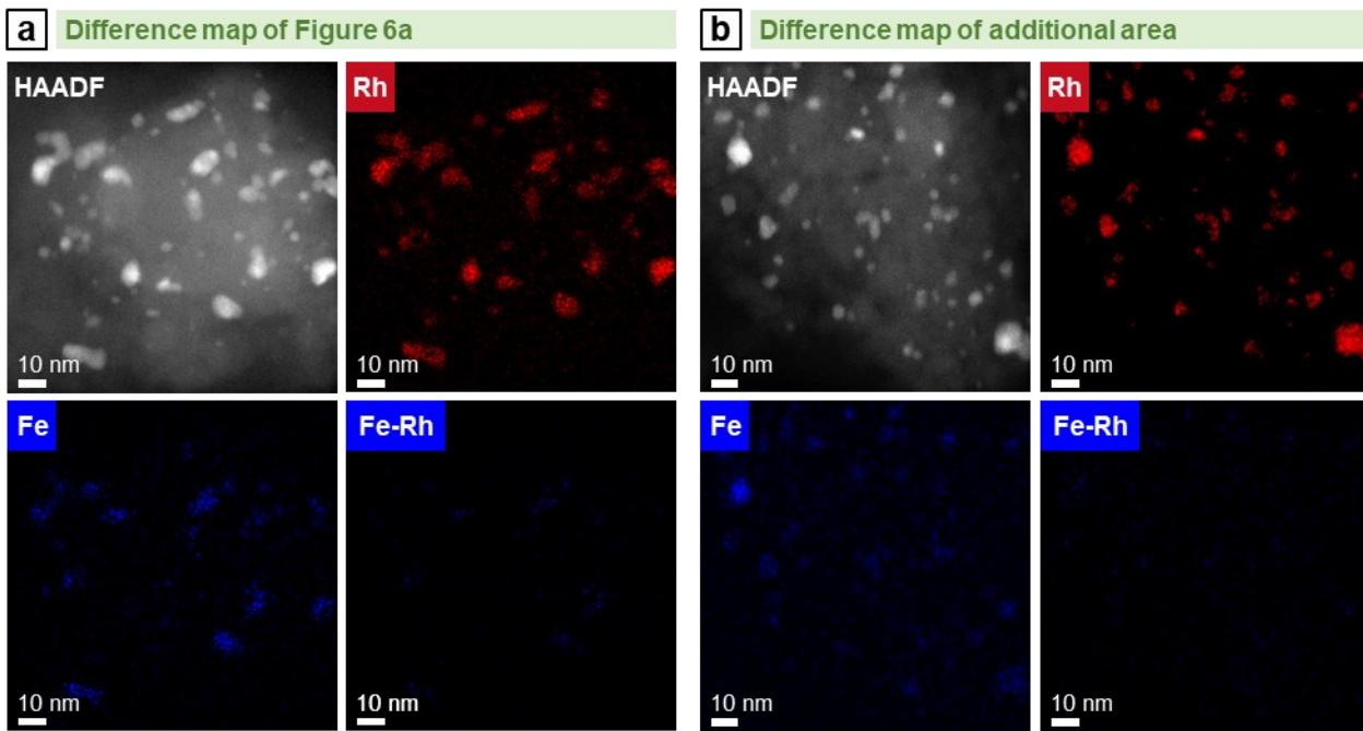
**Figure S9.** STEM-EDX mapping of RhFe/SiO<sub>2</sub> after long-term catalytic study (54 bar, max. 260 °C; 530 h on stream) within two different domains. Rh L and Fe K EDX signals were used. For additional single-element maps and corresponding EDX spectrum of (a) see Figure S8 and (b) see Figure S10.
