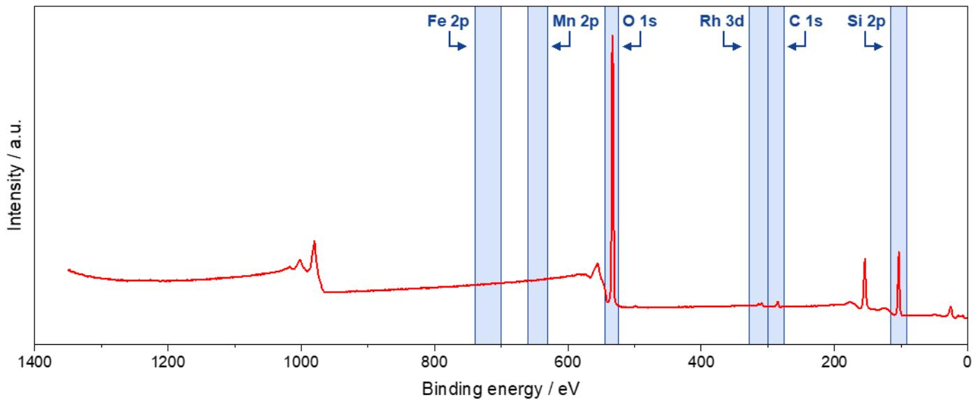
**Figure S20.** XP survey spectrum of calcined Rh/SiO<sub>2</sub> catalyst. Regions selected for high-resolution spectra are highlighted in blue.
