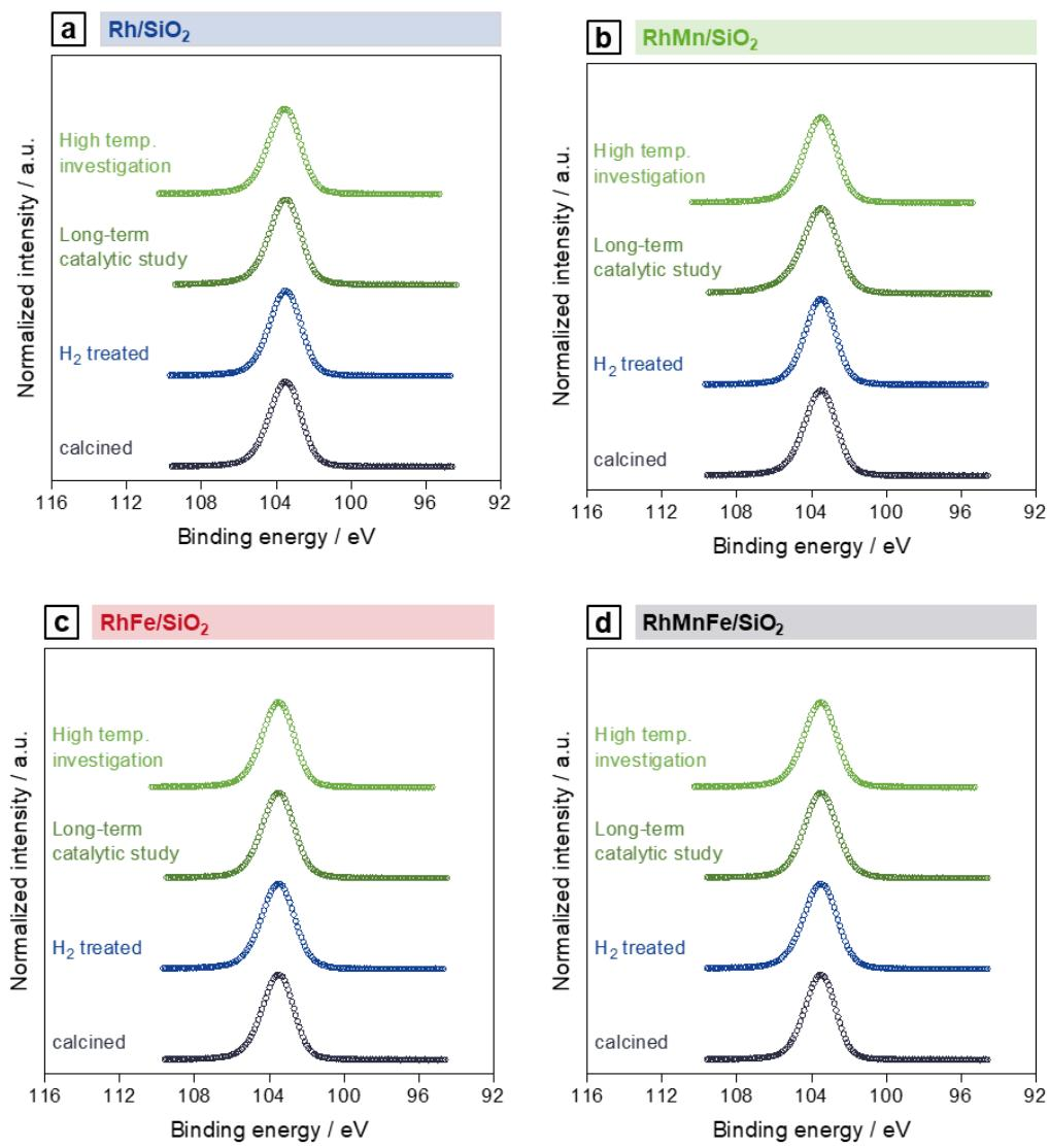
**Figure S18.** Si 2p XP spectra of (a) Rh/SiO<sub>2</sub>, (b) RhMn/SiO<sub>2</sub>, (c) RhFe/SiO<sub>2</sub>, and (d) RhMnFe/SiO<sub>2</sub> in four different states: calcined, reduced, after long-term catalytic study, and after high temperature stability investigation.
