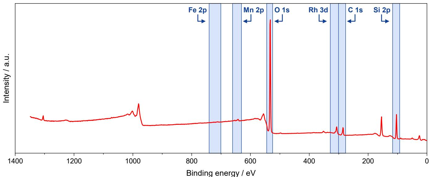
**Figure S35.** XP survey spectrum of RhMnFe/SiO<sub>2</sub> catalyst after long-term study. Regions selected for high-resolution spectra are highlighted in blue.
