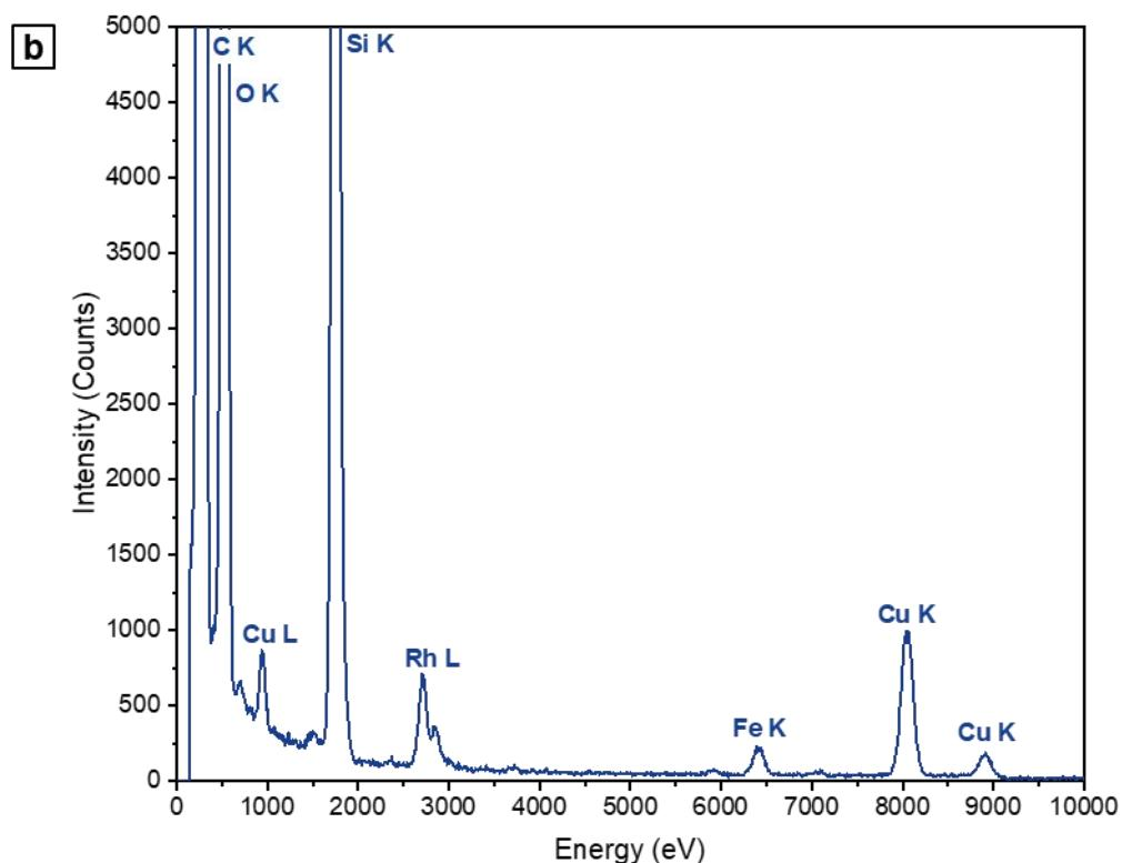
**Figure S8.** STEM-EDX analysis of RhFe/SiO<sub>2</sub> catalyst after long-term catalytic study: (a) HAADF micrograph, single-element maps (Rh L, Si K, O K, Fe K), superimposed map of Rh L and Fe K, and (b) corresponding EDX spectrum.
