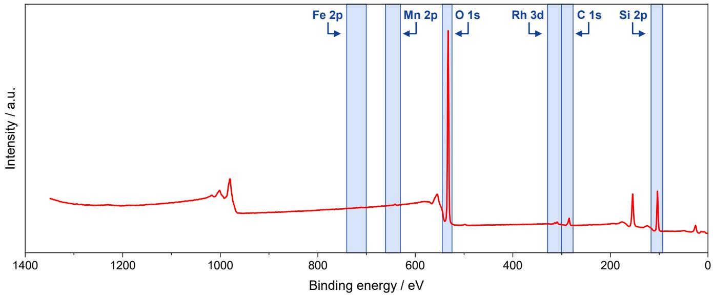
**Figure S32.** XP survey spectrum of calcined RhMnFe/SiO<sub>2</sub> catalyst. Regions selected for high-resolution spectra are highlighted in blue.
