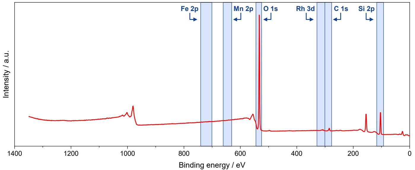
**Figure S26.** XP survey spectrum of RhMn/SiO<sub>2</sub> catalyst after high temperature investigation. Regions selected for high-resolution spectra are highlighted in blue.
