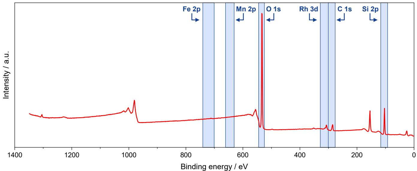
**Figure S31.** XP survey spectrum of RhFe/SiO<sub>2</sub> catalyst after long-term study. Regions selected for high-resolution spectra are highlighted in blue.
