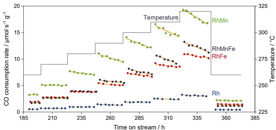
**Figure S16.** Linear regression for all four catalyst and each temperature step. Fit curves are highlighted in orange. Corresponding activity loss rates are given in Table S3.
