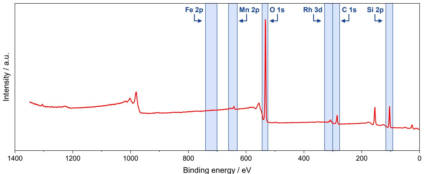
**Figure S27.** XP survey spectrum of RhMn/SiO<sub>2</sub> catalyst after long-term study. Regions selected for high-resolution spectra are highlighted in blue.
