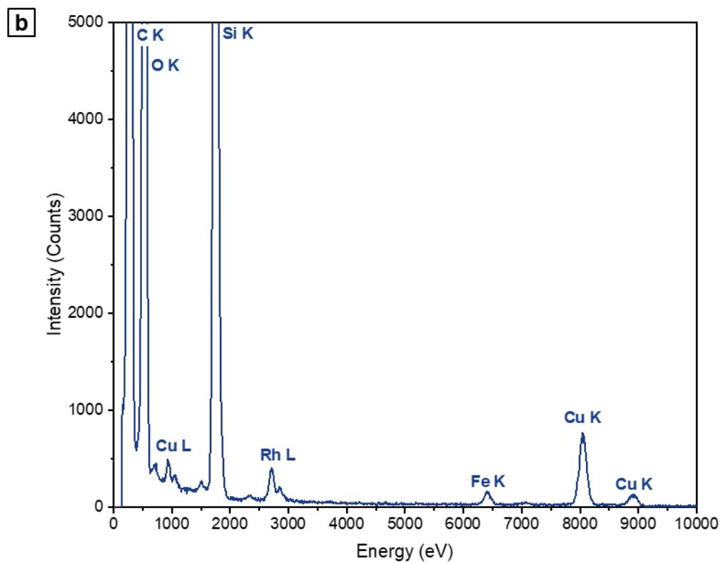
**Figure S10.** Additional STEM-EDX analysis of RhFe/SiO<sub>2</sub> catalyst after long-term catalytic study: (a) HAADF micrograph, single-element maps (Rh L, Si K, O K, Fe K), superimposed map of Rh L and Fe K, and (b) corresponding EDX spectrum.
