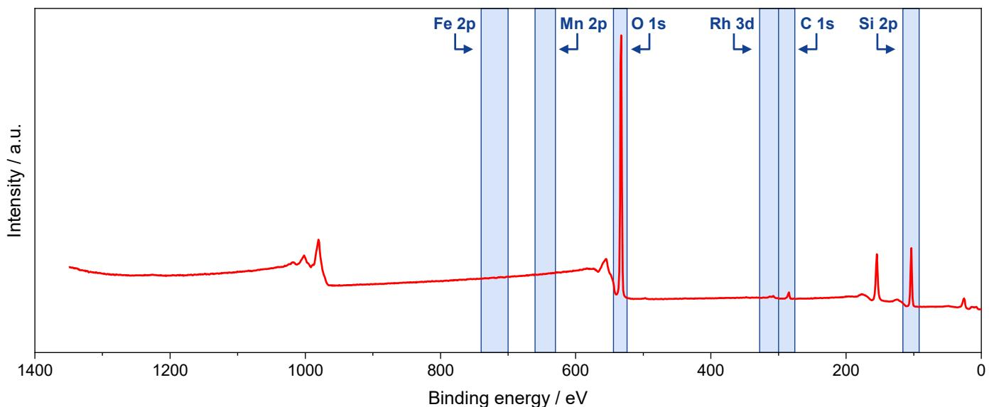
**Figure S21.** XP survey spectrum of reduced Rh/SiO<sub>2</sub> catalyst. Regions selected for high-resolution spectra are highlighted in blue.
