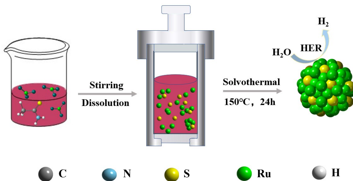
Scheme S1 Schematic illustration for the synthetic process of Ru-S catalyst.
