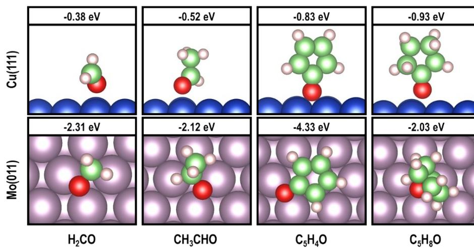
**Figure S2.** Top views of the adsorption sites and adsorption energies for the studied isolated deoxygenation products on Cu(111) and Mo(011) surfaces. Color code as in Figure S1.
