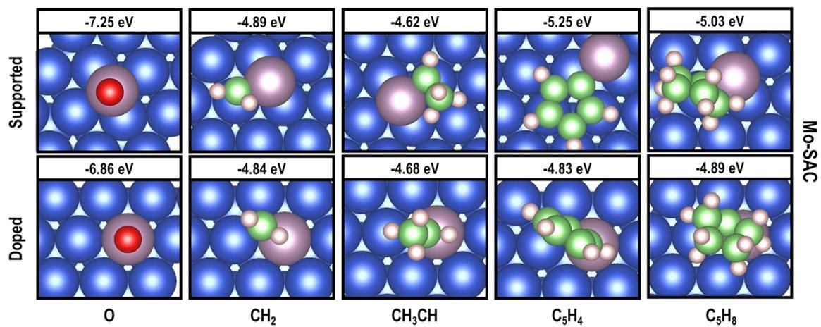
**Figure S7.** Top views of the adsorption sites and adsorption energies for the co-adsorbed products of the deoxygenation reactions on either a supported- or a doped-Mo SAC. Color code as in Figure S1.
