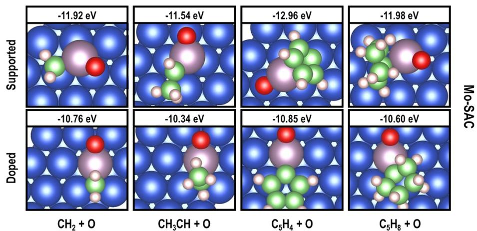
**Figure S8.** Top views of the adsorption sites and reaction energy barriers for the obtained transition states of the studied deoxygenation reactions explored on either a supported- or a doped-Mo SAC. Color code as in Figure S1.
