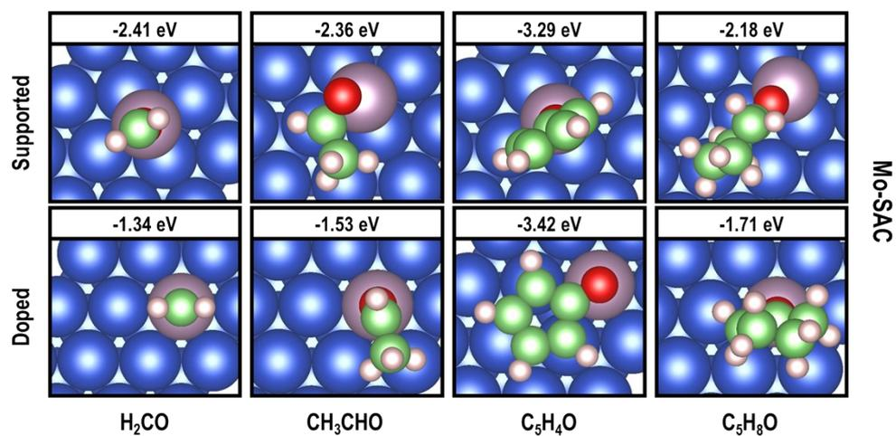
**Figure S6.** Top views of the adsorption sites and adsorption energies for the isolated reaction products on either a supported- or a doped-Mo SAC. Color code as in Figure S1.
