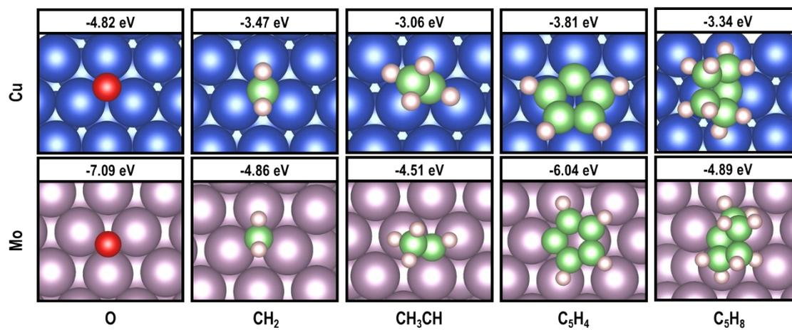
**Figure S3.** Top views of the adsorption sites and adsorption energies for the co-adsorbed products of the deoxygenation reactions as studied on Cu(111) and Mo(011) surfaces. Color code as in Figure S1.
