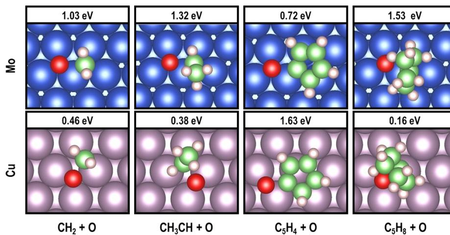
**Figure S5.** Top views of the adsorption sites and adsorption energies for the reactants adsorbed on either a supported- or a doped-Mo SAC. Color code as in Figure S1.
