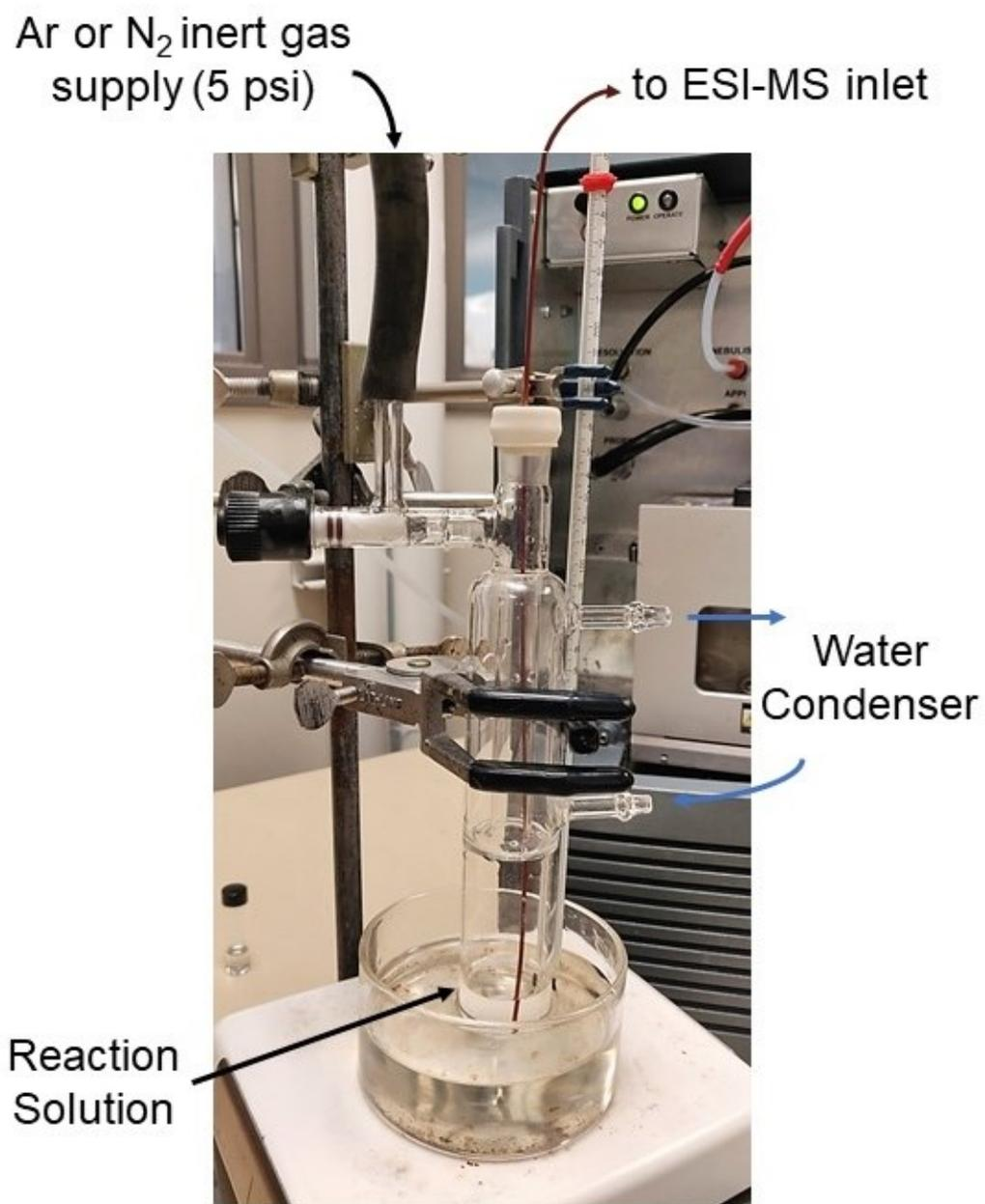
Figure SI 8: Photo of pressure sample infusion ESI-MS set-up
