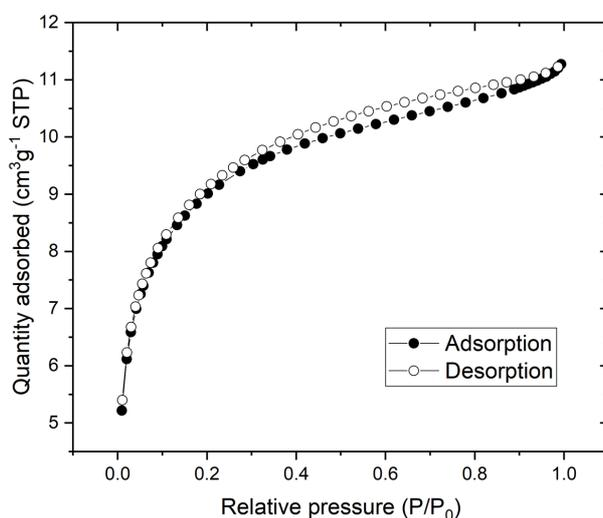
**Figure S12** N<sub>2</sub> adsorption/desorption isotherm for sMAOF(0.01,A)
