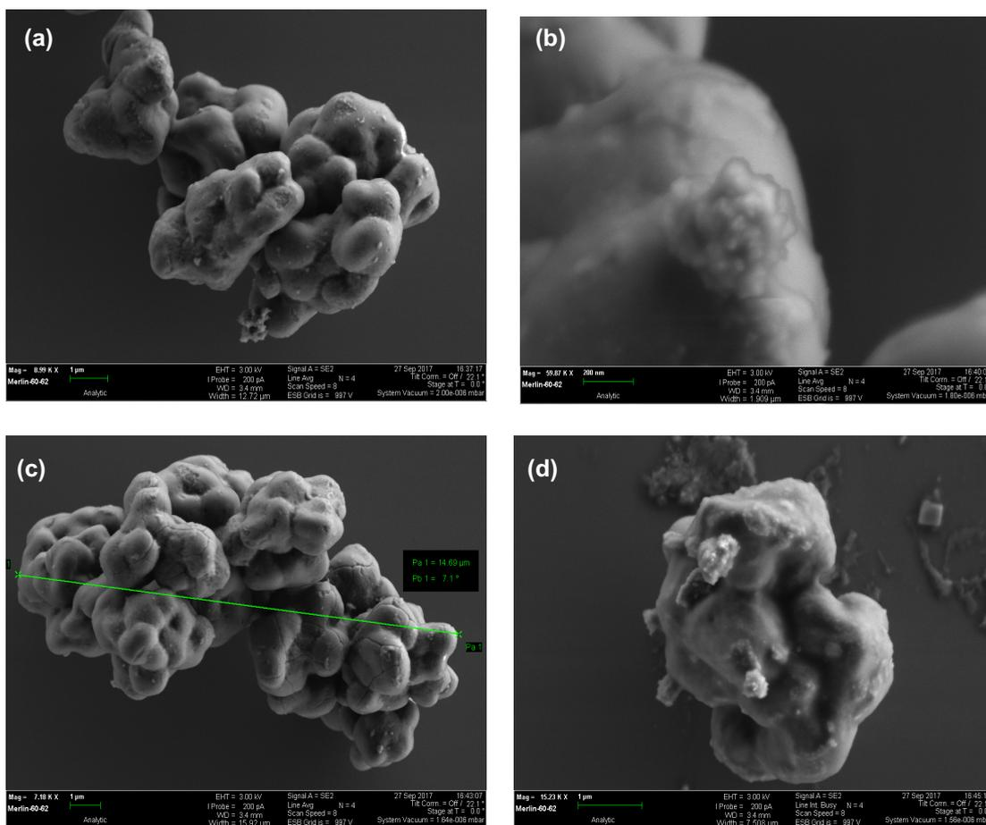
**Figure S20** SEM images of sMAOF(0.025,A) at (a) x8.99k (b) x59.87k (c) 7.18k and (d) x15.23k magnification.
