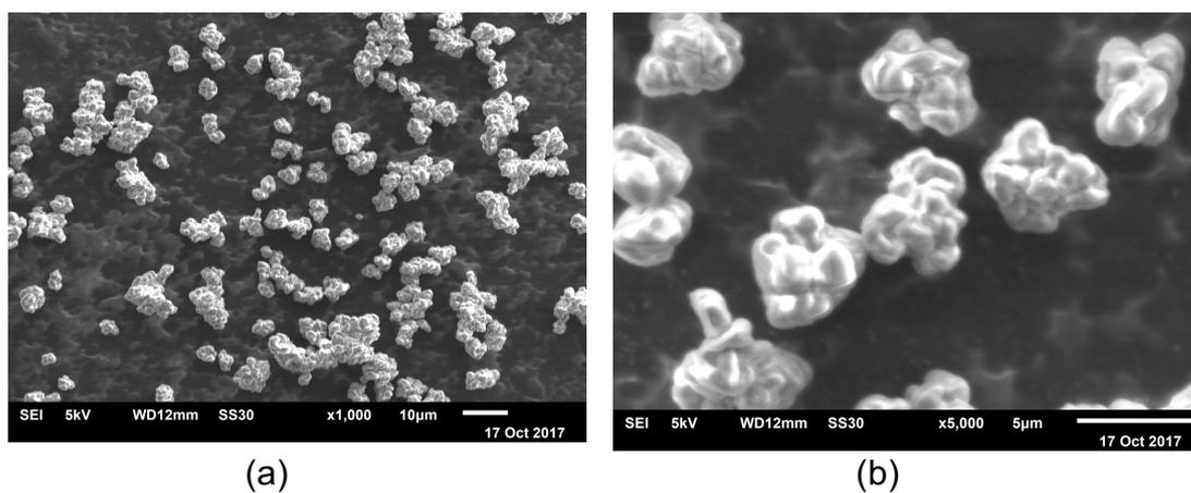
**Figure S19** SEM images of sMAOF(0.025,A) at (a) x1,000 and (b) x5,000 magnification.
