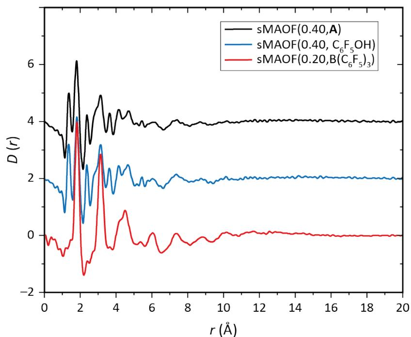
**Figure S15** Overlaid X-ray PDFs of the sMAOF(0.40,A) and previously reported sMAOF(0.40,C<sub>6</sub>F<sub>5</sub>OH), and sMAOF(0.20,B(C<sub>6</sub>F<sub>5</sub>)<sub>3</sub>).
