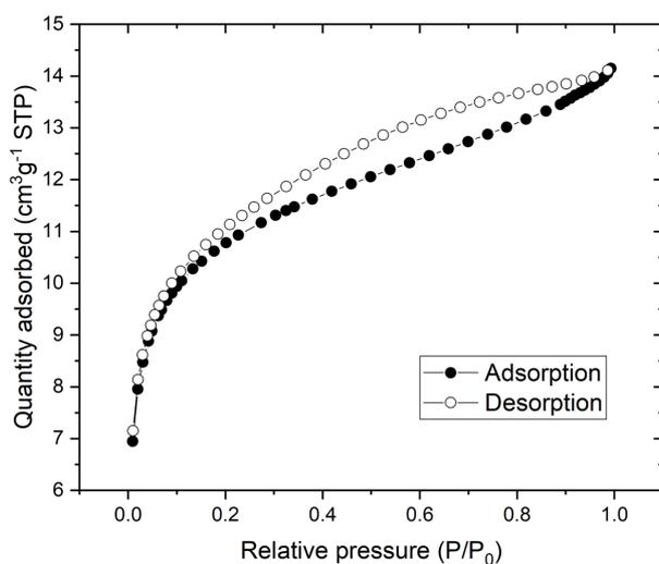
**Figure S14** N<sub>2</sub> adsorption/desorption isotherm for sMAOF(0.05,A)
