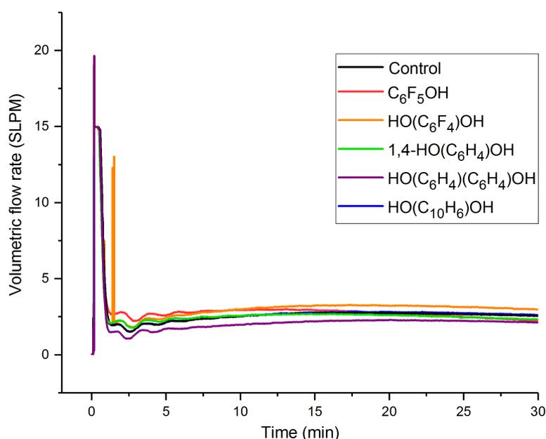
**Figure S23** Ethylene flow in standard litre per minute (SLPM) during scale-up polymerisation for (EBI)ZrCl<sub>2</sub>-sMAOF(0.025,M) catalysts. Polymerisation conditions: 25 mg catalyst, 8 bar C<sub>2</sub>H<sub>4</sub>, 80 °C, AlEt<sub>3</sub> = 2.5 mL, hexanes (1000 mL).
