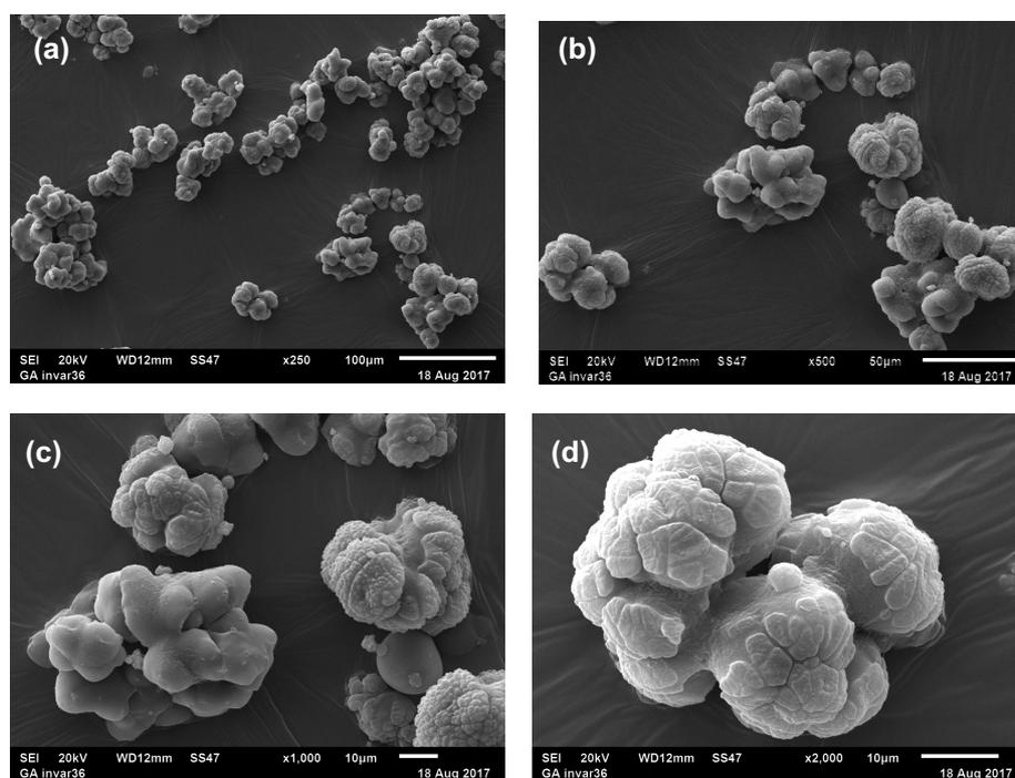
**Figure S25** SEM images at (a)×250, (b)×500, (c)×1000 and (d)×2000 magnification of PE samples produced from a(EBI)ZrCl<sub>2</sub>-sMAOF(0.05,A) catalyst system.
