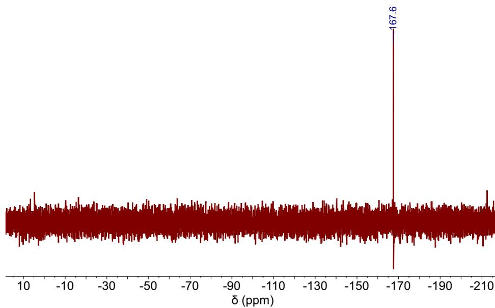
**Figure S3**  $^{19}\text{F}$   $\{^1\text{H}\}$  NMR spectrum of sMAOF(0.025/A) in  $d_8$ -THF.
