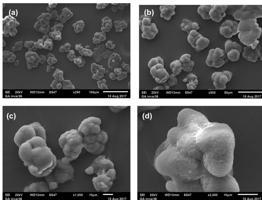
**Figure S24** SEM images at (a)×250, (b)×500, (c)×1000 and (d)×2000 magnification of PE samples produced from a(EBI)ZrCl<sub>2</sub>-sMAOF(0.025,A) catalyst system.
