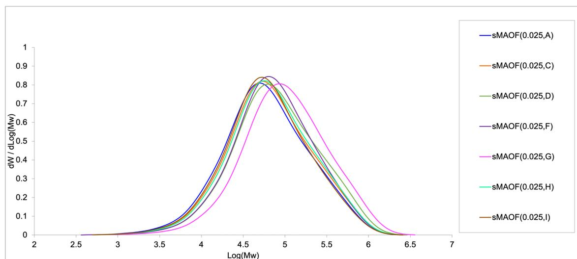
**Figure S27** Overlaid GPC traces of PE samples produced from (EBI)ZrCl<sub>2</sub>-sMAOF(0.025,M) catalysts at target loading  $[Al]_{sMAO} / [Zr]_0 = 200$ .
