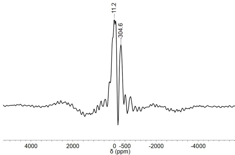
**Figure S6**  $^{27}\text{Al}$  Hahn echo SSNMR spectrum (15 kHz spinning) of sMAOF(0.05/A).
