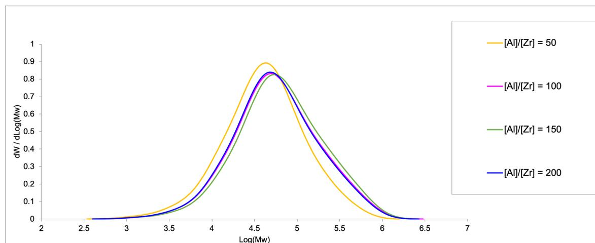
**Figure S26** Overlaid GPC traces of PE samples produced from (EBI)ZrCl<sub>2</sub>-sMAOF(0.025,A) catalysts at different zirconocene complex loadings.
