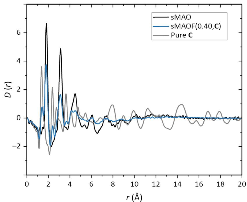
**Figure S16** Overlaid X-ray PDFs of the control sMAO sample, sMAOF(0.40,C) and the pure modifier compound C.
