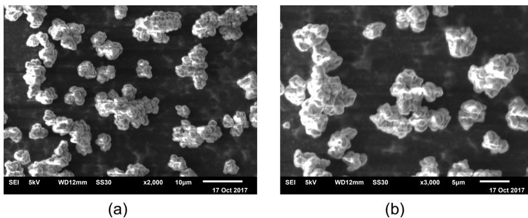
**Figure S21** SEM images of sMAOF(0.025,C) at (a) x2,000 and (b) x3,000 magnification.
