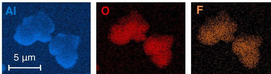
**Figure S18** SEM micrograph of sMAOF(0.40,A) particles with corresponding Al, (blue), O (red), and F (orange) elemental maps, as determined by EDX spectroscopy.
