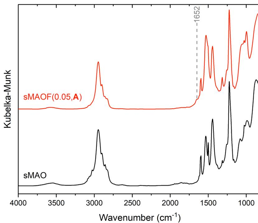
**Figure S1** Overlaid DRIFT spectra (NaCl window) of sMAOF(0.05/A) (red) and sMAO (black), with IR band assigned to the  $\nu(\text{C}=\text{C})$  stretch of the bridging  $-\text{OC}_6\text{F}_4\text{O}-$  group highlighted.
