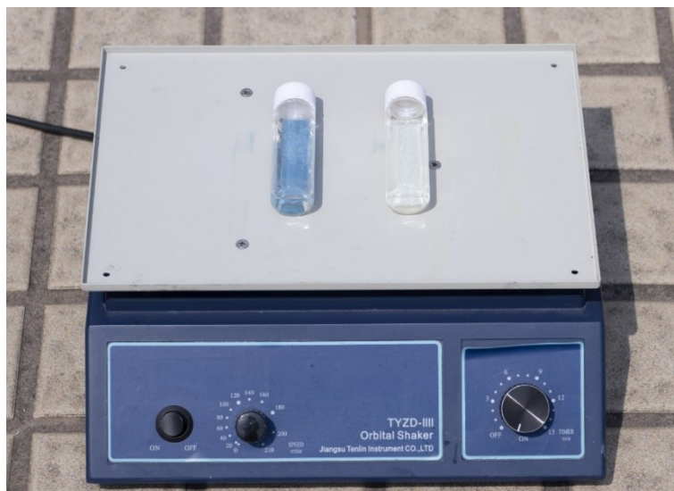
Fig. S6 The CO 2 reduction devices under natural sunlight for catalytic fibers.
