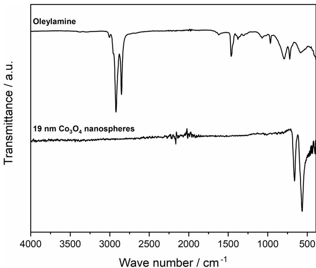
Fig. S2 FTIR spectra of the spherical  $\text{Co}_3\text{O}_4$  nanoparticles with a mean diameter of 19 nm and the surfactant (oleylamine).
