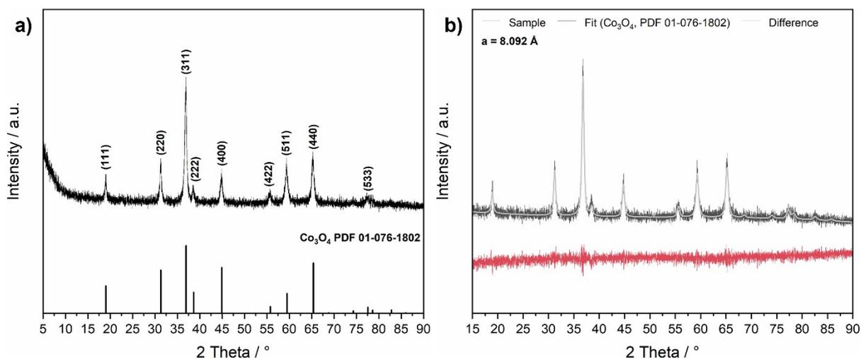
Fig. S1 a) XRD pattern and b) Rietveld refinement of the spherical  $\text{Co}_3\text{O}_4$  nanoparticles with a mean diameter of 19 nm.
