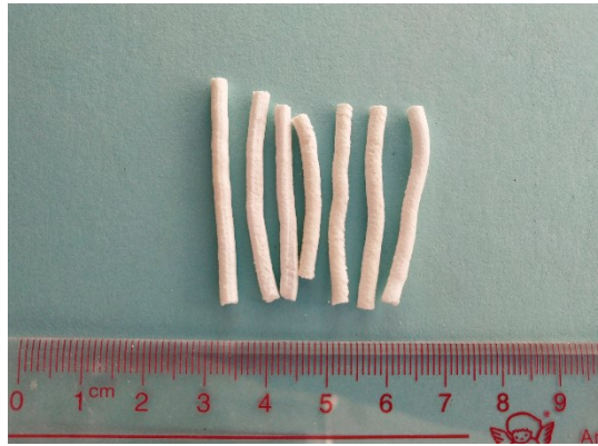
Fig. S1. Photograph of the shaped aluminosilicate extrudate before crystallization.
