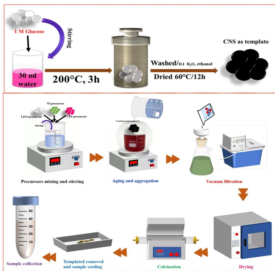
Fig. S1 Comprehensive synthetic scheme of Ni +2 species doped, and TS-1 coupled porous LaFeO 3 nanocomposite by utilizing carbon nanosphere (CNS) as sequential template approach (STA)
