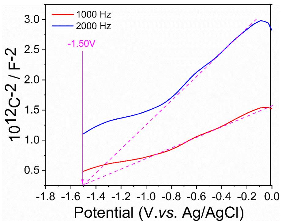
**Fig. S9.** Mott-Schottky plots for CbzCMP-2 in 0.2 M Na<sub>2</sub>SO<sub>4</sub> aqueous solution at 1000 and 2000 Hz
