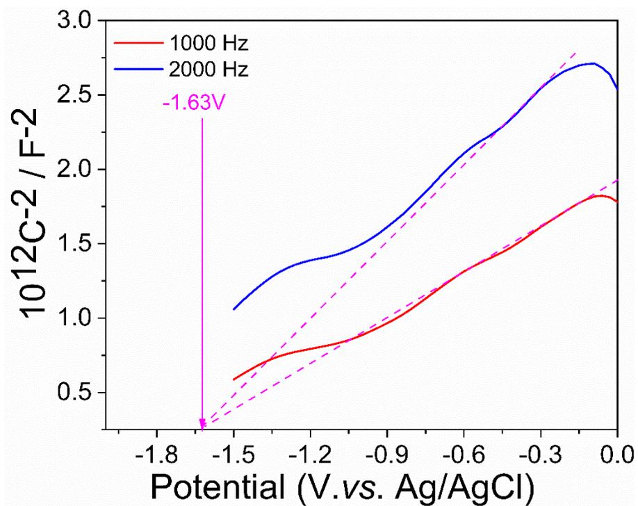
**Fig. S10.** Mott-Schottky plots for CbzCMP-3 in 0.2 M Na<sub>2</sub>SO<sub>4</sub> aqueous solution at 1000 and 2000 Hz
