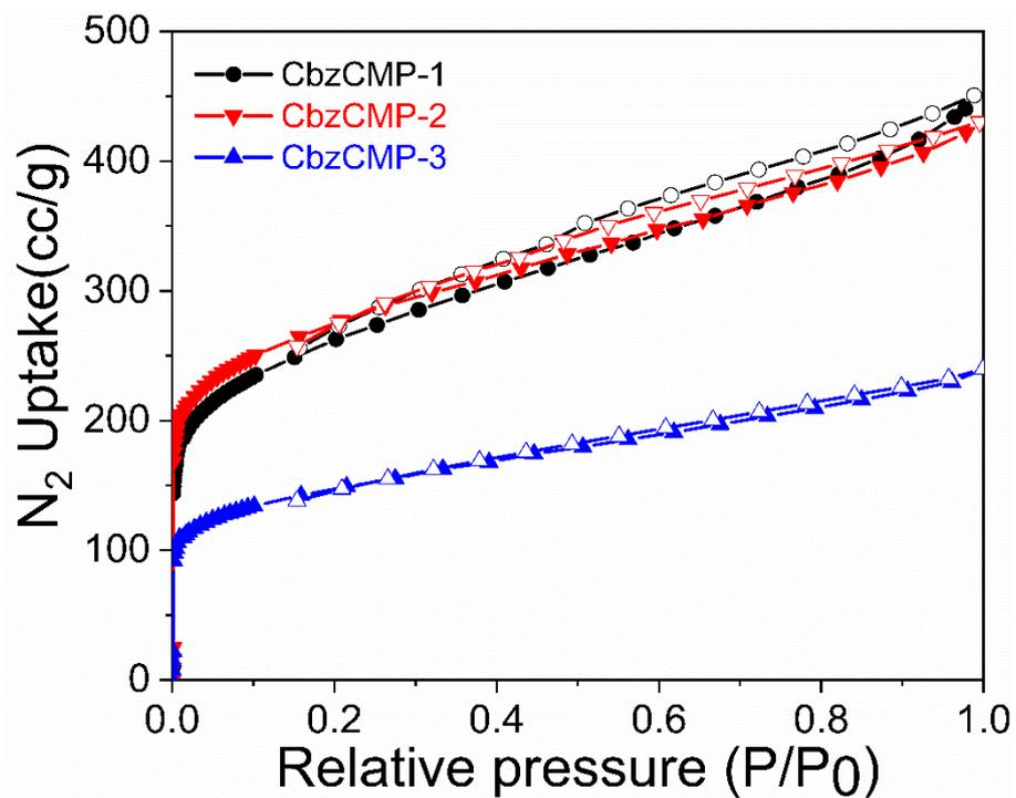
Fig. S6. Nitrogen sorption isotherms of CbzCMP-1, CbzCMP-2 and CbzCMP-3 at 77 K
