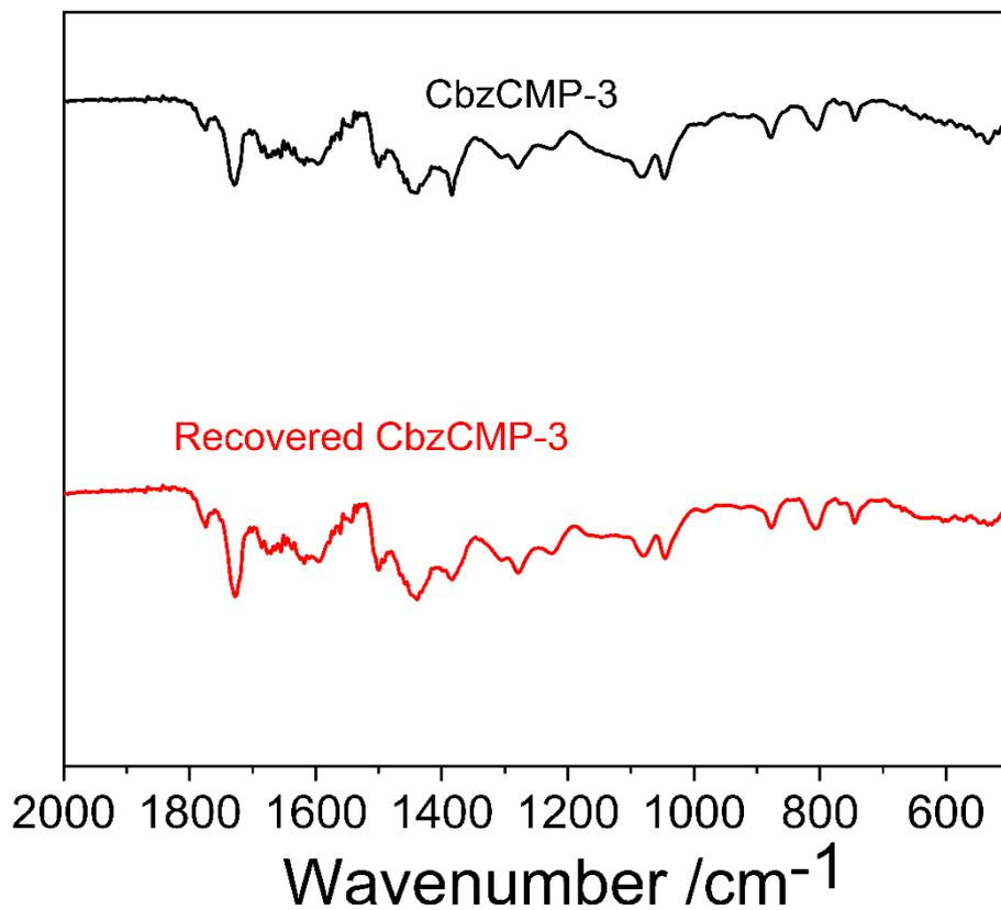
**Fig. S20.** FT-IR spectra of CbzCMP-3 and recovered CbzCMP-3 after ten cycles
