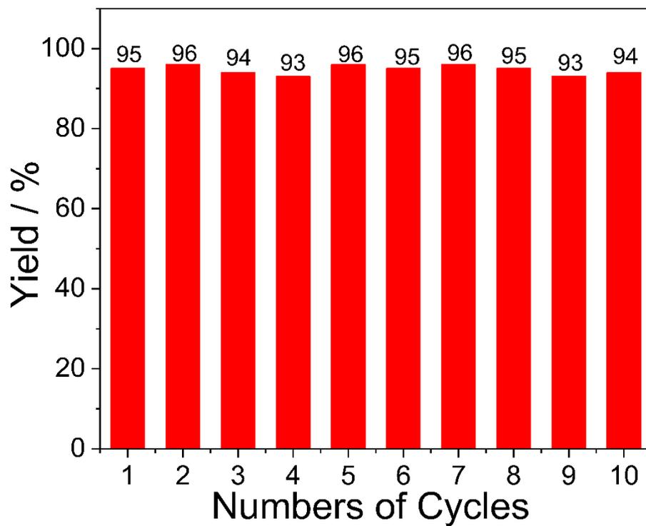
**Fig. S19.** Recyclability tests of CbzCMP-3 in reductive dehalogenation of 2-chloro-1-phenylethan-1-one
