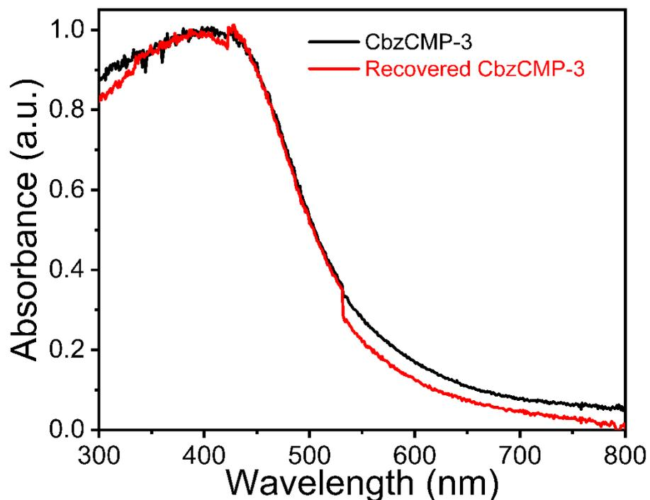
**Fig.S21.** UV/vis DRS spectra of CbzCMP-3 and recovered CbzCMP-3 after ten cycles
