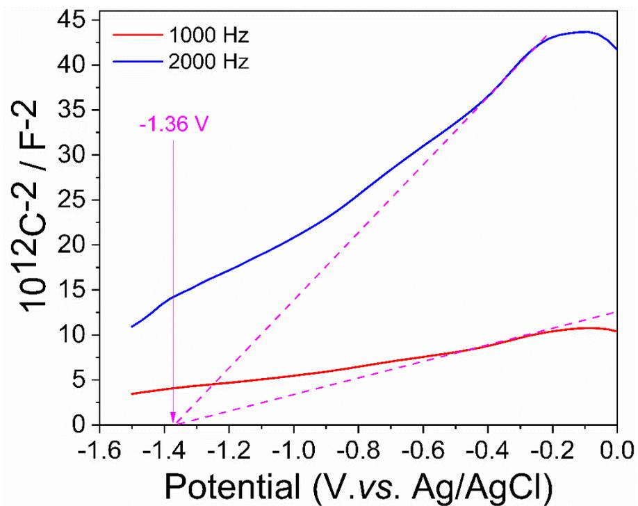
**Fig. S8.** Mott-Schottky plots for CbzCMP-1 in 0.2 M Na<sub>2</sub>SO<sub>4</sub> aqueous solution at 1000 and 2000 Hz
