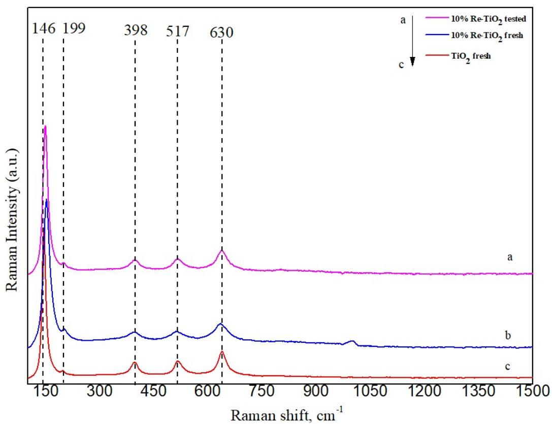
**Fig. S10.** Raman spectra for 10%Re-TiO<sub>2</sub> (tested at 210 °C) (a), 10%Re-TiO<sub>2</sub> (fresh) (b) and 0%Re-TiO<sub>2</sub> (fresh) (c)
