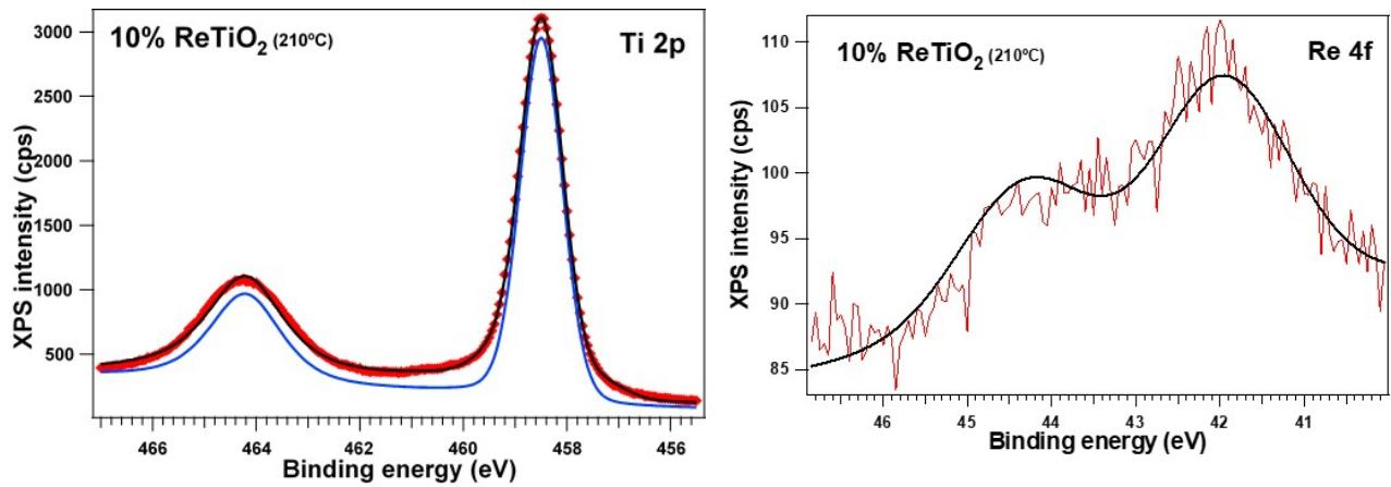
**Fig. S11.** XPS spectra of the Ti (2p) and Re (4f) level for 10%Re-TiO<sub>2</sub> tested at 210 °C
