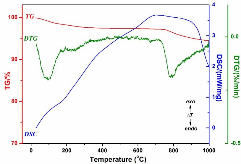
**Fig. S7.** Thermal curves (TG, DTG, and DSC) of the 2%Re- $\text{TiO}_2$  material
