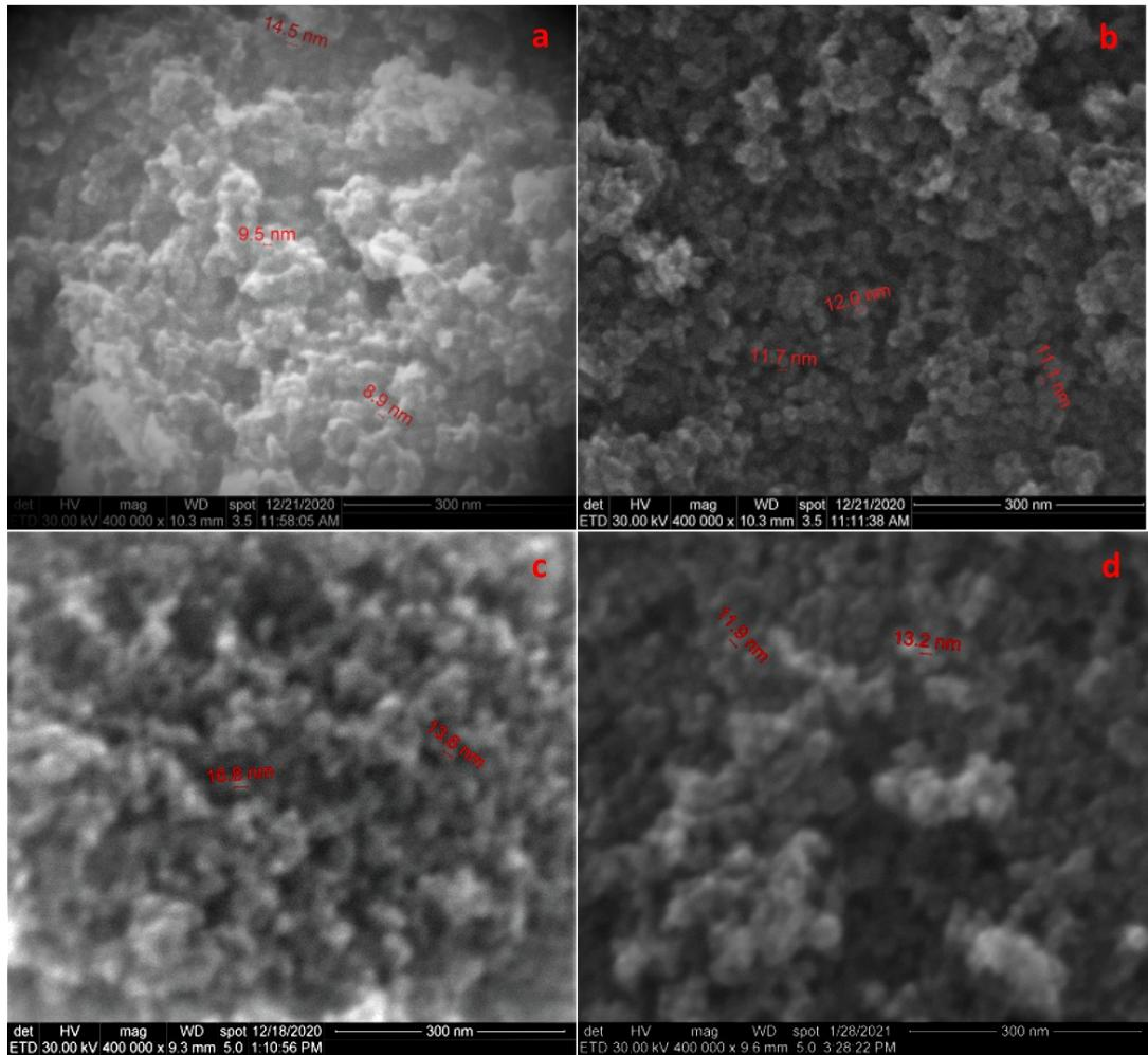
**Fig. S2.** Scanning electron microscopy (SEM) images of a) undoped TiO<sub>2</sub> nanoparticles (fresh), b) 2% Re- doped TiO<sub>2</sub> nanoparticles (fresh) c) 10% Re-doped TiO<sub>2</sub> nanoparticles (fresh) and d) 10% Re-doped TiO<sub>2</sub> nanoparticles (spent).
