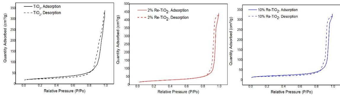
**Fig. S1.** Nitrogen adsorption and desorption isotherms for 0%Re-TiO<sub>2</sub>, 2% Re- TiO<sub>2</sub> and 10% Re-TiO<sub>2</sub>
