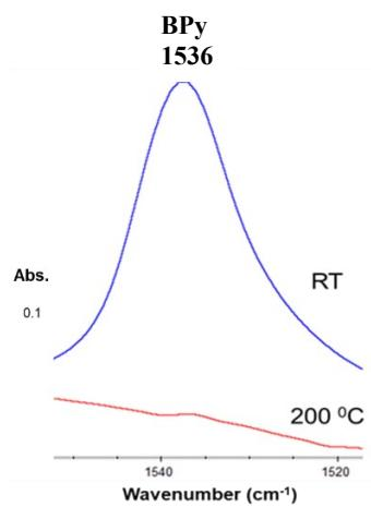
**Fig. S9.** In situ FTIR spectra for 10% Re-TiO<sub>2</sub> catalyst concerning desorption of pyridine at room temperature (RT) and 200 °C
