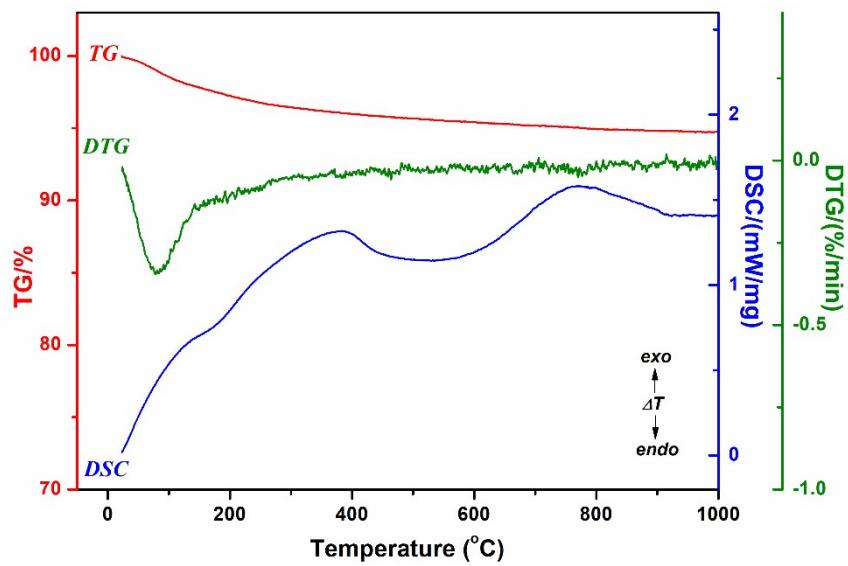
**Fig. S6.** Thermal curves (TG, DTG, and DSC) of undoped  $\text{TiO}_2$
