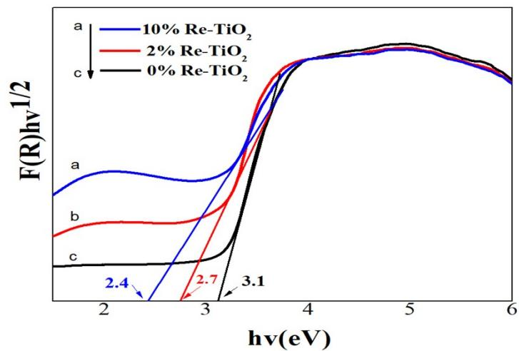
**Fig. S4.** Determination of band gaps for 10% Re-TiO<sub>2</sub> (a), 2%Re-TiO<sub>2</sub> (b) and 0%Re-TiO<sub>2</sub> (c)
