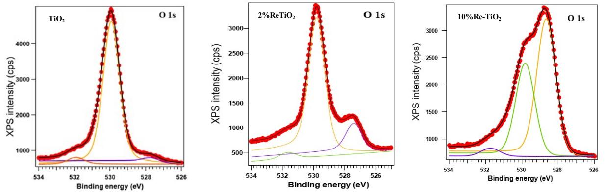
**Fig. S5.** XPS spectra of O1s for: 0%Re-TiO<sub>2</sub>; 2%Re-TiO<sub>2</sub> and 10% Re-TiO<sub>2</sub>
