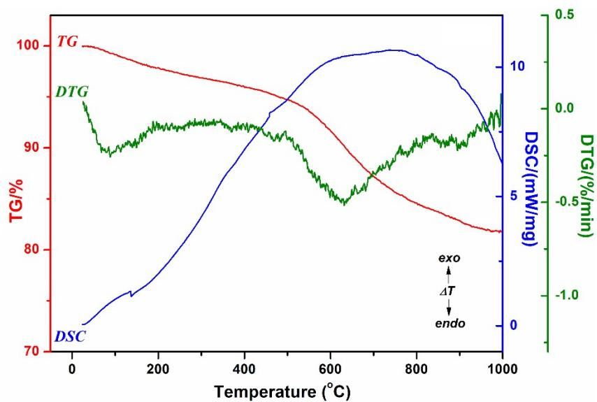
**Fig. S8.** Thermal curves (TG, DTG, and DSC) of the 10%Re-TiO<sub>2</sub> material
