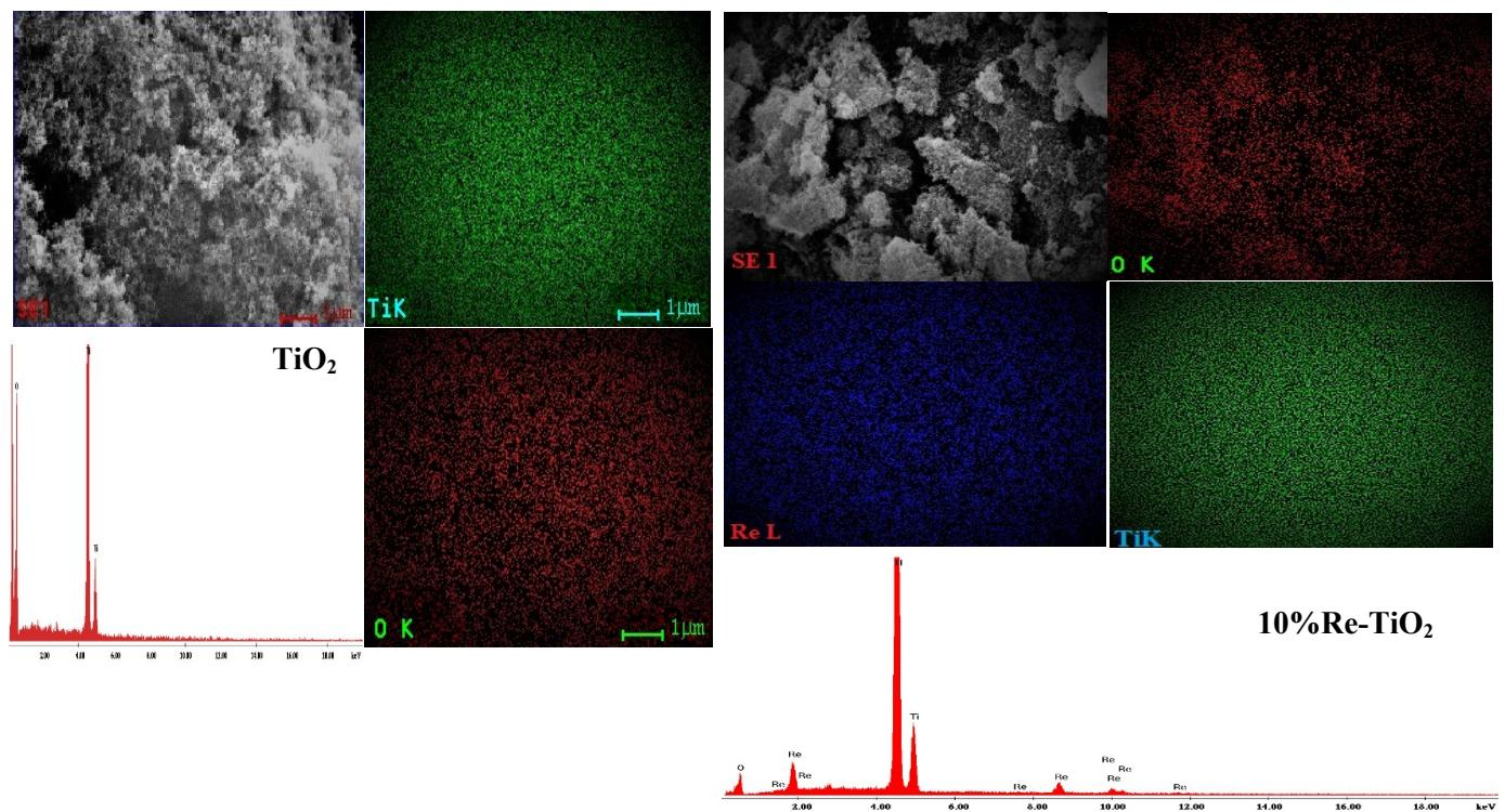
**Fig. S3.** Elemental mapping of Ti, O and Re for  $\text{TiO}_2$  and 10%Re-TiO<sub>2</sub> taken from the area of the SEM shown in the inset of figure (SE1)
