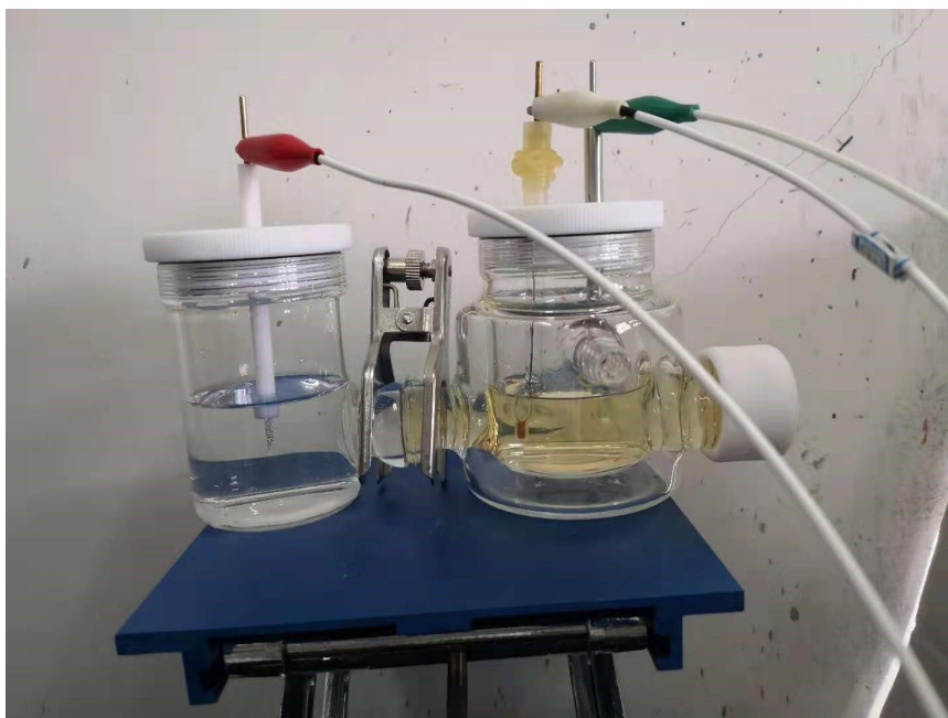
Figure S10. As mentioned in main text, The \text{BiVO}_4 film photoanode was prepared via the electrodeposition method. 0.04 \text{ M Bi(NO}_3)_3 was dissolved in 50 \text{ ml } 0.4 \text{ M KI} solution which pH was adjusted to 1.7 by \text{HNO}_3 . At the same time, 0.23 \text{ M p-benzoquinone} was added to 20 \text{ ml ethyl alcohol} . Then, these two kinds of solution were poured together and mixed under rapid stirring until the solution became clear. The Bi species layer was deposited in the above solution by applying a repetitive sequence of passing 0.1 \text{ C/cm}^2 at a potential of -0.1 \text{ V} versus \text{Ag/AgCl} . Then, 200 \mu\text{l } 0.2\text{M VO(acac)}_2 in \text{DMSO} was placed on \text{BiOI} and calcination at 450^\circ\text{C} for 2 \text{ h} .
