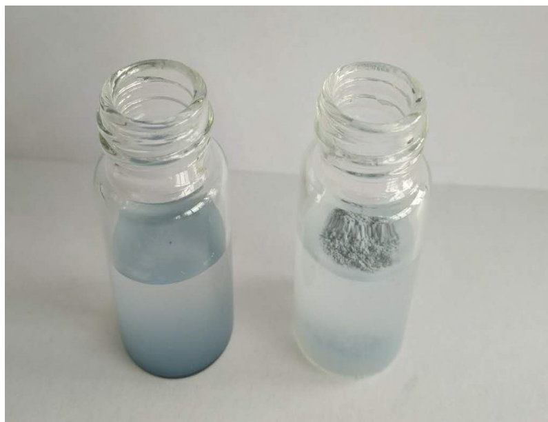
Fig. S4 The optical diagram of \text{TiO}_2\text{-SBO} and \text{F-TiO}_2\text{-SBO-3} samples dispersed in water.
