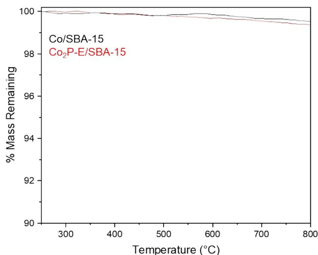
Figure S1. TGA of Co/SBA-15 (black) and Co<sub>2</sub>P-E/SBA-15 (red) after EDH. Reaction conditions 600°C, 5% C<sub>2</sub>H<sub>6</sub>, 5% H<sub>2</sub>, balance He, 100 ml/min total flow.
