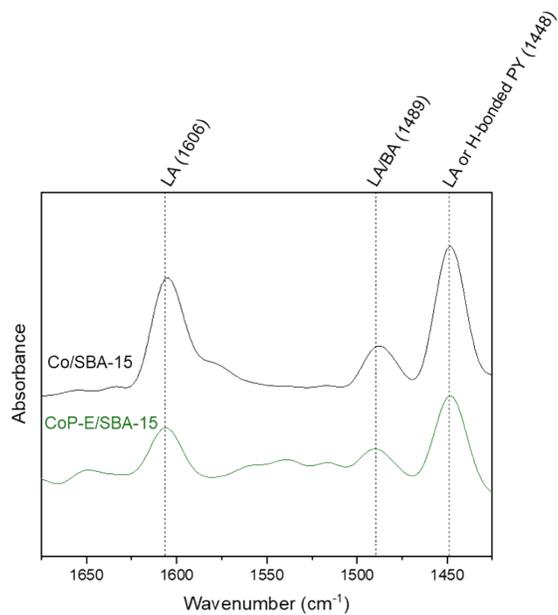
Figure S6. Pyridine DRIFTS of Co/SBA-15 and CoP-E/SBA-15 after purging at 150°C. (LA – Lewis acid feature, BA – Brønsted acid feature)
