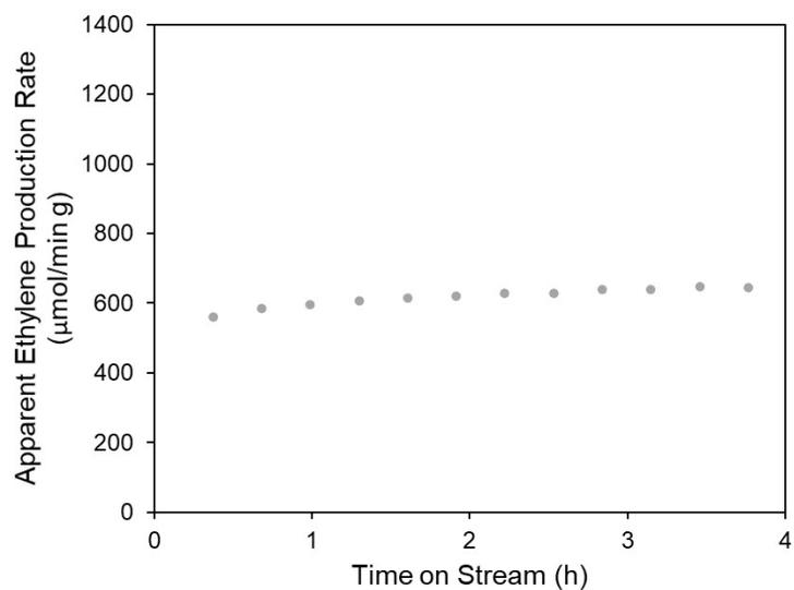
Figure S8. High temperature background runs with SBA-15 (grey). Reaction conditions were 700°C 5% C<sub>2</sub>H<sub>6</sub>, 5% H<sub>2</sub>, balance He, 100 ml/min total flow, 5 mg catalyst.
