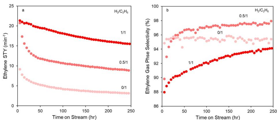
Figure S2. Ethylene STY (a) and ethylene carbon gas phase selectivity (b) as a function of time for varying H<sub>2</sub>:C<sub>2</sub>H<sub>6</sub> ratio.
