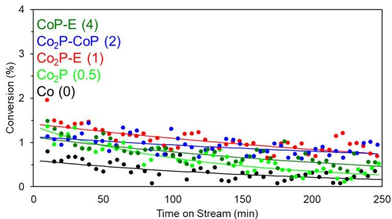
Figure S4. Conversion as a function of time for low temperature dehydrogenation reactions. The lines are the fit of the conversion vs time data to Equation 4. The value in parentheses is the nominal P:Co ratio. Reaction conditions were 600°C, 5% C<sub>2</sub>H<sub>6</sub>, 5% H<sub>2</sub>, balance He, 100 ml/min total flow.
