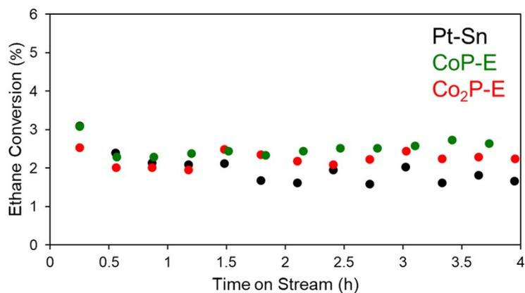
Figure S9. Conversion as a function of time for high temperature dehydrogenation reactions. Reaction conditions were 700°C, 5% C<sub>2</sub>H<sub>6</sub>, 5% H<sub>2</sub>, balance He, 100 ml/min total flow, 5 mg catalyst.
