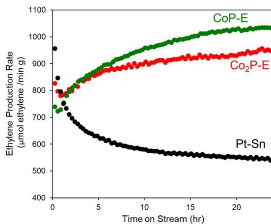
Figure S11. Ethylene production over time with CoP/SBA-15 (green), Co<sub>2</sub>P/SBA-15 (red), Pt-Sn/SBA-15 (black). Reaction conditions were 700°C, 5% C<sub>2</sub>H<sub>6</sub>, 5% H<sub>2</sub>, balance He, 100 ml/min, 5 mg catalyst.
