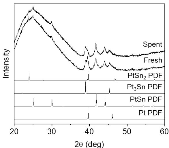
Figure S10. XRD of Pt-Sn/SBA-15 before and after reaction.
