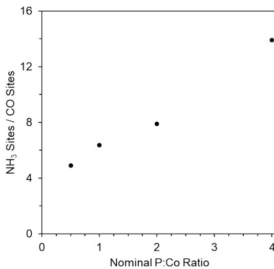
Figure S7. NH<sub>3</sub> sites (from NH<sub>3</sub> TPD) / CO Sites (from CO pulse) as a function of P:Co ratio.
