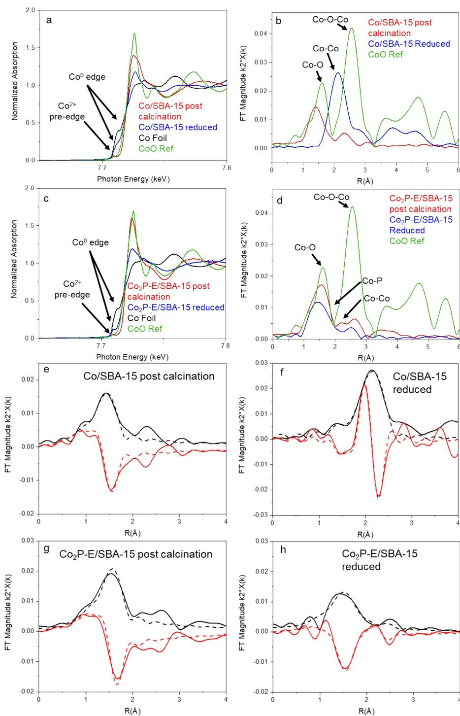
Figure S3. XANES and EXAFS spectra for Co/SBA-15 (a-b) and Co<sub>2</sub>P-E/SBA-15 (c-d). The X axis in b and d are uncorrected bond distances. The fits are provided for each sample: Co/SBA-15 post calcination (e) and reduced (f), Co<sub>2</sub>P-E/SBA-15 post calcination (g) and reduced (h). The black and red lines indicate the magnitude and imaginary components of the Fourier transform respectively where the solid lines represent the data and dashed lines represent the fit.
