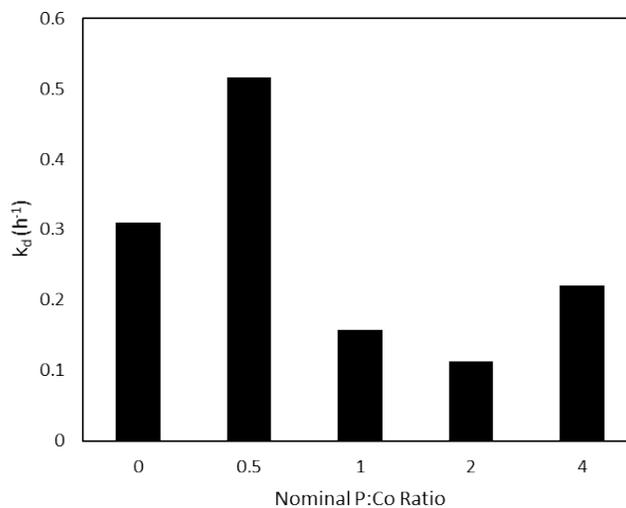
Figure S5.  $k_d$  values for different P:Co ratio materials during EDH. Reaction conditions were 600°C, 5% C<sub>2</sub>H<sub>6</sub>, 5% H<sub>2</sub>.
