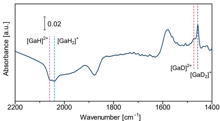
**Figure S3.** IR spectra for exchange reaction of Ga hydrides with D<sub>2</sub> at 300 °C. After the RSSIE reaction for Ga-MFI-1.0(800) (H<sub>2</sub>, 800 °C), the temperature decreased to 50 °C to take the background spectrum. Next, the sample was exposed to D<sub>2</sub> at 300 °C and then the temperature decreased to 50 °C again for measurement.
