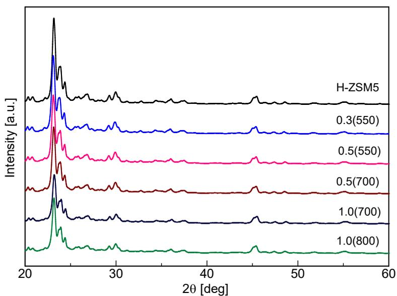
**Figure S4.** XRD patterns of a series of Ga-MFI after RSSIE. The XRD measurements were performed under room temperature and air atmosphere.
