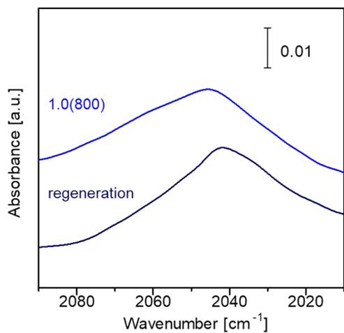
**Figure S2.** IR spectra of regenerated Ga-hydrides by H<sub>2</sub> treatment of the He-treated Ga-MFI-1.0(800). The difference spectrum was obtained in a similar manner.
