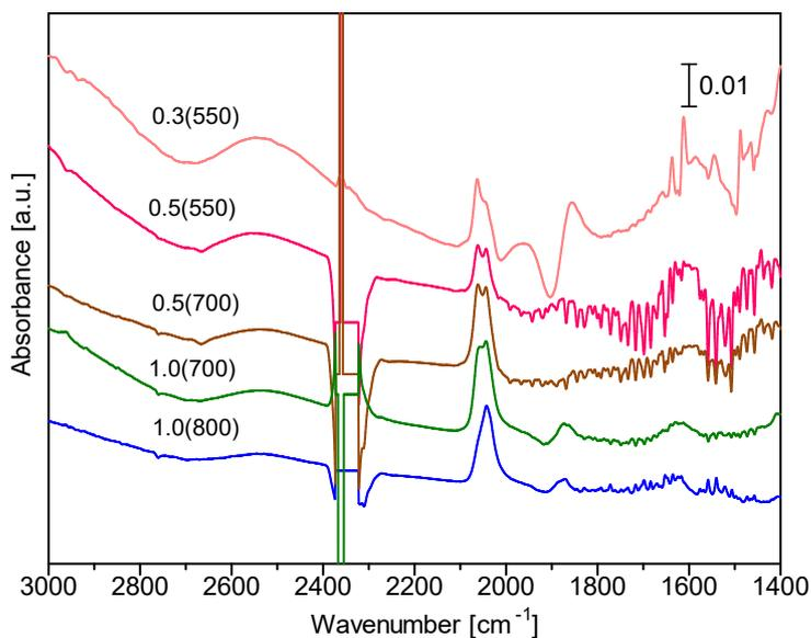
**Figure S1.** Wide-range difference IR spectra obtained at 50 °C without exposure to air. The IR spectra after H<sub>2</sub> treatment at different temperature was recorded at 50 °C and then the sample was further treated at 800 °C under He flow followed by cooling to 50 °C to record the spectra. The difference IR spectra were obtained by subtracting the spectra after He treatment from the ones after H<sub>2</sub> treatment.
