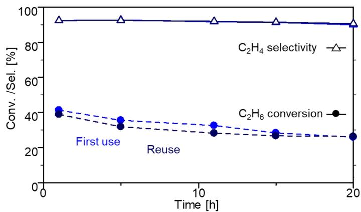
**Figure S5.** Time on stream of reuse experiment. Reaction conditions: 100 mg of Ga-MFI-1.0(800), 10% C<sub>2</sub>H<sub>6</sub>/He (10 mL/min), 660 °C. Regeneration treatment: (1) 5% O<sub>2</sub>/He (10 mL/min), 600 °C. (2) 10% H<sub>2</sub>/He (10 mL/min), 800 °C.
