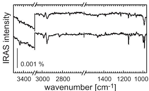
**Figure S1** IRAS measurements of 0.1 L (top) and 0.3 L (bottom)  $^{13}\text{C}$ -methanol (99 atom %  $^{13}\text{C}$ , Sigma Aldrich) adsorbed on clean Au(332) at 120 K.
