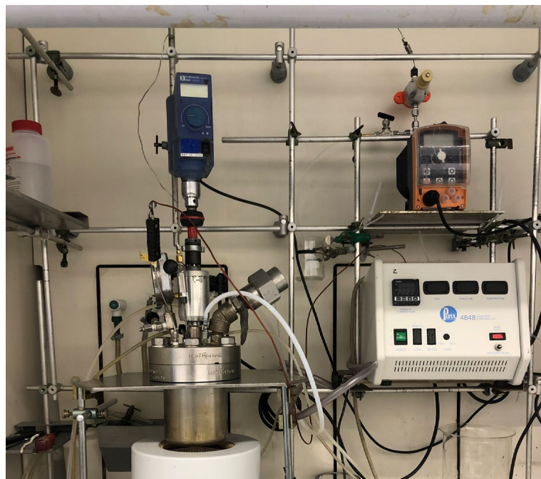
Figure S12. Reaction set-up for hydrolysis of polyester experiments.
