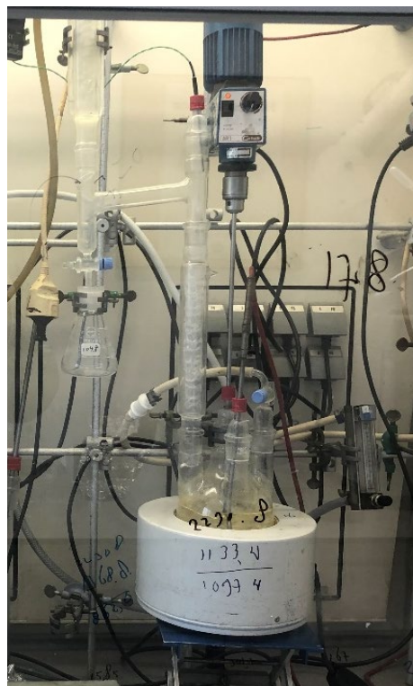
Figure S1. (A) Reaction set-up for neat polyesterification. (B) Reaction set-up for azeotropic polyesterification and in-situ FTIR-ATR.
