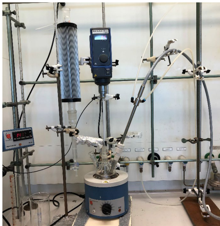
Figure S1. (A) Reaction set-up for neat polyesterification. (B) Reaction set-up for azeotropic polyesterification and in-situ FTIR-ATR.
