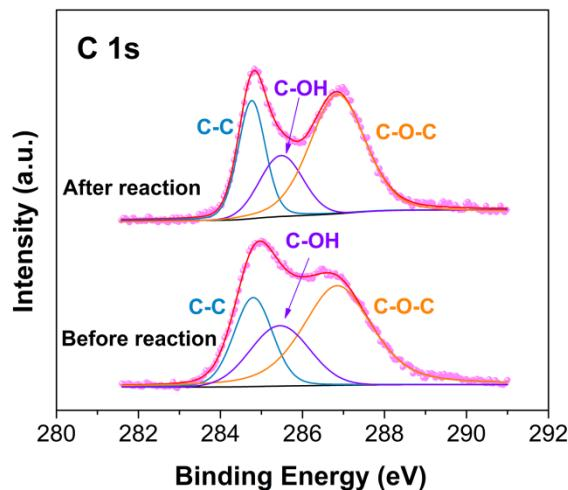
**Fig. S12.** C 1s signals of 2%-RGO/C<sub>0.15</sub>ZIS before and after photocatalytic reaction.
