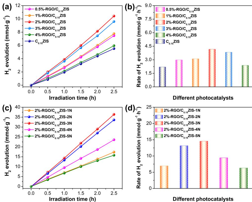
**Fig. S6.** (a, c) Photocatalytic H<sub>2</sub> generation activities and (b, d) corresponding HER rates of (a, b) x-RGO/C<sub>0.15</sub>ZIS ( $x = 0, 0.5\%, 1\%, 2\%, 3\%$ , and  $4\%$ ) and (c, d) 2%-RGO/C<sub>0.15</sub>ZIS-yN ( $y = 1, 2, 3, 4$ , and  $5$ ).
