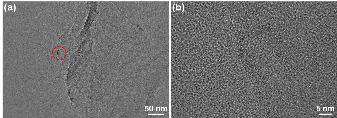
**Fig. S2.** (a) TEM and (b) HRTEM images of RGO nanosheets. (b) is magnified from the area (red dotted circle) marked in (a).
