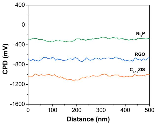
**Fig. S14.** Contact potential differences of  $\text{Ni}_2\text{P}$ , RGO, and  $\text{C}_{0.15}\text{ZIS}$  relative to the probe.
