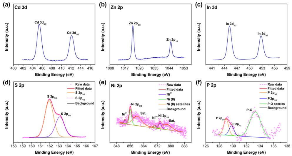
**Fig. S10.** (a) Cd 3d, (b) Zn 2p, (c) In 3d, (d) S 2p, (e) Ni 2p, and (f) P 2p spectra of 2%-RGO/C<sub>0.15</sub>ZIS-5N after photocatalytic reaction.
