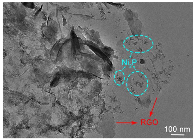
**Fig. S3.** TEM observation on the edge area of 2%-RGO/C<sub>0.15</sub>ZIS-3N composite.
