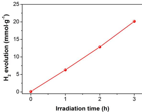
**Fig. S7.** H<sub>2</sub> evolution curve for calculating the AQY of 2%-RGO/C<sub>0.15</sub>ZIS-3N.
