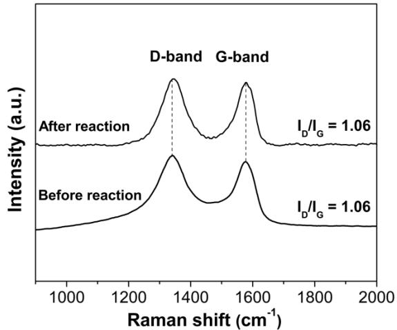
**Fig. S11.** Raman spectra of 2%-RGO/C<sub>0.15</sub>ZIS before and after photocatalytic reaction.
