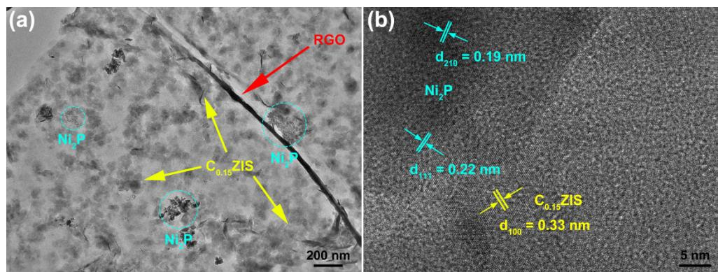
**Fig. S9.** (a) TEM and (b) HRTEM graphs of the 2%-RGO/C<sub>0.15</sub>ZIS-3N composite after HER measurement.
