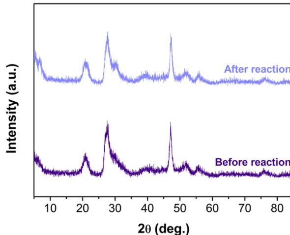
**Fig. S8.** XRD patterns of the 2%-RGO/C<sub>0.15</sub>ZIS-3N hybrid before and after HER test.
