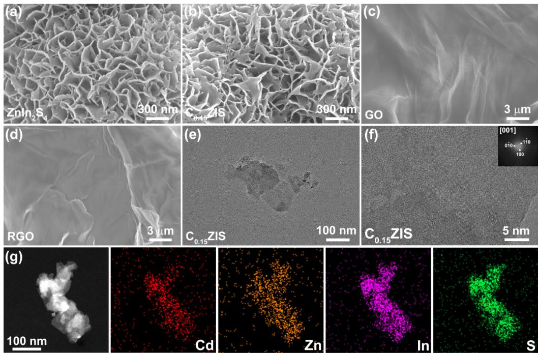
**Fig. S1.** (a-d) SEM images of (a) ZnIn<sub>2</sub>S<sub>4</sub> nanosheets, (b) C<sub>0.15</sub>ZIS nanosheets, (c) GO nanosheets, and (d) RGO nanosheets. (e) TEM, (f) HRTEM, and (g) STEM and EDX mapping results of C<sub>0.15</sub>ZIS nanosheets.
