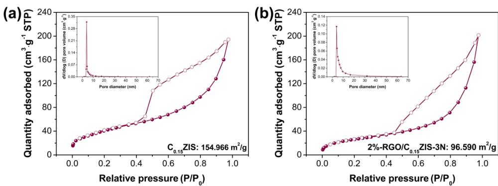
**Fig. S15.**  $\text{N}_2$  adsorption-desorption isotherms and corresponding pore-size distributions of (a)  $\text{C}_{0.15}\text{ZIS}$  and (b) 2%-RGO/ $\text{C}_{0.15}\text{ZIS}$ -3N.
