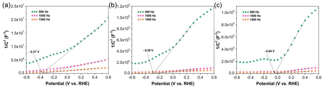
**Fig. S13.** Mott-Schottky curves of (a)  $\text{C}_{0.15}\text{ZIS}$ , (b) 2%-RGO/ $\text{C}_{0.15}\text{ZIS}$ , and (c) 2%-RGO/ $\text{C}_{0.15}\text{ZIS}$ -3N.
