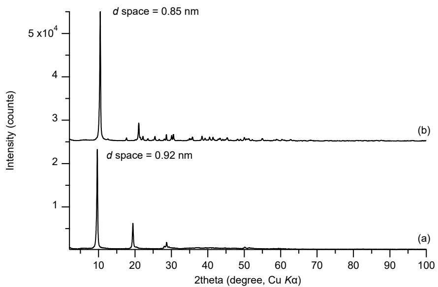
**Fig. S6** XRD profiles for (a)  $\text{NO}_3^-/\text{Y-LRH}$  and (b)  $\text{Cl}^-/\text{Y-LRH}$  catalyst
