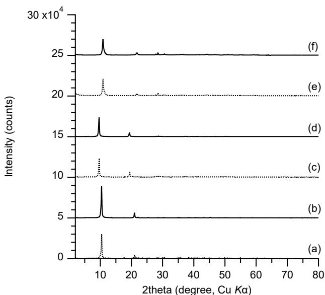
**Fig. S12** XRD profiles for (a) dry  $\text{Cl}^-/\text{Y-LRH}$ , (b) wet  $\text{Cl}^-/\text{Y-LRH}$ , (c) dry  $\text{NO}_3^-/\text{Y-LRH}$ , (d) wet  $\text{NO}_3^-/\text{Y-LRH}$ , (e) dry  $\text{HCOO}^-/\text{Y-LRH}$ , and (f) wet  $\text{HCOO}^-/\text{Y-LRH}$ ,
