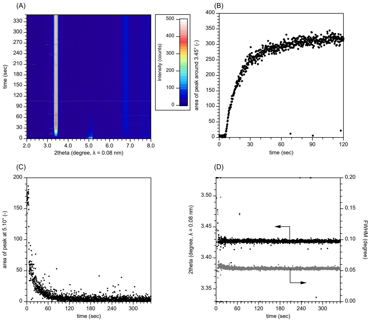
**Fig. S5** (A) 2D mapping plots of the *t*-SXRD patterns of Y-LRH during anion-exchange reaction from  $\text{NO}_3^-$  into  $\text{CH}_3\text{COO}^-$ . (B) Time profile of the newly appeared peak area at  $3.43^\circ$  in *t*-SXRD. (C) Time profile of the disappeared peak area at  $5.10^\circ$  in *t*-SXRD. (D) The peak position and FWHM values of newly appeared peak at  $3.43^\circ$ .
