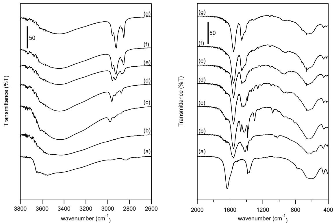
**Fig. S2** FT-IR spectra for (a)  $\text{HCOO}^-/\text{Y-LRH}$ , (b)  $\text{CH}_3\text{COO}^-/\text{Y-LRH}$ , (c)  $\text{C}_2\text{H}_5\text{COO}^-/\text{Y-LRH}$ , (d)  $\text{C}_3\text{H}_7\text{COO}^-/\text{Y-LRH}$ , (e)  $\text{C}_5\text{H}_{11}\text{COO}^-/\text{Y-LRH}$ , (f)  $\text{C}_7\text{H}_{15}\text{COO}^-/\text{Y-LRH}$ , and (g)  $\text{C}_9\text{H}_{19}\text{COO}^-/\text{Y-LRH}$  catalyst.
