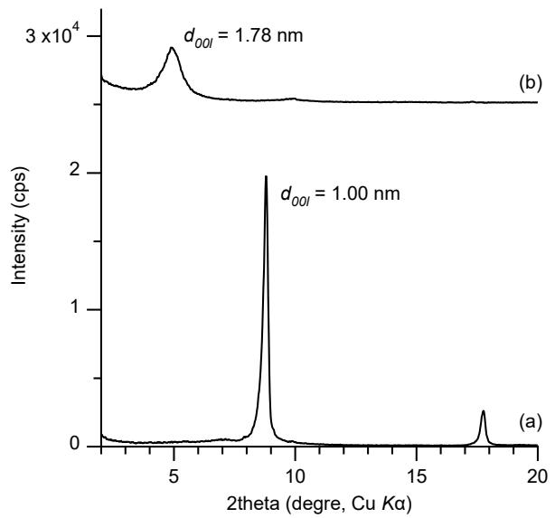
**Fig. S9** XRD profiles for (a) fresh  $\text{CH}_3\text{COO}^-/\text{Y-LRH}$  in dry state and (b) recovered  $\text{CH}_3\text{COO}^-/\text{Y-LRH}$  in dry state. Values in graph were  $d_{00l}$  space, calculated by the Bragg equation
