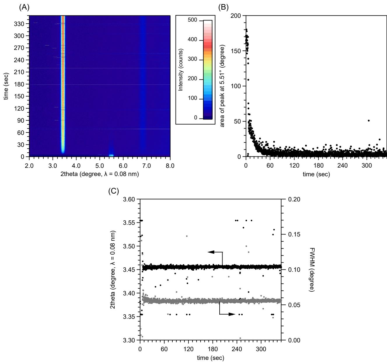
**Fig. S3** (A) 2D mapping plots of the *t*-SXRD patterns of Y-LRH during anion-exchange reaction from  $\text{Cl}^-$  into  $\text{CH}_3\text{COO}^-$ . (B) Time profile of the disappeared peak area at  $5.51^\circ$  in *t*-SXRD. (C) The peak position and FWHM values of newly appeared peak at  $3.45^\circ$ .
