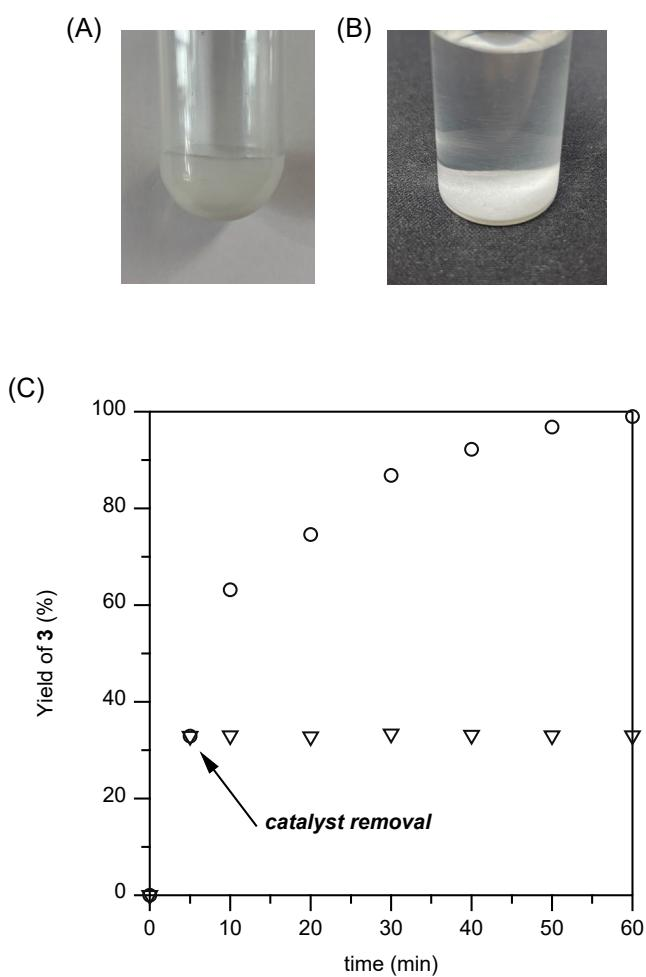
**Fig. S8** (A) Photoimages of  $\text{CH}_3\text{COO}^-/\text{Y-LRH}$  catalyst: (A) during reaction and (B) after centrifugation. (C) Hot filtration experiment. reaction conditions were as follows:  $\text{CH}_3\text{COO}^-/\text{Y-LRH}$  catalyst (0.05 g), **1** (1.5 mmol), **2** (1 mmol),  $\text{H}_2\text{O}$  (5 mL), 303 K. Yield was based on **2**, determined by GC.
