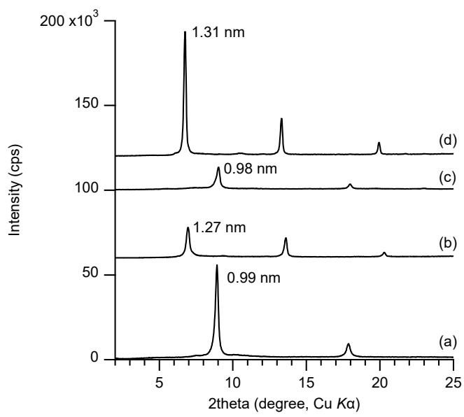
**Fig. S10** XRD profiles for (a) dry  $\text{CH}_3\text{COO}^-/\text{Gd-LRH}$ , (b) wet  $\text{CH}_3\text{COO}^-/\text{Gd-LRH}$ , (c) dry  $\text{CH}_3\text{COO}^-/\text{Yb-LRH}$ , and (d) wet  $\text{CH}_3\text{COO}^-/\text{Yb-LRH}$ . Values in graph were  $d_{00l}$  space, calculated by the Bragg equation.
