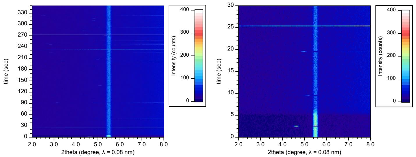
**Fig. S4** 2D mapping plots of the *t*-SXRD patterns of  $\text{Cl}^-/\text{Y-LRH}$ . After 5 sec, 2 mL of water was added in the slurry of  $\text{Cl}^-/\text{Y-LRH}$  (0.05 g) and water (0.5 mL).
