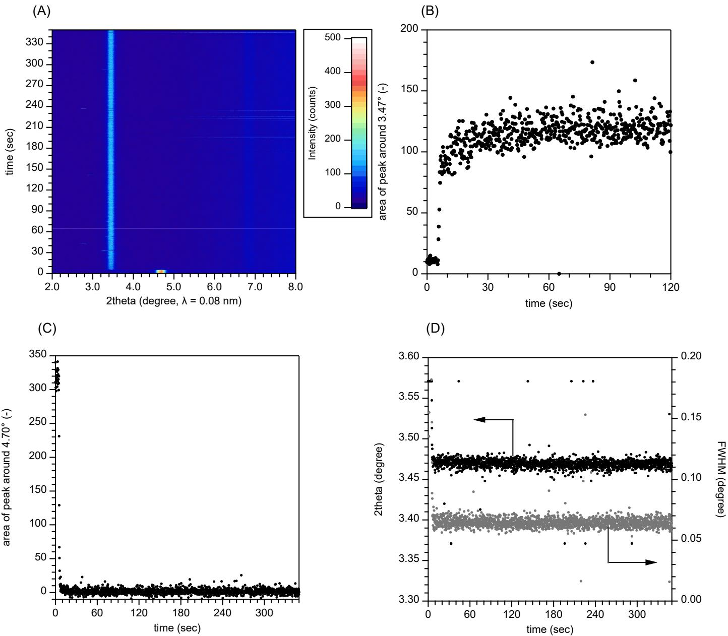
**Fig. S11** (A) 2D mapping plots of the *t*-SXRD patterns of  $\text{CH}_3\text{COO}^-/\text{Y-LRH}$  during the interlayer lift-up process. Arrows indicated the start point of addition of water into solid dispersion in acetonitrile solution. (B) Time profile of the newly appeared peak area at  $3.47^\circ$  in *t*-SXRD. (C) Time profile of the disappeared peak area at  $4.70^\circ$  in *t*-SXRD. (D) The peak position and FWHM values of newly appeared peak at  $3.47^\circ$ .
