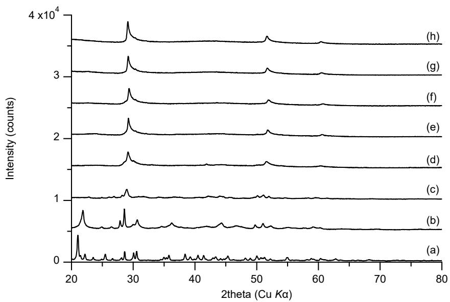
**Fig. S7** XRD profiles for (a)  $\text{Cl}^-/\text{Y-LRH}$ , (b)  $\text{HCOO}^-/\text{Y-LRH}$ , (c)  $\text{CH}_3\text{COO}^-/\text{Y-LRH}$ , (d)  $\text{C}_2\text{H}_5\text{COO}^-/\text{Y-LRH}$ , (e)  $\text{C}_3\text{H}_7\text{COO}^-/\text{Y-LRH}$ , (f)  $\text{C}_5\text{H}_{11}\text{COO}^-/\text{Y-LRH}$ , (g)  $\text{C}_7\text{H}_{15}\text{COO}^-/\text{Y-LRH}$ , and (h)  $\text{C}_9\text{H}_{19}\text{COO}^-/\text{Y-LRH}$  catalyst.
