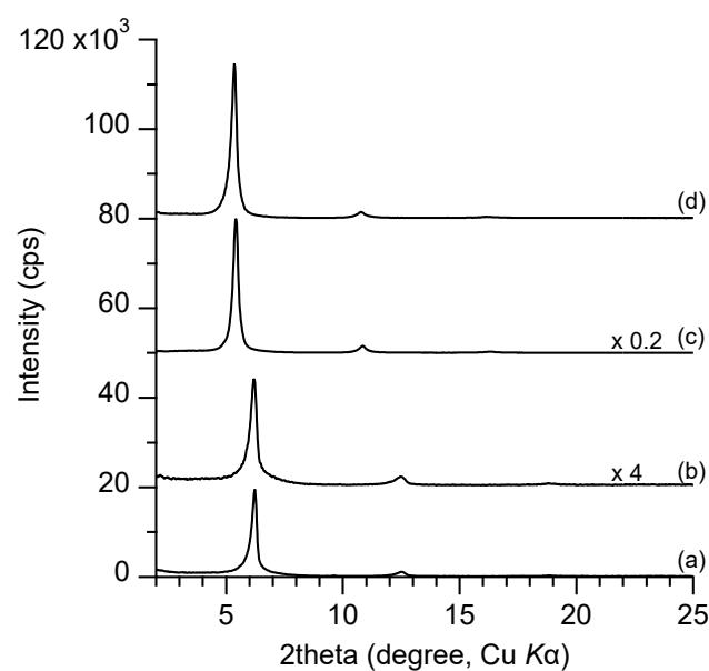
**Fig. S13** XRD profiles for (a) dry  $\text{C}_2\text{H}_5\text{COO}^-/\text{Y-LRH}$ , (b) wet  $\text{C}_2\text{H}_5\text{COO}^-/\text{Y-LRH}$ , (c) dry  $\text{C}_3\text{H}_7\text{COO}^-/\text{Y-LRH}$  and (d) wet  $\text{C}_3\text{H}_7\text{COO}^-/\text{Y-LRH}$  catalyst
