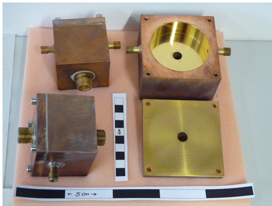
Figure S5: A photo of MCPT cavities of various sizes, made from copper, plated with silver and gold. The disassembled cavity on the right ( h_c = 20 mm, r_c = 34 mm) has been used throughout this work.
