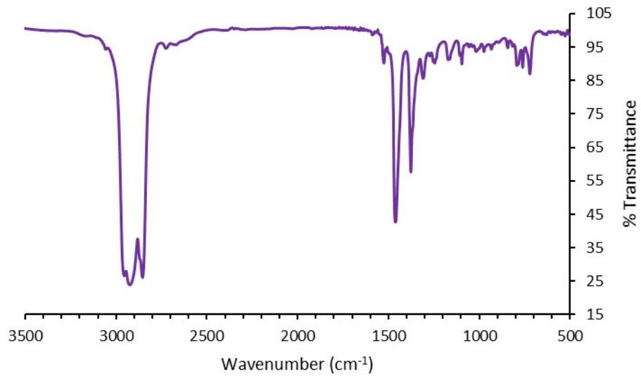
**Figure S30.** FT-IR spectrum (Nujol/KBr) of  $\mu_2\text{-Ge}[\text{Re}(\eta^5\text{-Cp})(\text{BDI})]_2$  (**3**).
