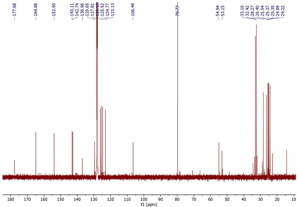
**Figure S2.**  $^{13}\text{C}$  NMR spectrum of  $\text{Re}(\text{Si}[\text{PhC}(\text{N}'\text{Bu})_2])(\eta^5\text{-Cp})(\text{BDI})$  (**1a**) in  $\text{C}_6\text{D}_6$  (151 MHz, 298 K).
