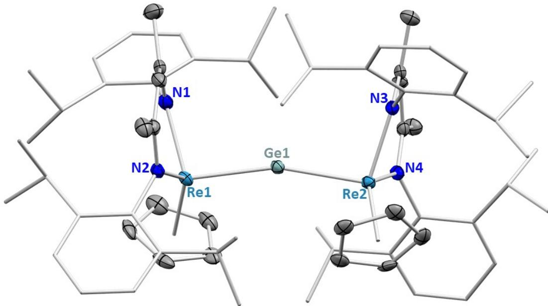
**Figure S24.** X-ray crystal structure of **3** with 50% probability ellipsoids. The BDI diisopropylphenyl groups are shown in wireframe, and hydrogen atoms are omitted for clarity. A pentane molecule, which can be found in the asymmetric unit, is also omitted.
