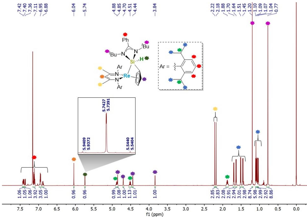
**Figure S3.**  $^1\text{H}$  NMR spectrum of  $(\text{BDI})\text{Re}(\mu-\eta^5:\eta^1\text{-Cp})(\text{SiH}[\text{PhC}(\text{N}^t\text{Bu})_2])$  (**1b**) in  $\text{C}_6\text{D}_6$  (600 MHz, 298 K). Minor  $^{29}\text{Si}$  satellites can be observed at 5.54 and 5.94 ppm corresponding to one-bond coupling of the silane proton with silicon (inset). An internal standard of  $\text{SiMe}_4$  (0 ppm) is also present.
