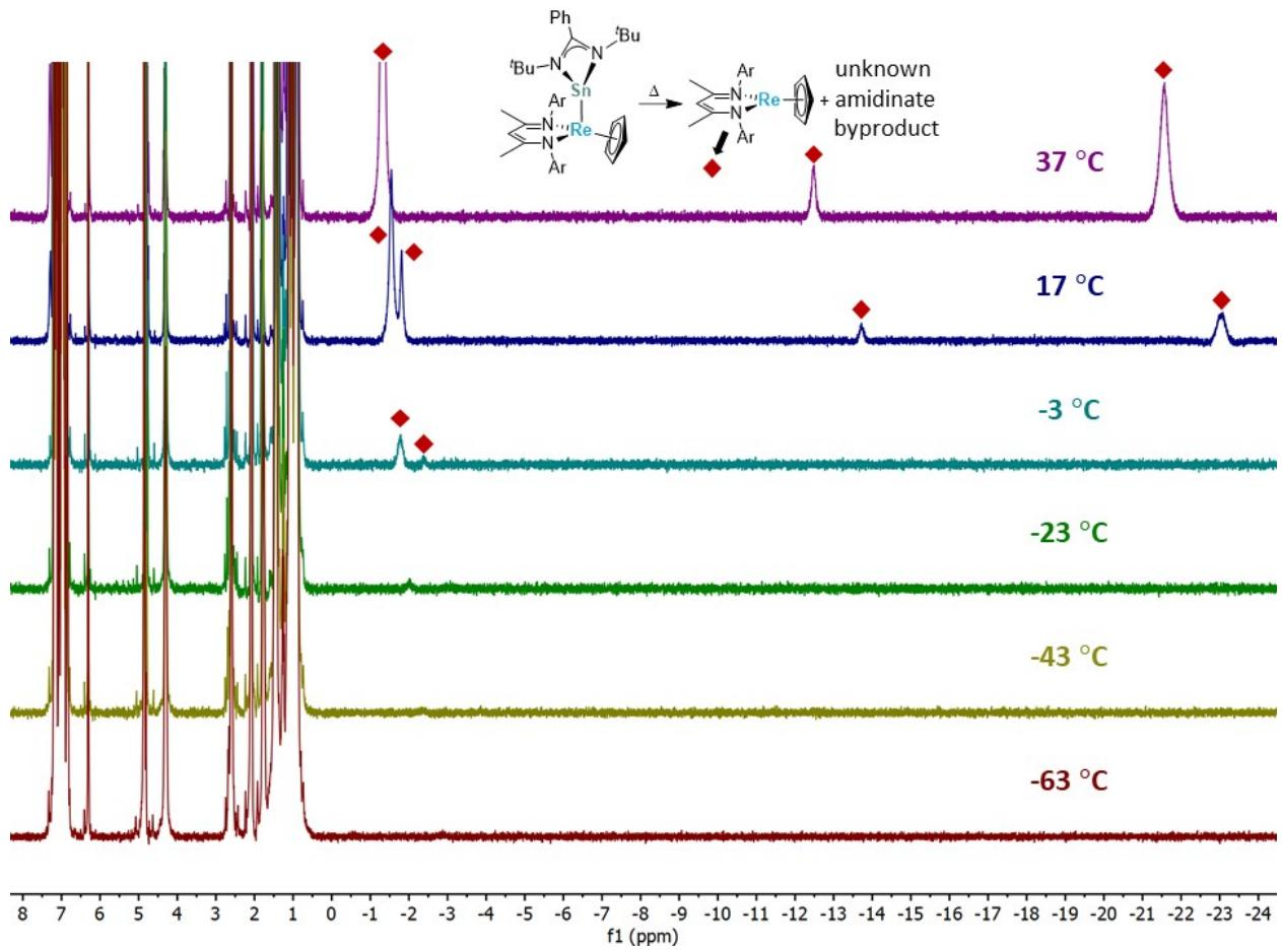
**Figure S16.** Variable temperature <sup>1</sup>H NMR spectrum of the upfield region of  $\text{Re}(\text{Sn}[\text{PhC}(\text{N}'\text{Bu})_2])(\eta^5\text{-Cp})(\text{BDI})$  (**4**) in toluene-*d*<sub>8</sub> (400 MHz, 210–310 K). Starting at ~270 K, the product **4** begins to decompose into paramagnetic  $\text{Re}(\eta^5\text{-Cp})(\text{BDI})^1$  as well as an unknown amidinate byproduct.
