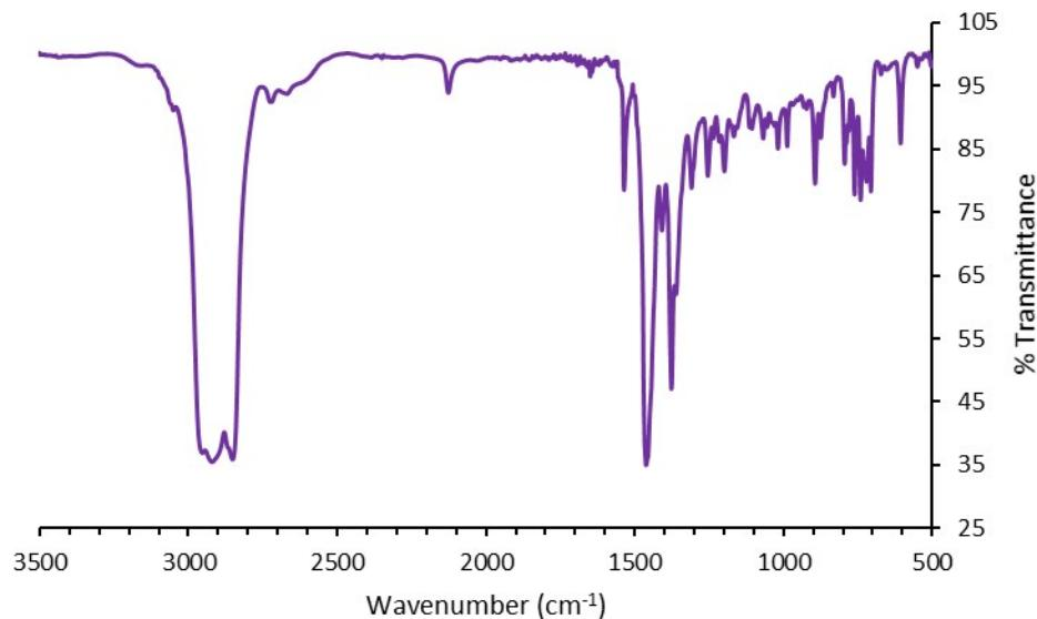
**Figure S27.** FT-IR spectrum (Nujol/KBr) of  $(\text{BDI})\text{Re}(\mu\text{-}\eta^5\text{:}\eta^1\text{-Cp})(\text{SiH}[\text{PhC}(\text{N}'\text{Bu})_2])$  (**1b**).  $\nu_{\text{Si-H}}$   $2128 \text{ cm}^{-1}$ .
