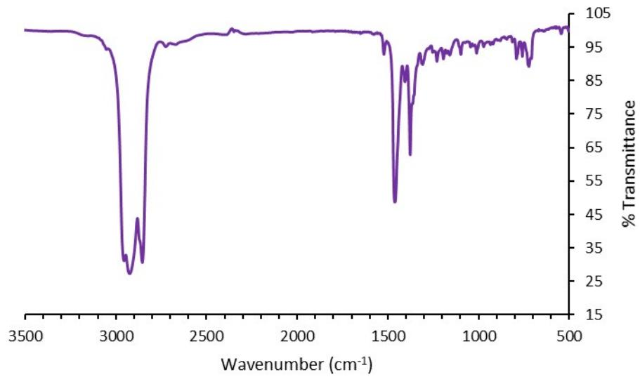
**Figure S31.** FT-IR spectrum (Nujol/KBr) of  $\text{Re}(\text{Sn}[\text{PhC}(\text{N}'\text{Bu})_2])(\eta^5\text{-Cp})(\text{BDI})$  (**4**).
