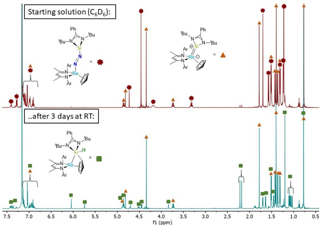
**Figure S8.** Stacked  $^1\text{H}$  NMR spectrum showing conversion of **1c** to **1b** in  $\text{C}_6\text{D}_6$  (700 MHz, 293 K).
