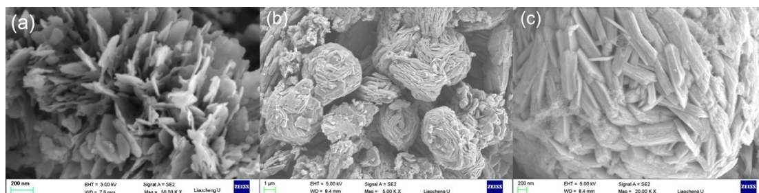
Fig. S1 FESEM image of as-synthesized CSr heterostructure at high magnification (a) and SnS 2 at low and high magnification (b and c).
