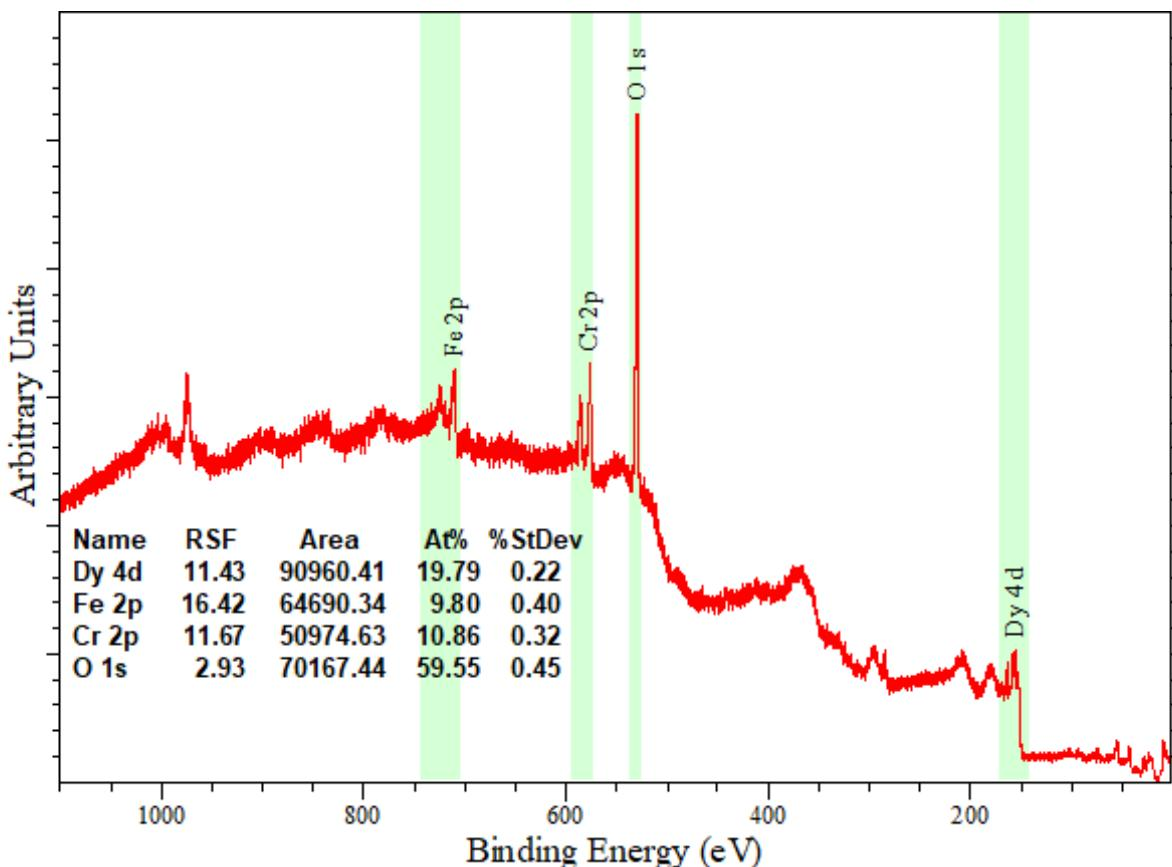
Figure S5. XPS survey spectra of synthesized nanoparticles.
