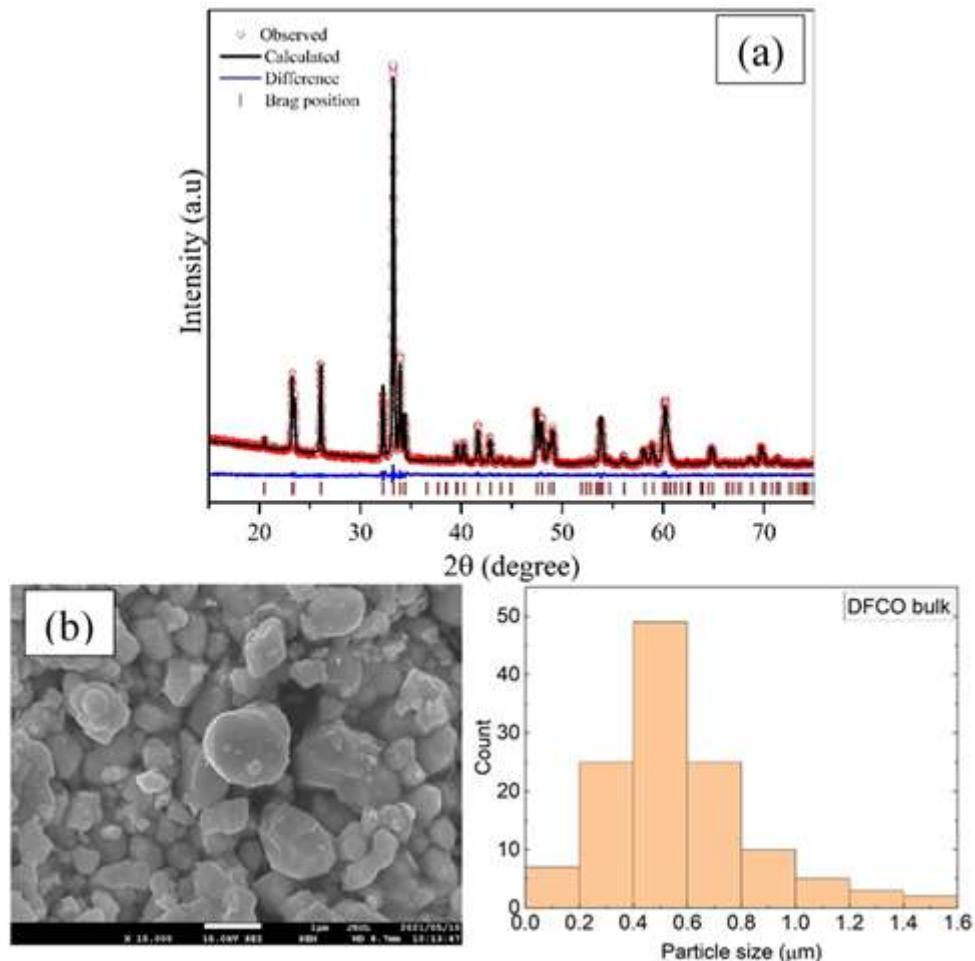
Figure S3: (a) XRD and corresponding Rietveld refinement of bulk sized  $\text{DyFe}_{0.5}\text{Cr}_{0.5}\text{O}_3$  prepared by solid-state reaction technique. (b) FSEM image and histogram of the particle size distribution.
