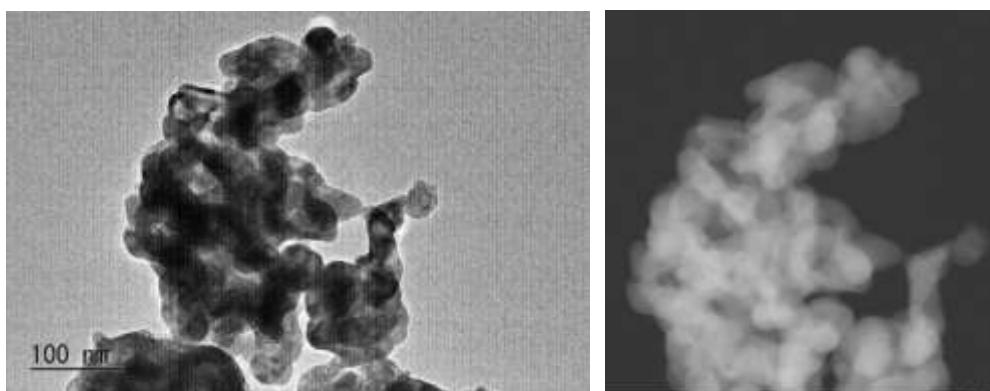
Figure S1. (left) TEM and (right) HAADF-STEM image of  $\text{DyFe}_{0.5}\text{Cr}_{0.5}\text{O}_3$  nanoparticles.
