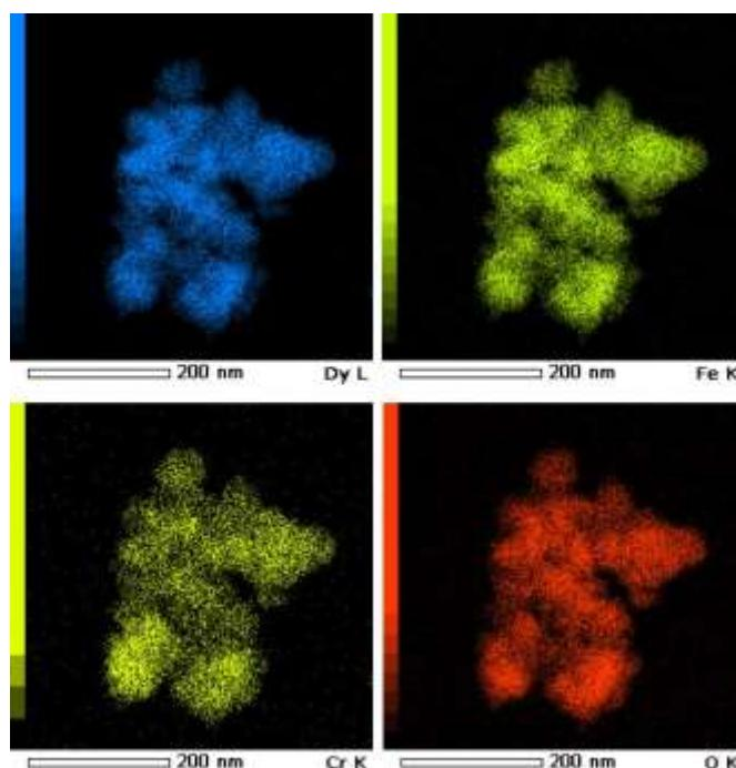
Figure S2. The elemental mapping pattern of Dy, Fe, Cr and O in  $\text{DyFe}_{0.5}\text{Cr}_{0.5}\text{O}_3$  nanoparticles respectively.
