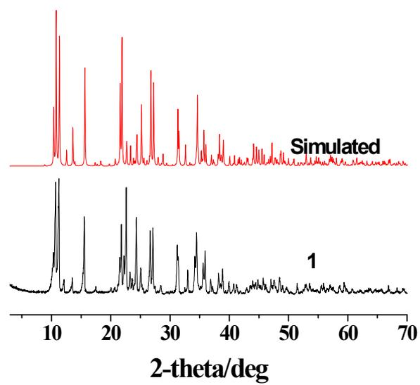
Fig. S3 Simulated and experimental powder XRD patterns of **1**.
