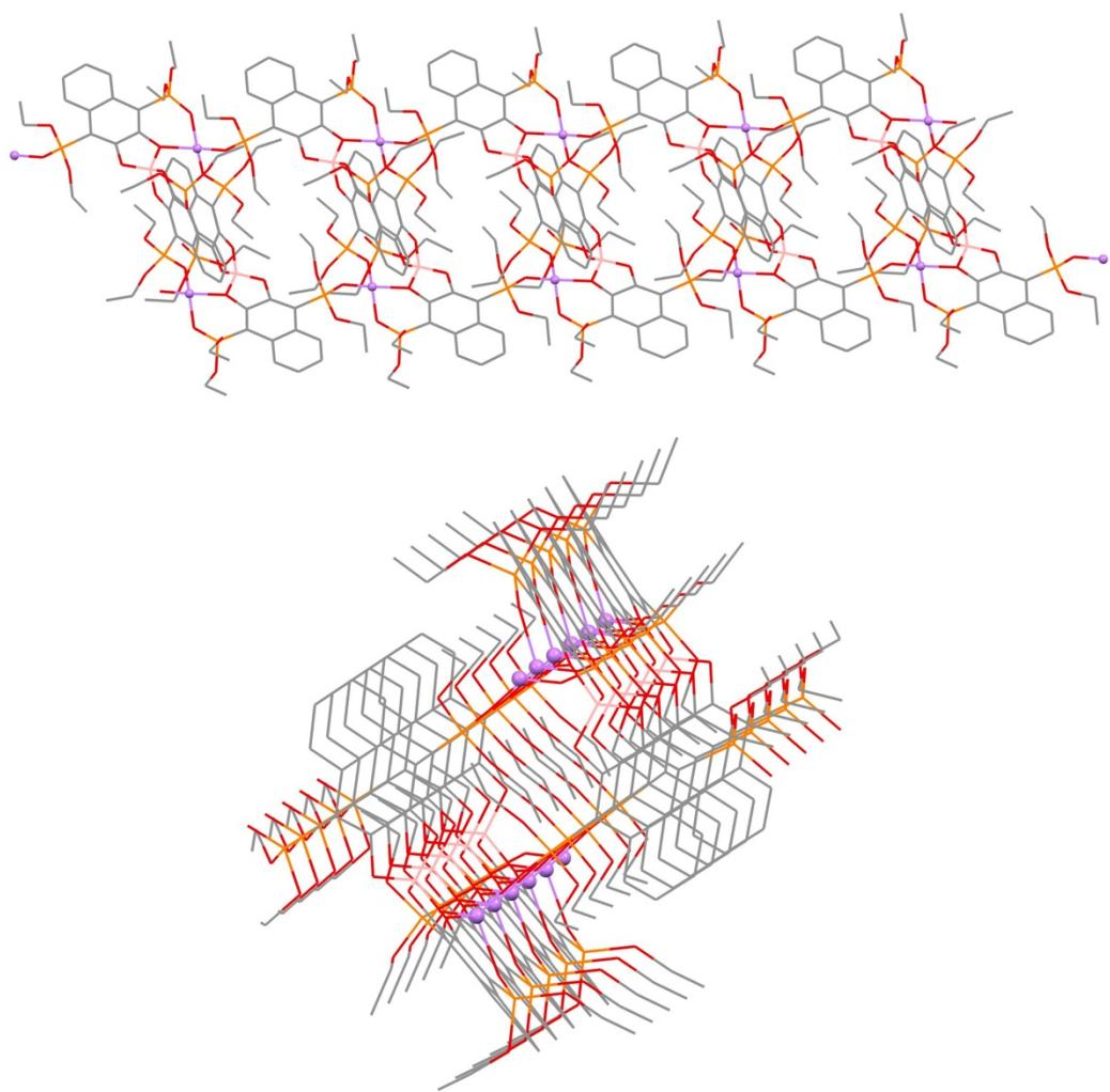
**Figure S20.** Packing diagram of  $\text{Li}[\text{B}(\text{DPN})_2]$  illustrating lithium ions (lavender color) bridging pairs of independent molecules to one another (along a-axis).
