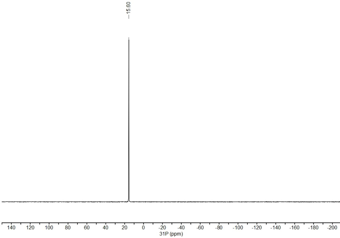
**Figure S3.**  $^{31}\text{P}\{^1\text{H}\}$  NMR (202 MHz, DMSO- $d_6$ ) spectrum of  $\text{Li}[\text{B}(\text{DPN})_2]$ .
