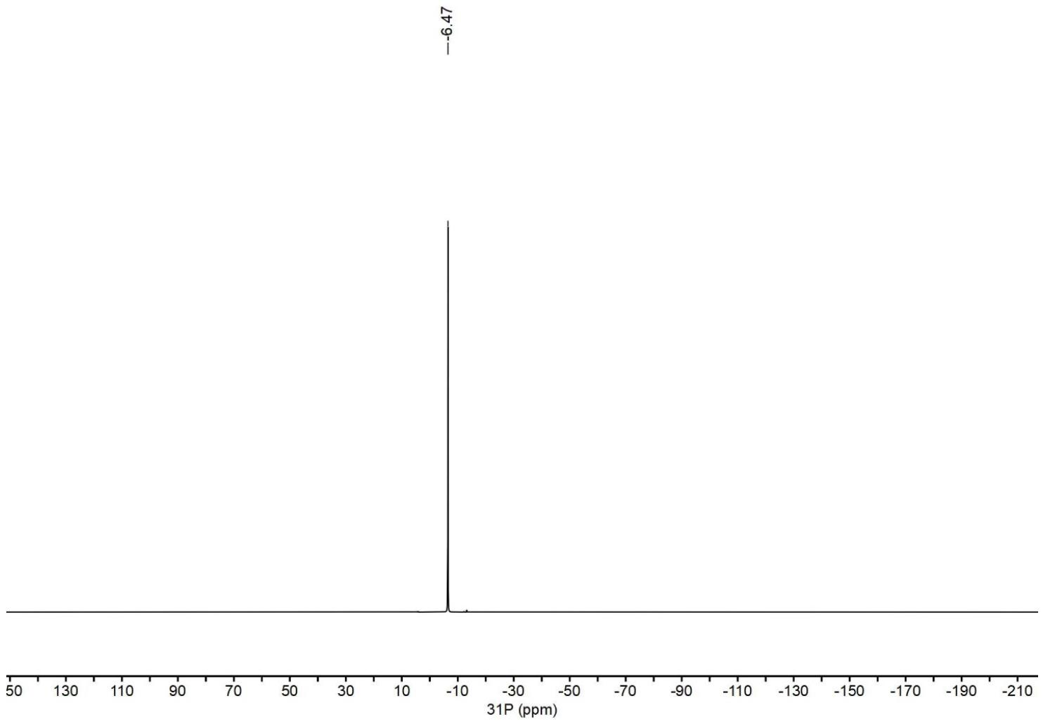
**Figure S9.**  $^{31}\text{P}\{\text{H}\}$  NMR (202 MHz,  $\text{CDCl}_3$ ) spectrum of 2,3-dihydroxy-1,4-diphosphinatonaphthalene.
