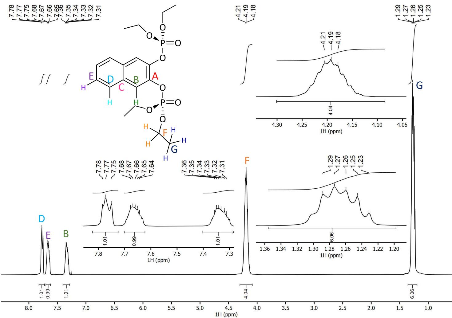
**Figure S8.**  $^1\text{H}$  NMR (500 MHz,  $\text{CDCl}_3$ ) spectrum of 2,3-dihydroxy-1,4-diphosphinatonaphthalene.
