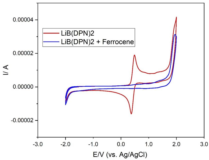
**Figure S19.** Cyclic Voltammograms of  $\text{Li}[\text{B}(\text{DPN})_2]$  (0.1 mM) with ferrocene (0.1 mM) as a standard and  $\text{Li}[\text{B}(\text{DPN})_2]$  (0.1 mM);  $[\text{Bu}_4\text{N}] \text{PF}_6$  (Tetrabutylammonium hexafluorophosphate) 0.1 M in DCM, working electrode: glassy carbon (3 mm), reference electrode: non-aqueous  $\text{Ag}/\text{Ag}^+$ , counter electrode: Pt (2 mm), potential window: -2.0 V – 2.0 V with a scan rate of  $0.08 \text{ V s}^{-1}$ .
