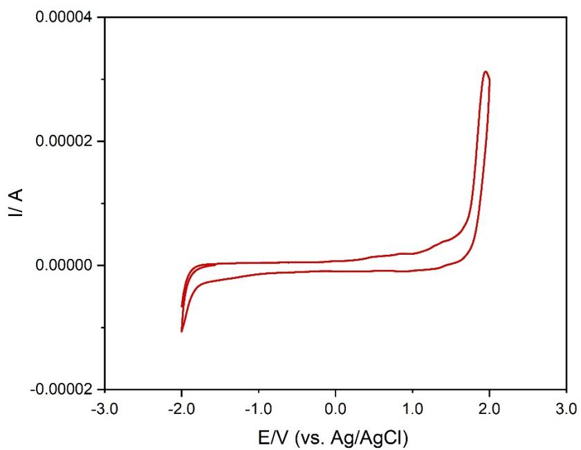
**Figure S17.** Cyclic Voltammogram of  $\text{Li}[\text{B}(\text{DPN})_2]$  (0.1 mM);  $[\text{Bu}_4\text{N}] \text{PF}_6$  (Tetrabutylammonium hexafluorophosphate) 0.1 M in DCM, working electrode: glassy carbon (3 mm), reference electrode: non-aqueous  $\text{Ag}/\text{Ag}^+$ , counter electrode: Pt (2 mm), potential window: -2.0 V – 2.0 V) with a scan rate of  $0.08 \text{ V s}^{-1}$ .
