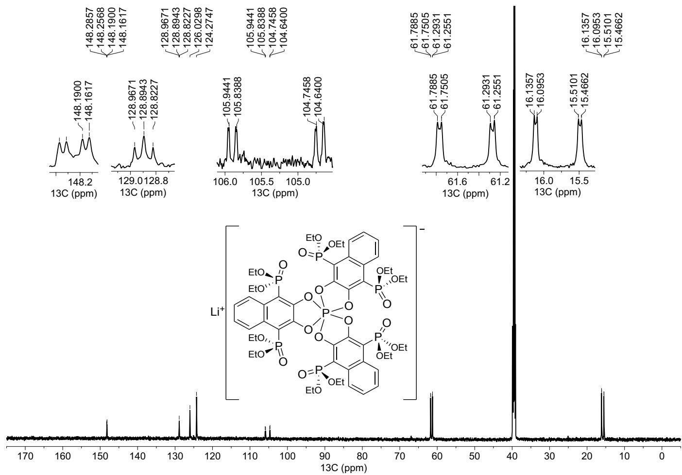
**Figure S15.**  $^{13}\text{C}\{\text{H}\}$  NMR (400 MHz,  $\text{DMSO-d}_6$ ) spectrum of  $\text{Li}[\text{P}(\text{DPN})_3]$ .
