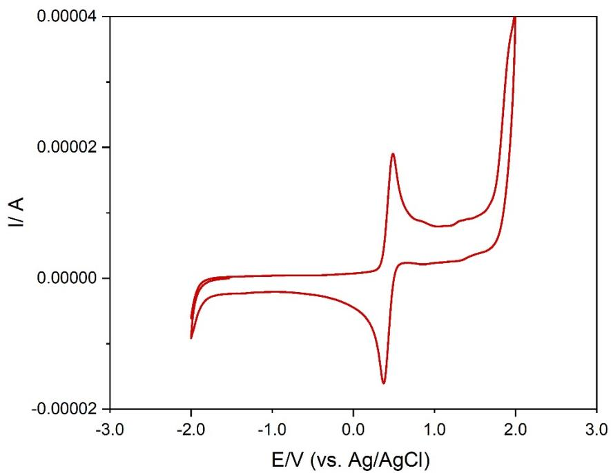
**Figure S18.** Cyclic Voltammogram of  $\text{Li}[\text{B}(\text{DPN})_2]$  (0.1 mM) with ferrocene (0.1 mM) as a standard;  $[\text{Bu}_4\text{N}] \text{PF}_6$  (Tetrabutylammonium hexafluorophosphate) 0.1 M in DCM, working electrode: glassy carbon (3 mm), reference electrode: non-aqueous  $\text{Ag}/\text{Ag}^+$ , counter electrode: Pt (2 mm), potential window: -2.0 V – 2.0 V with a scan rate of  $0.08 \text{ V s}^{-1}$ .
