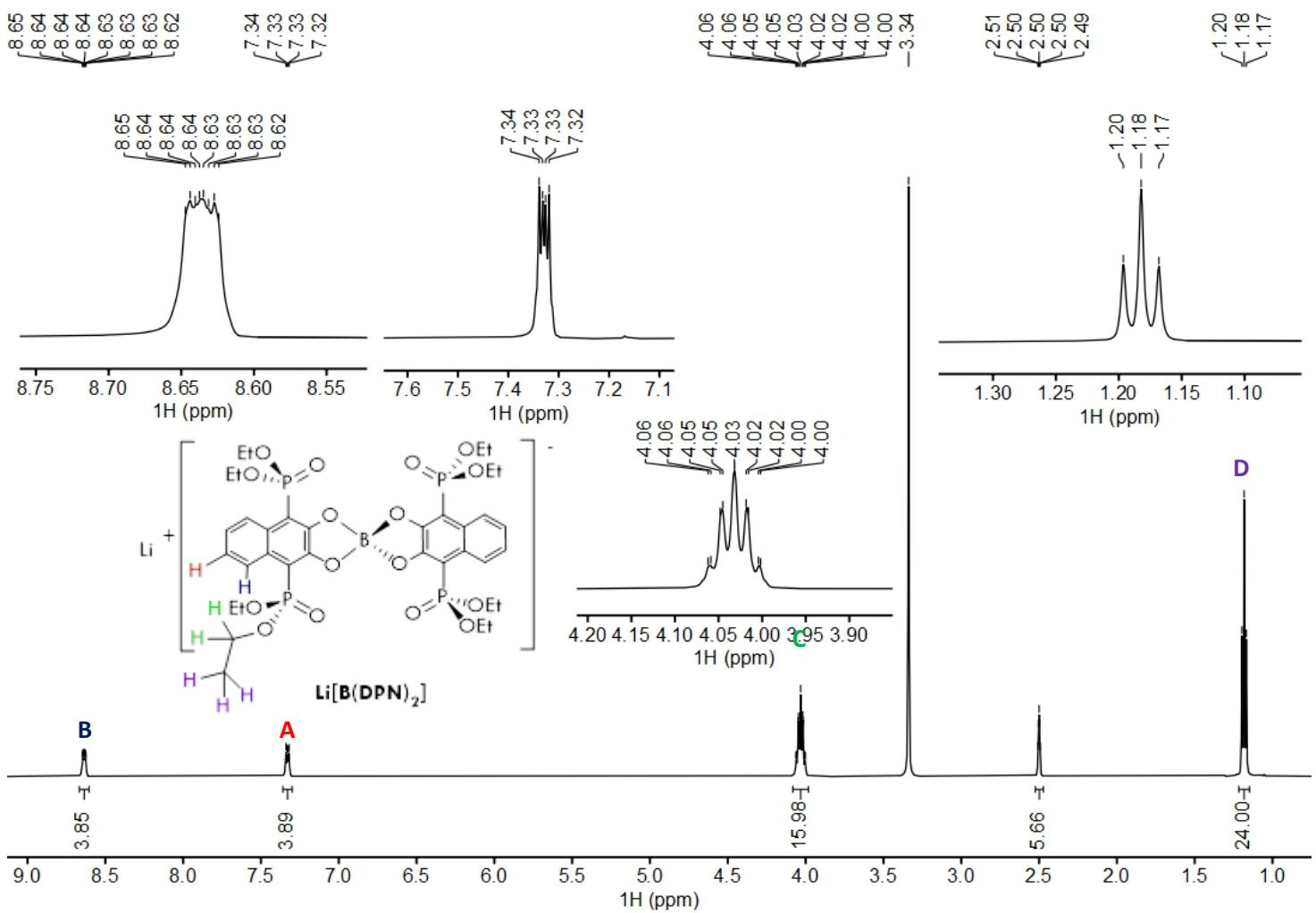
**Figure S1.**  $^1\text{H}$  NMR (500 MHz,  $\text{DMSO-d}_6$ ) spectrum of  $\text{Li}[\text{B}(\text{DPN})_2]$ .
