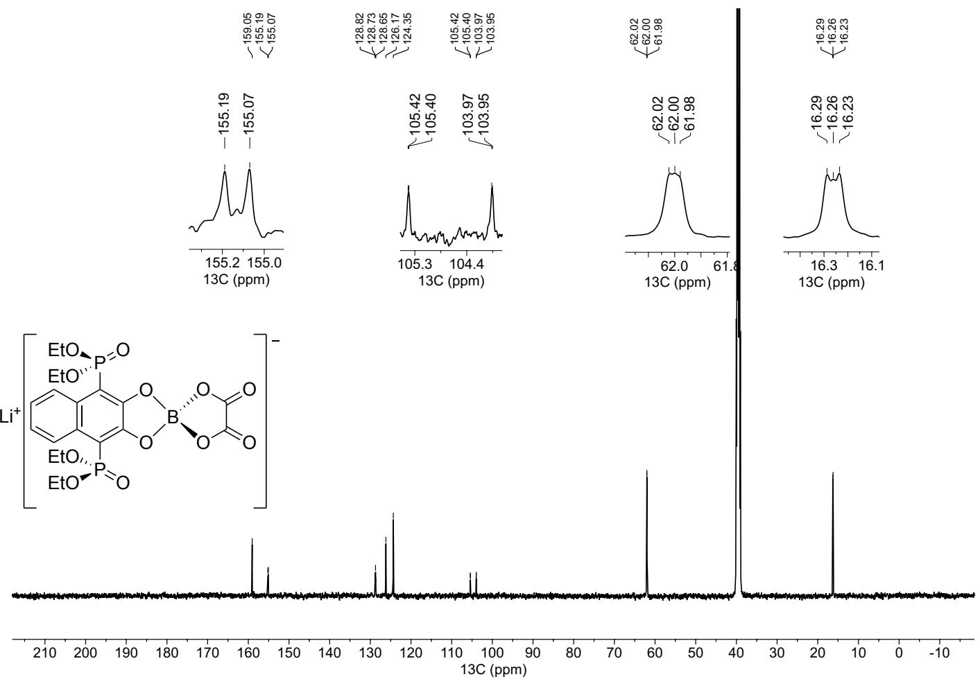
**Figure S11.**  $^{13}\text{C}\{^1\text{H}\}$  NMR (500 MHz,  $\text{CDCl}_3$ ) spectrum of  $\text{Li}[\text{B}(\text{DPN})(\text{oxalato})]$ .
