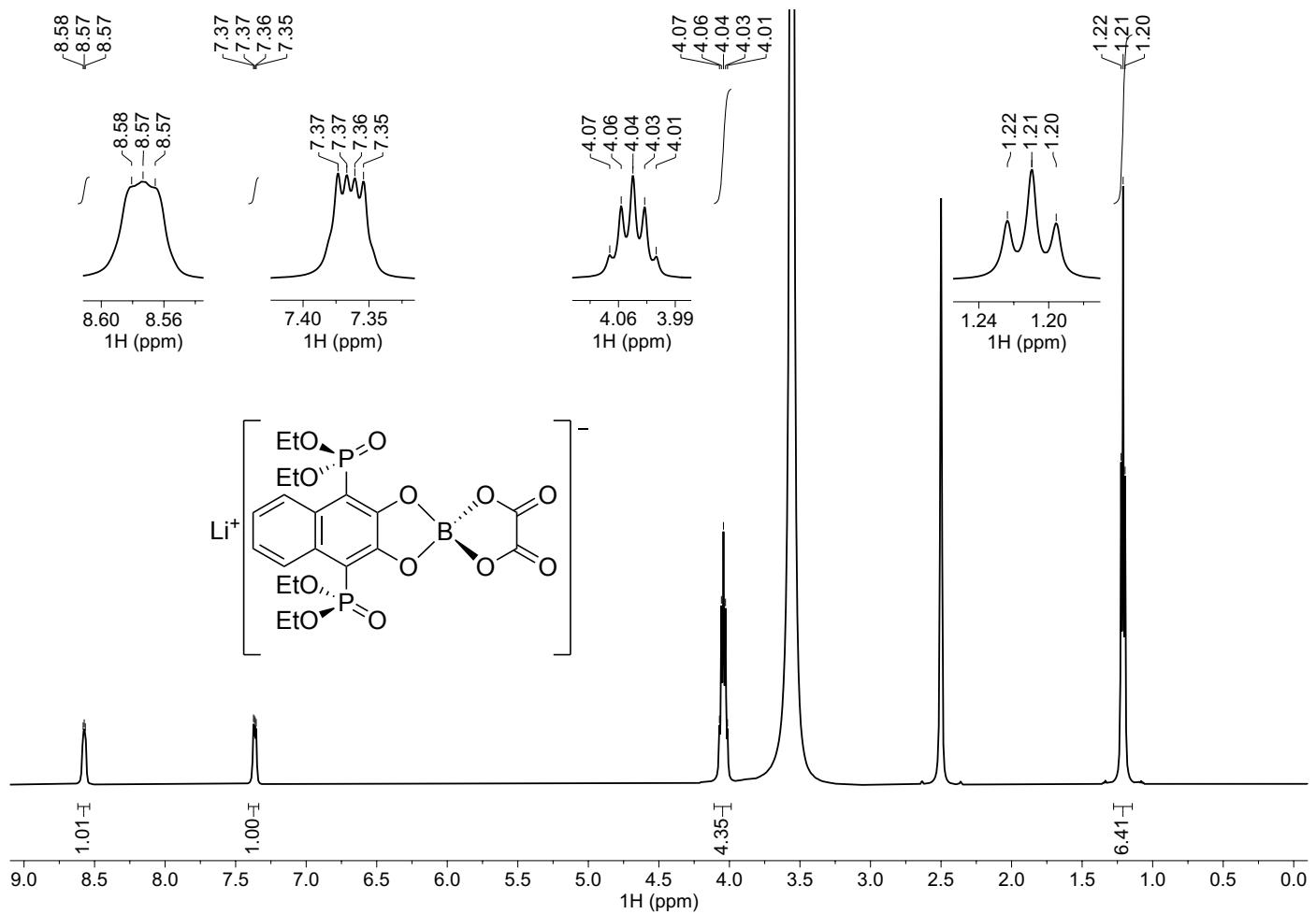
**Figure S10.**  $^1\text{H}$  NMR (500 MHz,  $\text{DMSO-d}_6$ ) spectrum of  $\text{Li}[\text{B}(\text{DPN})(\text{oxalato})]$ .
