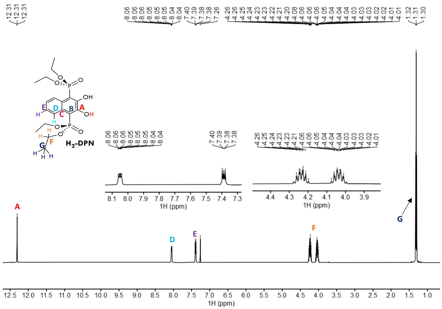
**Figure S5.**  $^1\text{H}$  NMR (500 MHz,  $\text{CDCl}_3$ ) spectrum of  $\text{H}_2\text{-DPN}$ .
