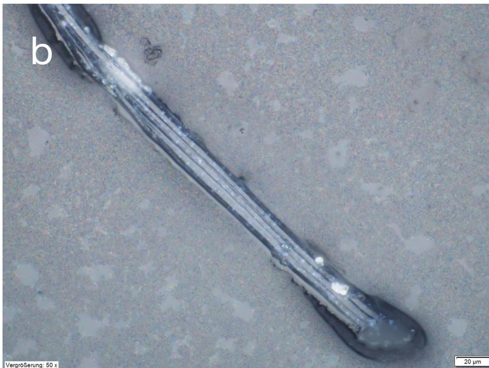
Fig. SI 1: (a) SEM (scale bar 300 microns) and (b) OPM image (scale bar 20 microns) of fibers obtained with hydrothermal synthesis at 120 °C (*Na-2-ht*).
