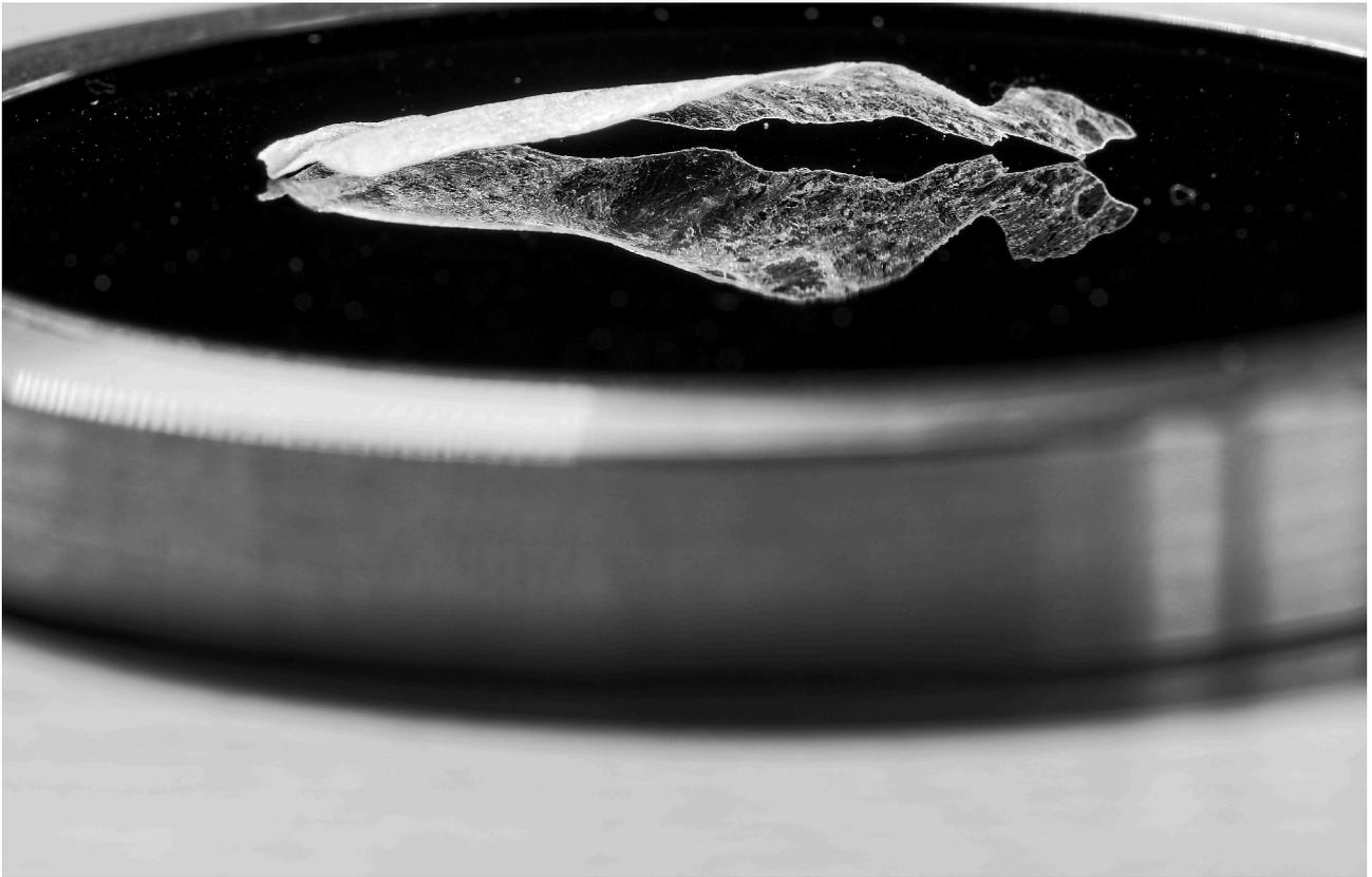
Fig. SI 6: Self-supporting film of freeze-dried *Na-2* dispersion.
