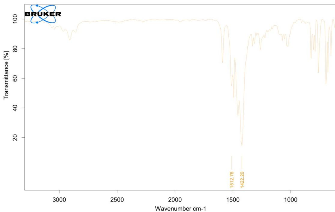
**Fig. S6.** IR spectrum of **5**, with the bands assigned to the  $\kappa^2$ -carbamate ligands highlighted.
