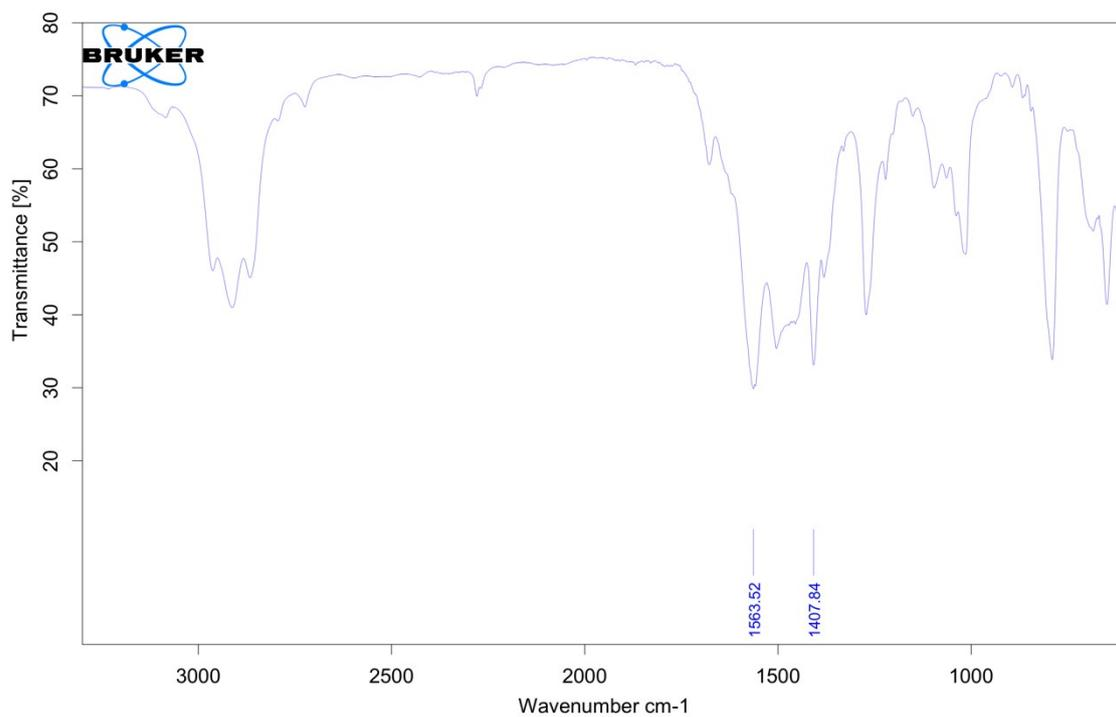
**Fig. S5.** IR spectrum of **4**, with the bands assigned to the  $\eta^1$ -carbamate ligand highlighted.
