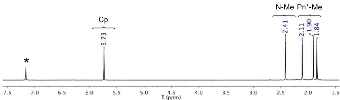
**Fig. S1.**  $^1\text{H}$  NMR spectrum (400 MHz,  $\text{C}_6\text{D}_6$ , 298 K) of  $\text{Pn}^*\text{ZrCp}(\text{NMe}_2)$  (1). \* denotes residual protio solvent.
