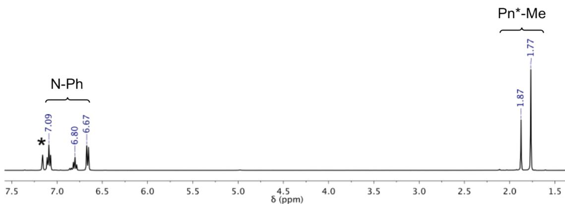
**Fig. S2.**  $^1\text{H}$  NMR spectrum (400 MHz,  $\text{C}_6\text{D}_6$ , 298 K) of  $\text{Pn}^*\text{Zr}(\text{NPh})_2$  (3). \* denotes residual protio solvent.
