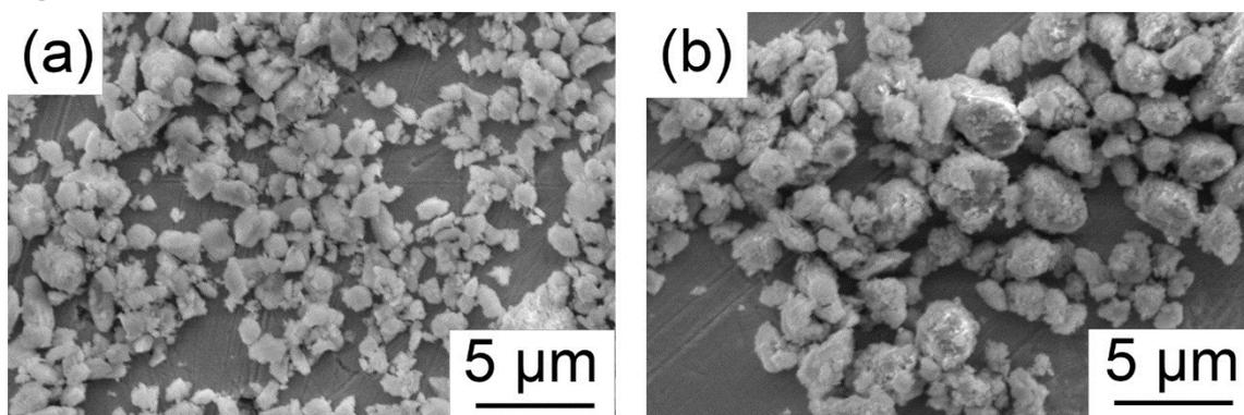
Figure S5 SEM images of the Eu-doped products (a)  $\text{Ba}_3\text{Si}_6\text{O}_{12}\text{N}_2$  at 800 °C and (b)  $\text{Ba}_3\text{Si}_6\text{O}_9\text{N}_4$  at 950 °C obtained for 15 h under a  $\text{N}_2$  atmosphere.
