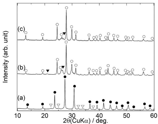
Figure S4 XRD patterns for products obtained at (a) 800 °C for 15 h, (b) 800 °C for 50 h and (c) 950 °C for 15 h in Ta container sealed under  $\text{N}_2$  atmosphere. The filled and open circles and filled and open triangles indicate peaks attributed to  $\text{Ba}_3\text{Si}_6\text{O}_{12}\text{N}_2$ ,  $\text{Ba}_3\text{Si}_6\text{O}_9\text{N}_4$ ,  $\text{SiO}_2$  and  $\text{BaCO}_3$ , respectively.
