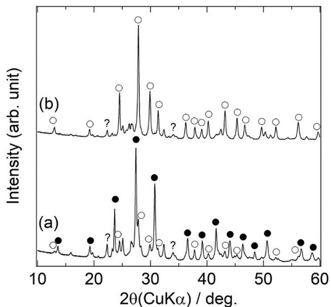
Figure S3 XRD patterns for the products obtained at (a) 800 °C and (b) 950 °C after 15 h under Ar flow of 50 mL/min. The filled and open circles indicate peaks attributed to  $\text{Ba}_3\text{Si}_6\text{O}_{12}\text{N}_2$  and  $\text{Ba}_3\text{Si}_6\text{O}_9\text{N}_4$ , respectively. Unknown peaks are marked with “?”.
