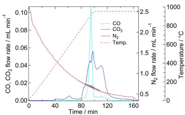
Figure S2 GC curves for CO, CO<sub>2</sub> and N<sub>2</sub> gases released from  $\text{BaCN}_2/2\text{SiO}_2$  mixture under Ar flow. The heating rate was 10 °C/min, which was the same as that for the TG-DTA measurement. Obvious nitrogen gas generation was observed around 800 °C, emphasized as a hatched area on the curve.
