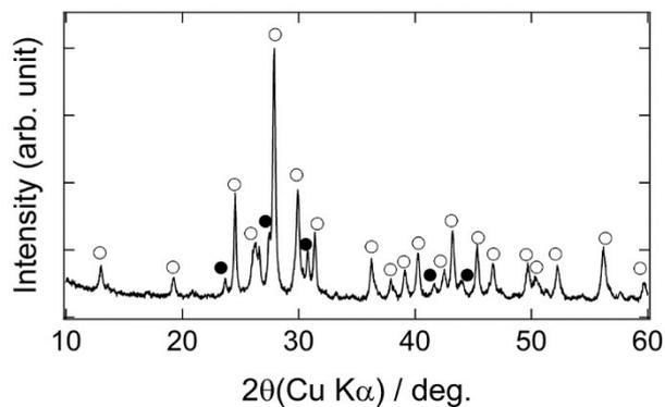
Figure S1 XRD pattern for the sample after the Q-MS analysis under Ar flow. The filled and open circles indicate peaks attributed to  $\text{Ba}_3\text{Si}_6\text{O}_{12}\text{N}_2$  and  $\text{Ba}_3\text{Si}_6\text{O}_9\text{N}_4$ , respectively.
