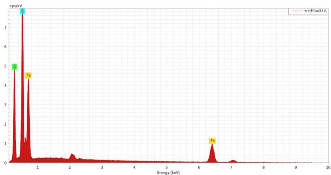
**Fig.S2** The EDS images of  $\text{Fe}_2\text{O}_3@\text{C}@\text{Fe}_2\text{O}_3$ .
