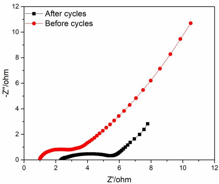
**Fig.S7** The EIS curves of ASCs device before and after cycles.
