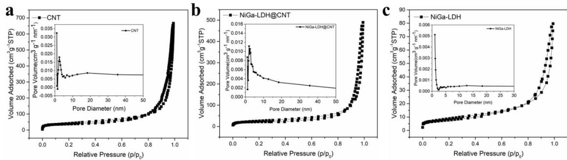
**Fig.S3.** Nitrogen adsorption-desorption isotherms and the corresponding pore size distribution of the as-prepared CNT, NiGa-LDH@CNT and NiGa-LDH electrode materials.
