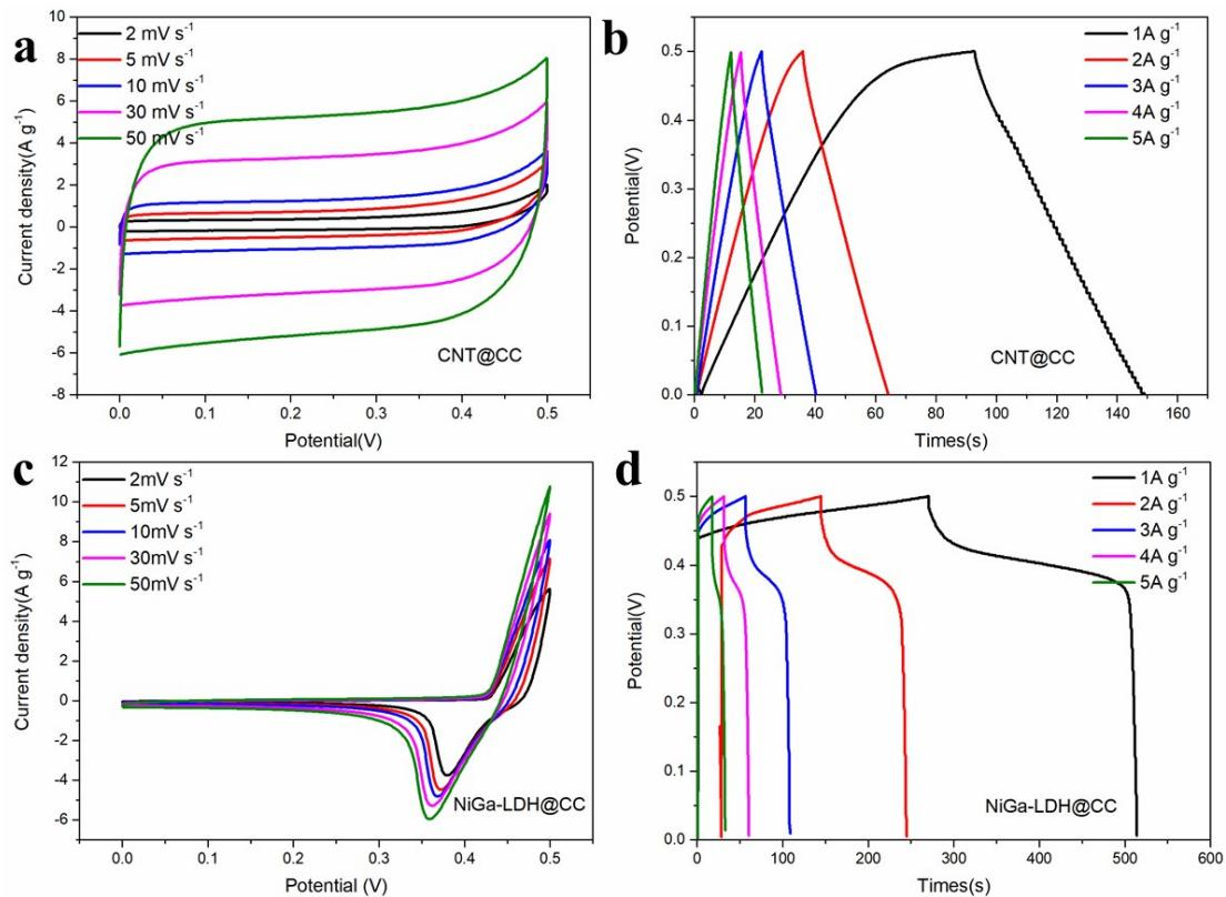
**Fig.S4** The CV and GCD curves of (a) and (b) CNT@CC; (c) and (d) NiGa-LDH@CC.
