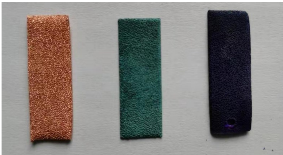
Fig. S1. Picture of the composite samples, the order from left to right is CF, \text{Cu}(\text{OH})_2/\text{CF} and \text{Cu}(\text{OH})_2@ZIF-67/\text{CF} .
