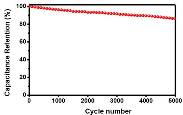
**Fig. S6** Cycling performance of Co<sub>9</sub>S<sub>8</sub>-aCNT-NiCoLDH electrodes after 5000 cycles at 10 A g<sup>-1</sup>.
