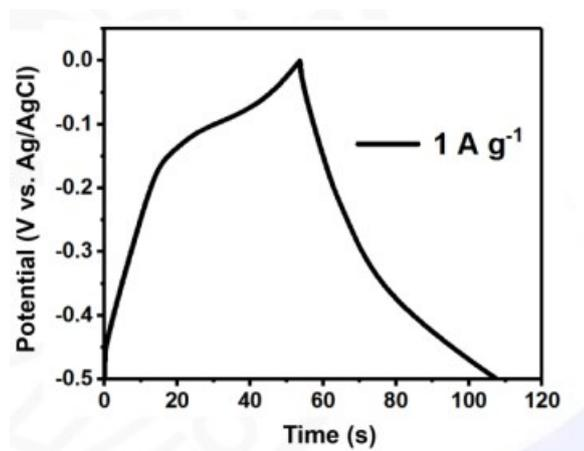
**Fig. S7** GCD curves of active carbon (AC) at 1 A g<sup>-1</sup>
