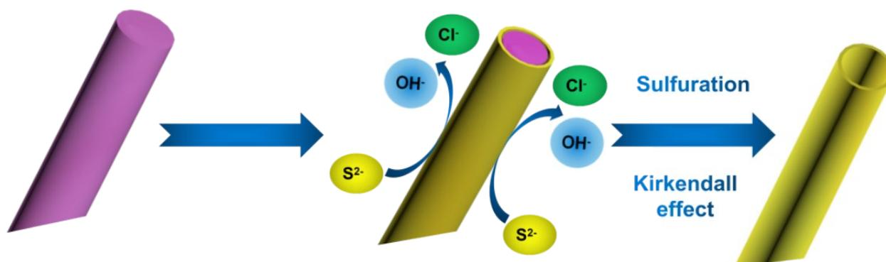
**Fig. S1** Schematic diagram of Ke-Kendal effect.
