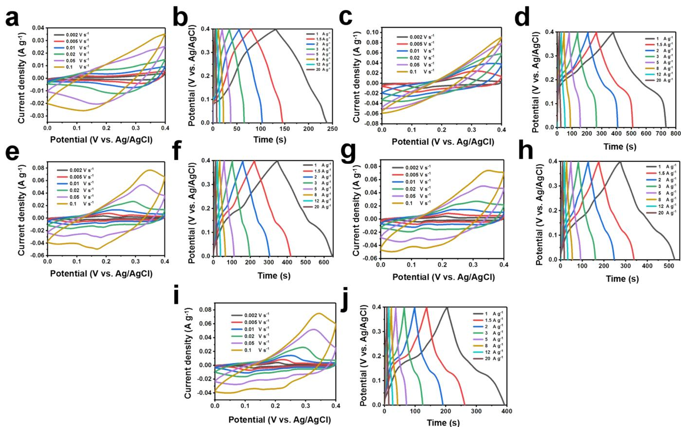
**Fig. S4** a-j CV curves and GCD curves of (a, b)  $\text{Co}_9\text{S}_8$ , (c, d) NiCoLDH, (e, f)  $\text{Co}_9\text{S}_8\text{-aCNT}$ , (g, h)  $\text{Co}_9\text{S}_8\text{-aCNT}$  (low) and (i, g)  $\text{Co}_9\text{S}_8\text{-aCNT}$  (high).
