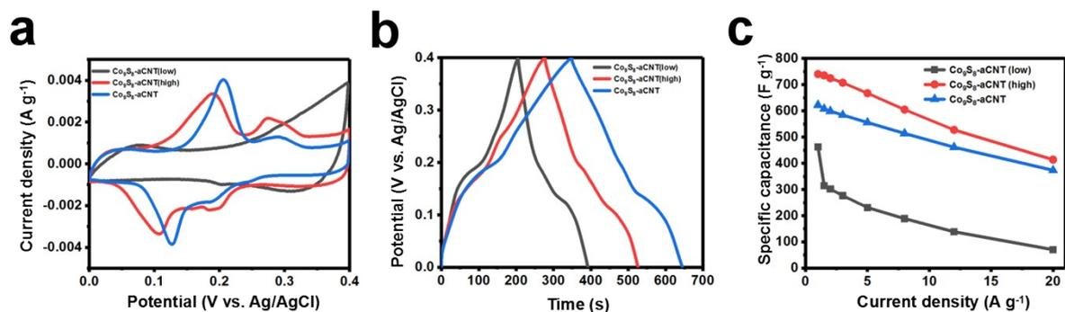
**Fig. S5** Comparison of (a) CV curve, (b) GCD curves and (c) specific capacitance of  $\text{Co}_9\text{S}_8\text{-aCNT}$  (low),  $\text{Co}_9\text{S}_8\text{-aCNT}$  (high) and  $\text{Co}_9\text{S}_8\text{-aCNT}$ .
