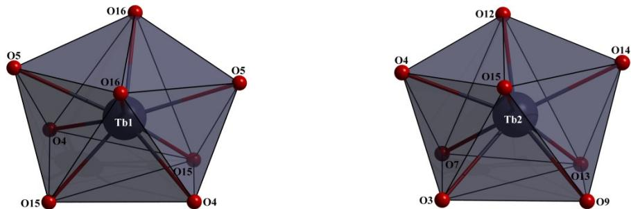
**Figure S1.** Distorted Triangular Dodecahedron (TDD) geometry around Tb1 (left) and distorted Square Antiprism (SAPR) geometry around Tb2 (right) in **1**.
