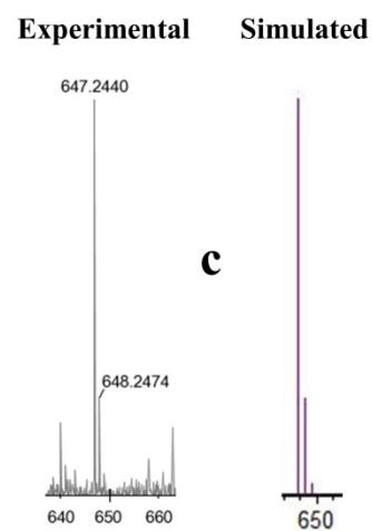
**Figure S10.** Experimental and simulated peaks obtained from HRMS (+ve) of **1** in MeOH corresponding to different species present in solution.
