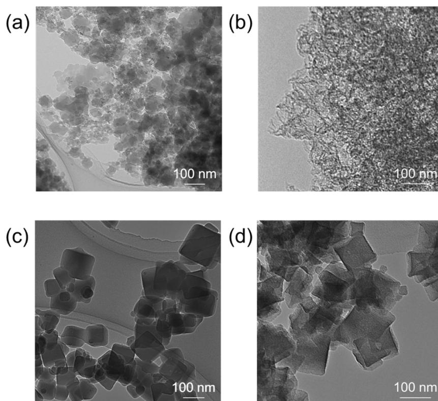
**Fig. S10** TEM photographs of Co-ZIF-8 NSs (a) before and (b) after calcination, and of conventional Co-ZIF-8 crystals (c) before and (d) after calcination.
