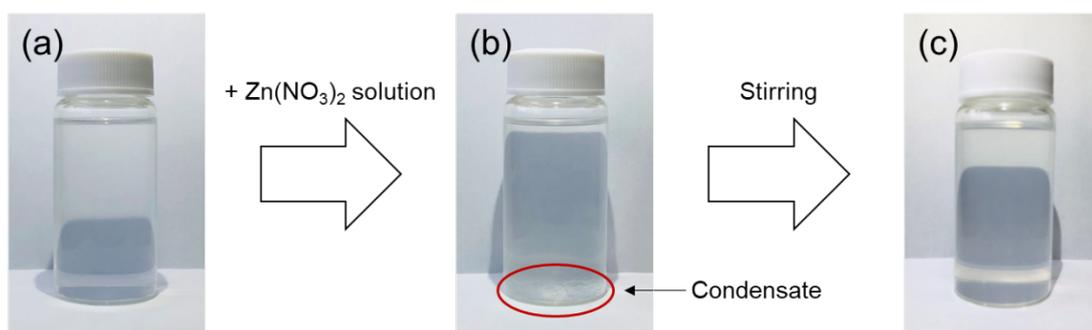
**Fig. S1** Addition of the aqueous  $\text{Zn}(\text{NO}_3)_2$  solution to the decane solution of hydrophilic TRAPs. (a) Before adding the aqueous  $\text{Zn}(\text{NO}_3)_2$  solution, the decane solution is clear. (b) The mixture becomes turbid once immediately after adding  $\text{Zn}(\text{NO}_3)_2$ . (c) After stirring, the mixture becomes clear again.
