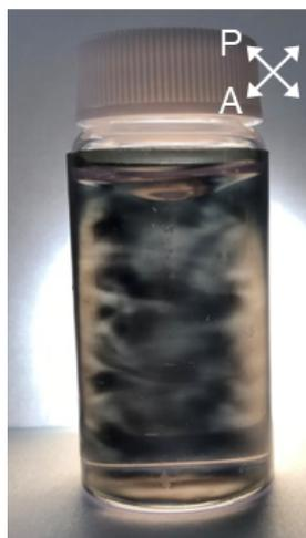
**Fig. S6** Polarized photograph of a hyperswollen lyotropic lamellar phase of decane solution of Brij L4 ( $1.8 \times 10^{-1}$  M), water (1.0 M), ammonium hydroxide ( $1.2 \times 10^{-2}$  M), 2-mim ( $2.8 \times 10^{-3}$  M),  $\text{Zn}(\text{NO}_3)_2$  ( $1.2 \times 10^{-3}$  M), and  $\text{Co}(\text{NO}_3)_2$  ( $6.1 \times 10^{-5}$  M).
