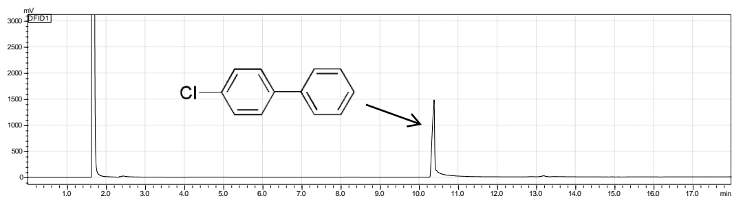
Fig. S31 GC of the reaction of 4-chlorophenylboronic acid and iodobenzene.
