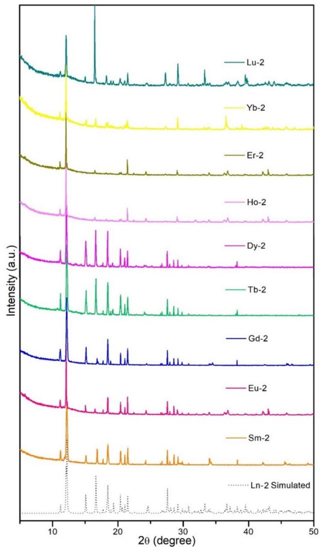
**Fig. S2** The Powder X-ray diffraction (PXRD) patterns of **Ln-2** (Ln = Sm, Eu, Gd, Tb, Dy, Ho, Er, Yb, and Lu). Dashed line simulated patterns; solid line: experimental patterns.
