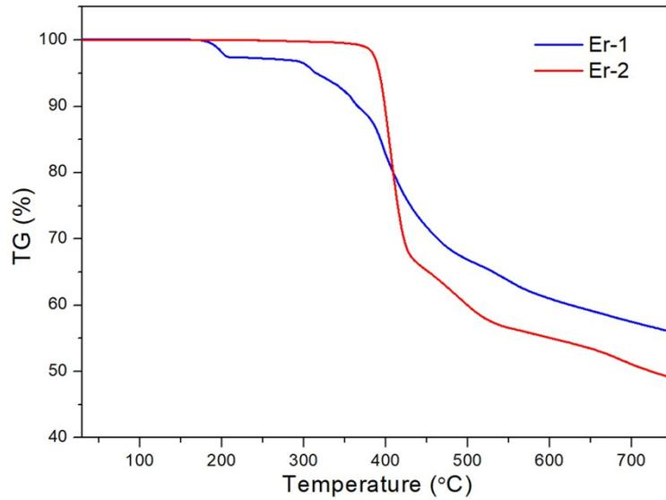
**Fig. S8** The thermogravimetric analysis data showing that **Er-1** and **Er-2** are thermally stable up to 275 and 380 °C, respectively.
