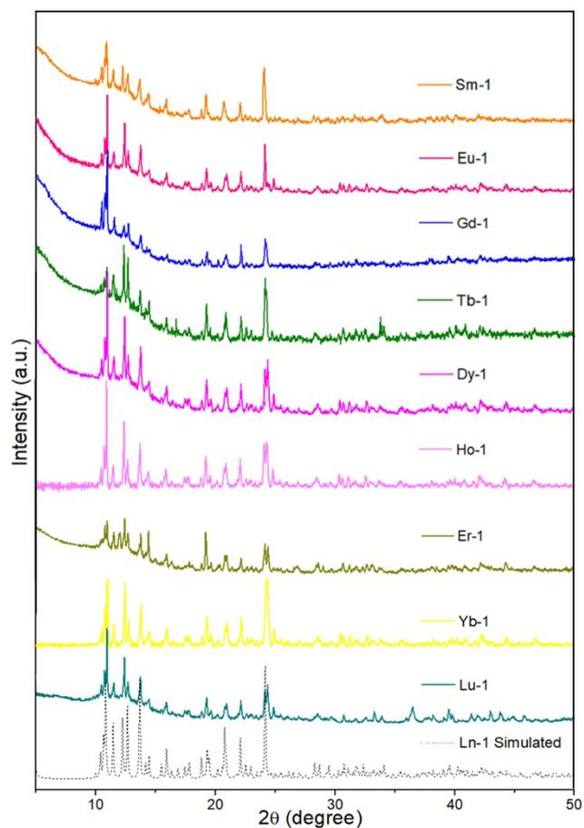
**Fig. S1** The Powder X-ray diffraction (PXRD) patterns of **Ln-1** (Ln = Sm, Eu, Gd, Tb, Dy, Ho, Er, Yb, and Lu). Dashed line simulated patterns; solid line: experimental patterns.
