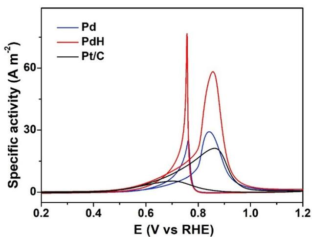
**Figure S7** Cyclic voltammograms of Pd concave cubes,  $\beta$ -PdH concave cubes, and Pt/C in an Ar-saturated 1 M methanol + 1 M KOH electrolyte (scan rate = 50 mVs<sup>-1</sup>) for methanol oxidation.
