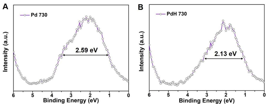
**Figure S3.** XPS valence band structure of (A) Pd concave cubes, and (B) PdH concave cubes.
