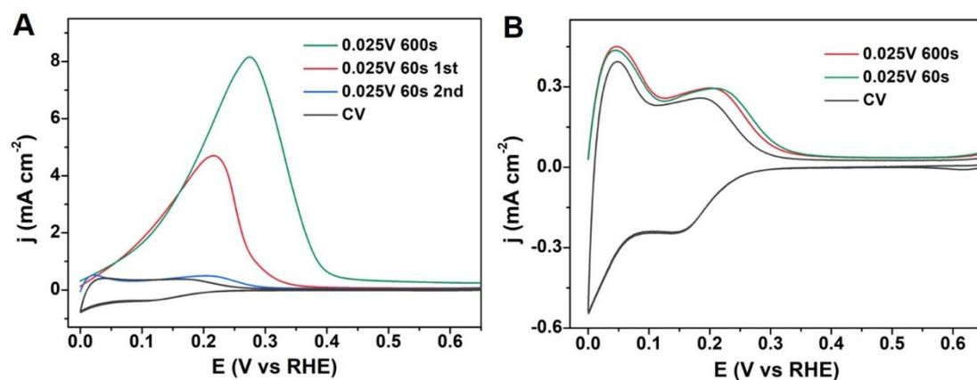
**Figure S5.** H stripping of (A) Pd, and (B) PdH concave nanocubes in Ar-saturated 0.1 M HClO<sub>4</sub> electrolyte (scan rate = 50 mV s<sup>-1</sup>) after the potential was held at 0.025V vs RHE for different holding time.
