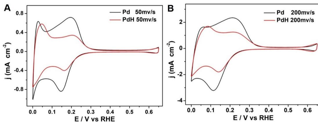
**Figure S4.** Cyclic voltammograms of (A) Pd concave cubes, and (B) PdH concave cubes in Ar-saturated 0.1 M HClO<sub>4</sub> electrolyte with a scan rate of 50 mV s<sup>-1</sup>.
