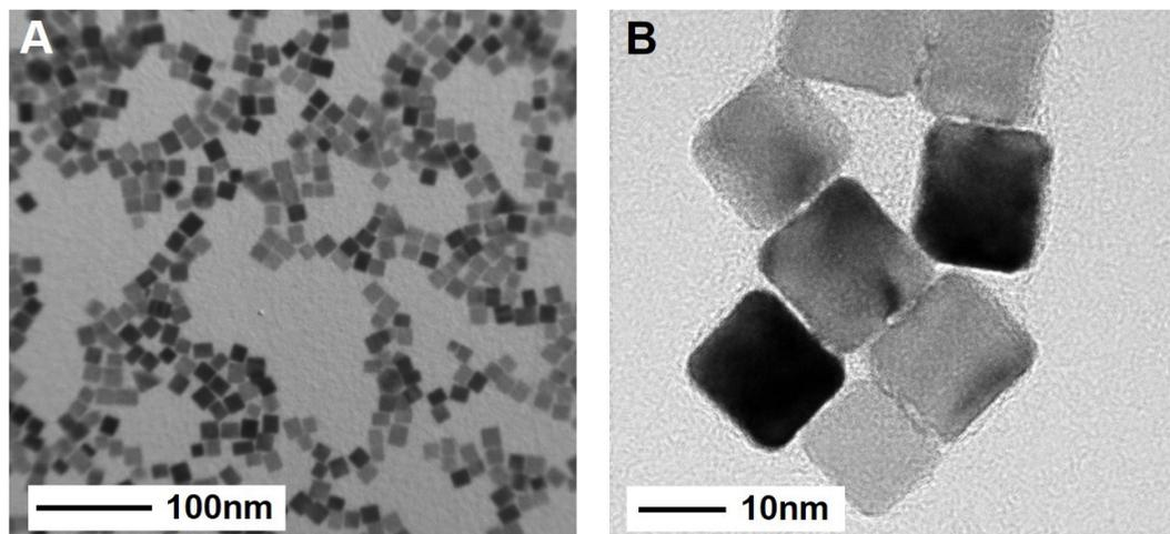
**Figure S1.** (A) TEM and (B) HRTEM images of Pd nanocubes that were used as seeds for the synthesis of concave Pd nanocubes.
