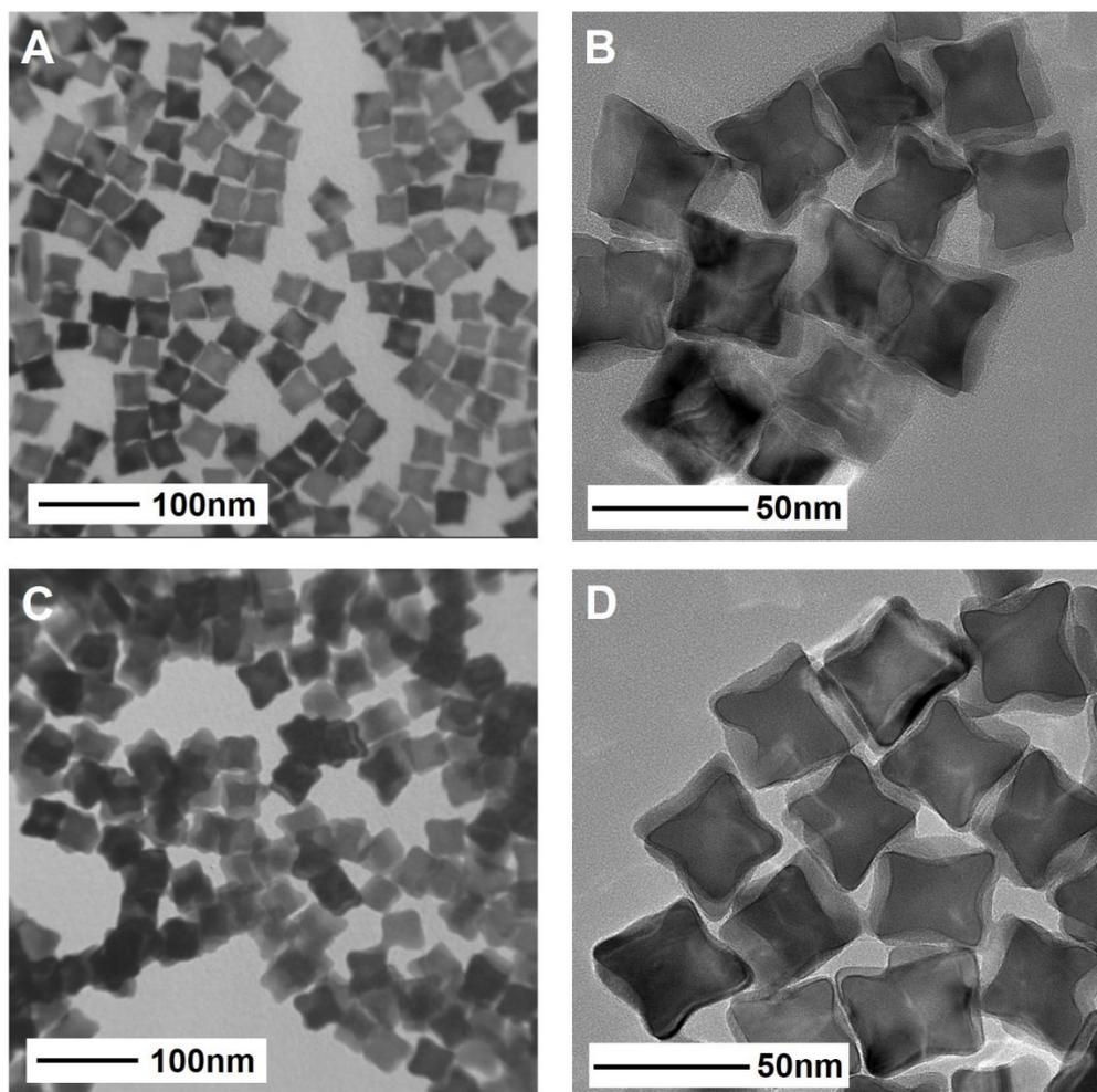
**Figure S2.** TEM images of (A) Pd concave cubes, (C) PdH concave cubes, and HRTEM images of (C) Pd concave cubes, (D) PdH concave cubes respectively.
