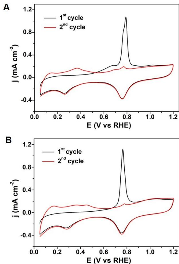
**Figure S6.** CO stripping voltammograms of (A) Pd concave cubes/C and (B)  $\beta$ -PdH concave cubes/C, respectively in a 1 M KOH solution with a scan rate of 10 mV s<sup>-1</sup>.
