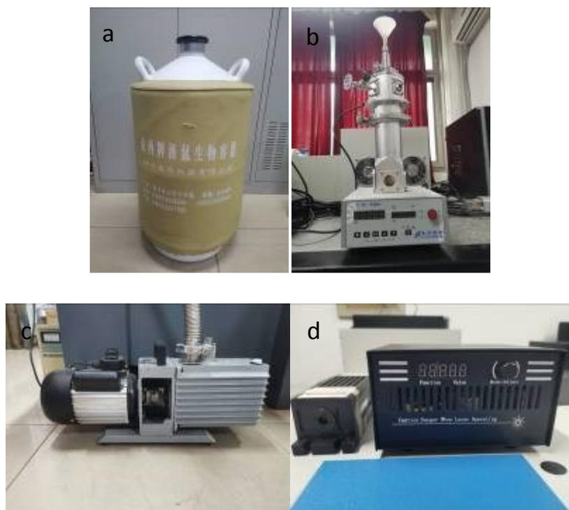
**Fig. S1** (a) Liquid nitrogen tank. (b) Temperature controller equipment and sample chamber. (c) Vacuum pump.
