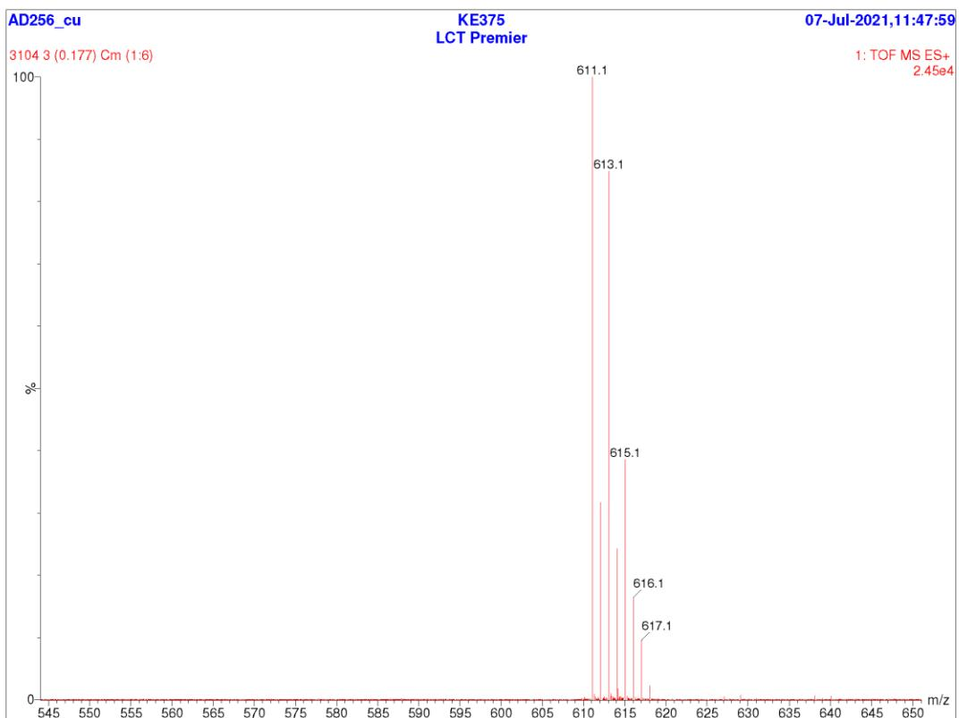
Figure S46. LRMS (ESI+) of **1a**, 611.1 [M-Cl]<sup>+</sup>.
