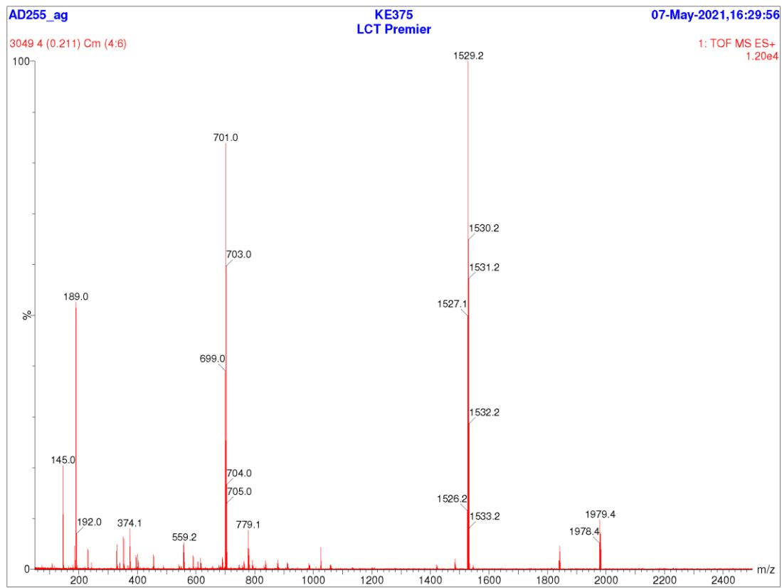
Figure S55. LRMS (ESI+) of **5a**, full spectrum.
