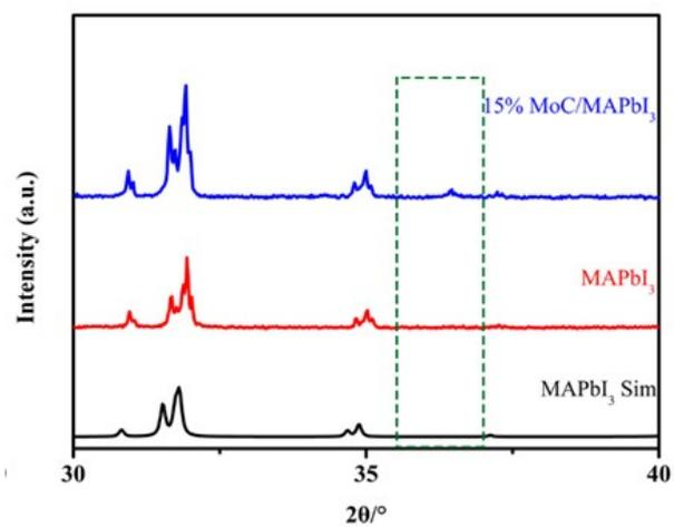
Figure S2. Partial XRD enlarged view of MAPbI<sub>3</sub> and MoC/MAPbI<sub>3</sub>
