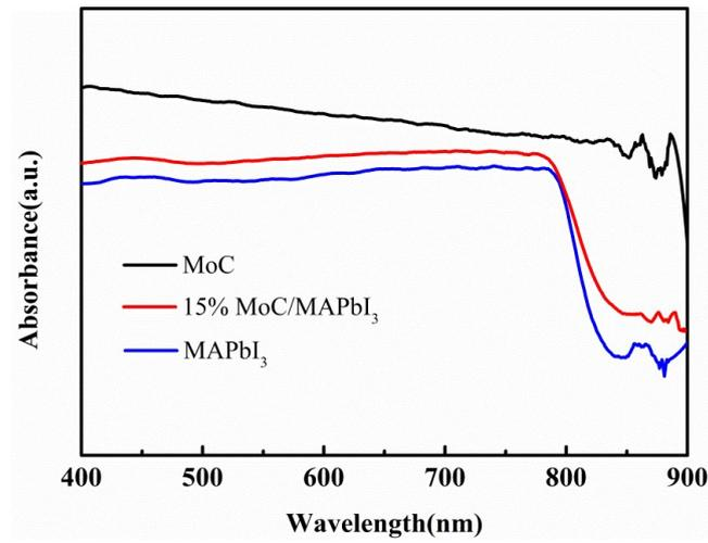
Figure S4. Absorption spectra of MoC, MAPbI<sub>3</sub>, MoC/MAPbI<sub>3</sub>
