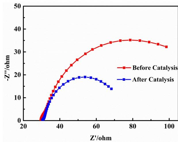
Figure S11. Nyquist plots of 15% MoC/MAPbI<sub>3</sub> composites before catalysis and after 16 h catalysis
