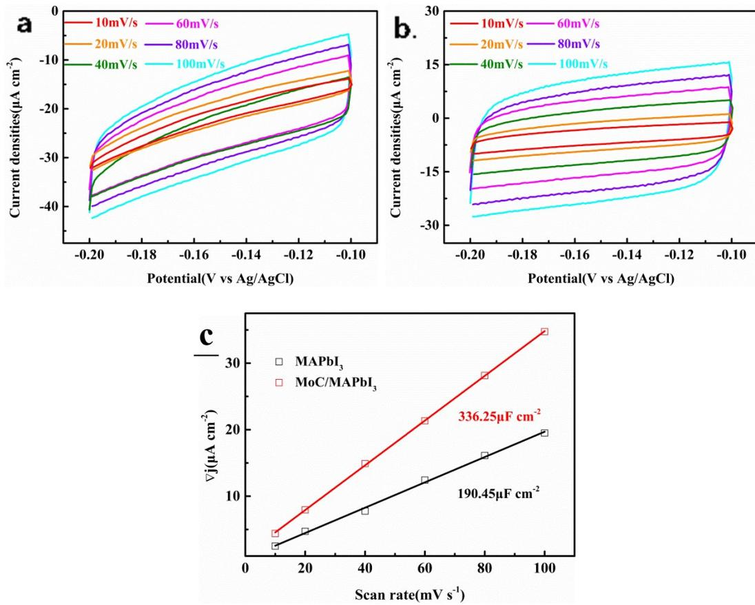
Figure S5. CV curves of MAPbI<sub>3</sub> (a) and MoC/MAPbI<sub>3</sub> after catalysis (b) tested in the non-faradaic region of -0.2 to -0.1 V vs. Ag/AgCl at various scan rates. (c) The corresponding capacitive currents densities at -0.15 V vs. Ag/AgCl as a function of scan rate.
