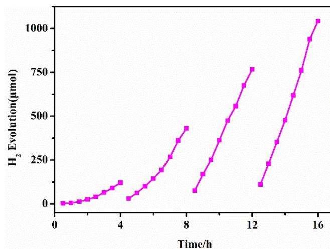
Figure S8. Cycling photocatalytic H<sub>2</sub> evolution performance of the MAPbI<sub>3</sub>/MoC hybrid of 4 cycles (4 h for each cycle) under visible-light illumination ( $\lambda \geq 420$  nm).
