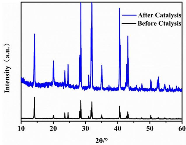
Figure S10. XRD patterns of MoC/MAPbI<sub>3</sub> before and after photocatalytic HI splitting reaction
