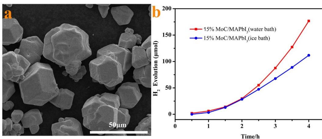
Figure S7. a) SEM image of MAPbI<sub>3</sub> synthesis through ice bath and b) comparison of hydrogen production by MAPbI<sub>3</sub> with different particle sizes.
