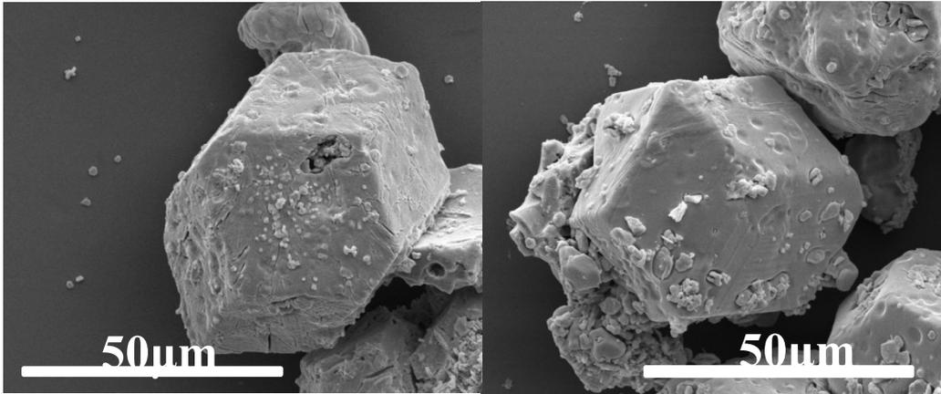
Figure S9. SEM images of MoC/MAPbI<sub>3</sub> composites after 16 h photocatalytic reaction
