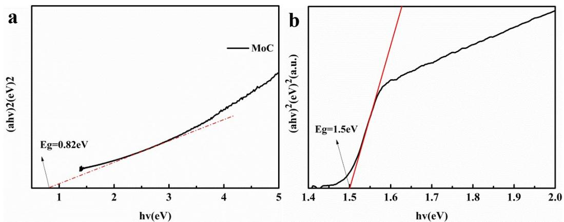
Figure S12. Band gap determination of the a) MoC and b) MAPbI<sub>3</sub> powder
