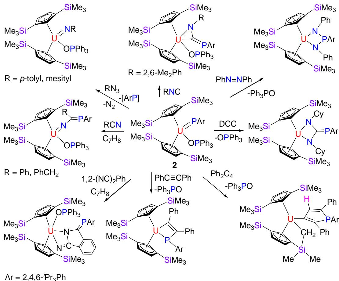
**Figure S4.** Selected reactivity of  $[\eta^5\text{-1,3-(Me}_3\text{Si)}_2\text{C}_5\text{H}_3]_2\text{U}(=\text{P-2,4,6-}i\text{Pr}_3\text{C}_6\text{H}_2)(\text{OPPh}_3)$ .
