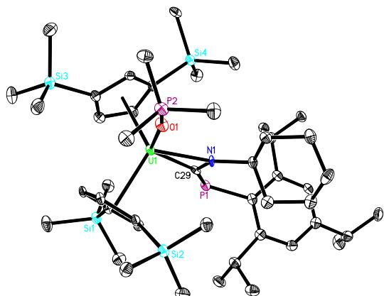
**Figure S7.** Molecular structure of **15** (thermal ellipsoids drawn at the 35% probability level).
