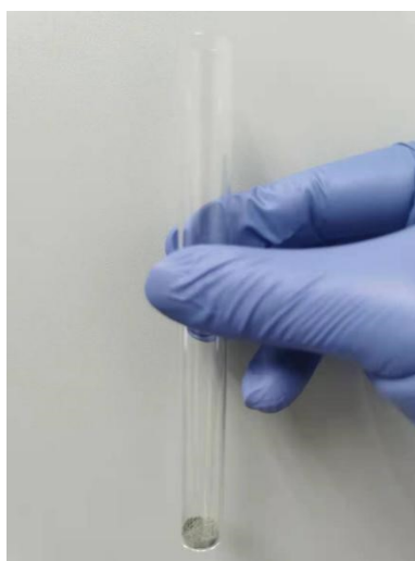
Figure S1 Schematic of quartz ampoule with the well-mixed reactants inside.
