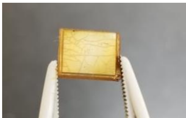
Fig. S62. Photograph of a golden-colored Ge thin film deposited on a polyethylene terephthalate (PET) substrate ( 0.7 \times 0.8 mm, initially transparent and colorless). Deposition conditions: three equivalents of \text{H}_3\text{B}\cdot\text{SMe}_2 (2.0 M solution in THF) were combined with a 0.014 M solution of [\text{Ge}(\text{O}^t\text{Bu})_2] ( 1 ) in 1.5 mL of toluene with heating to 70 °C for 1 hr.
