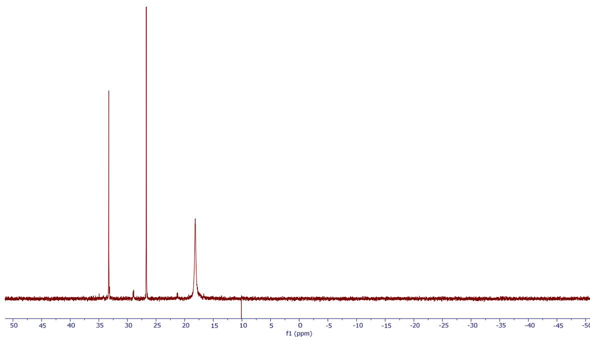
**Figure S45.** <sup>31</sup>P{<sup>1</sup>H} NMR spectrum (162 MHz, CDCl<sub>3</sub>) of the reaction mixture obtained by mixing (**1**<sup>iPr</sup>H)Cl (2 equiv.) and [PdCl<sub>2</sub>(MeCN)<sub>2</sub>] (1 equiv.). The major product is **9**-Cl.
