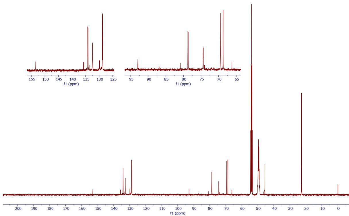
**Figure S50.**  $^{13}\text{C}\{^1\text{H}\}$  NMR spectrum (101 MHz,  $\text{CD}_2\text{Cl}_2/\text{CD}_3\text{OD}$ ) of **10**
