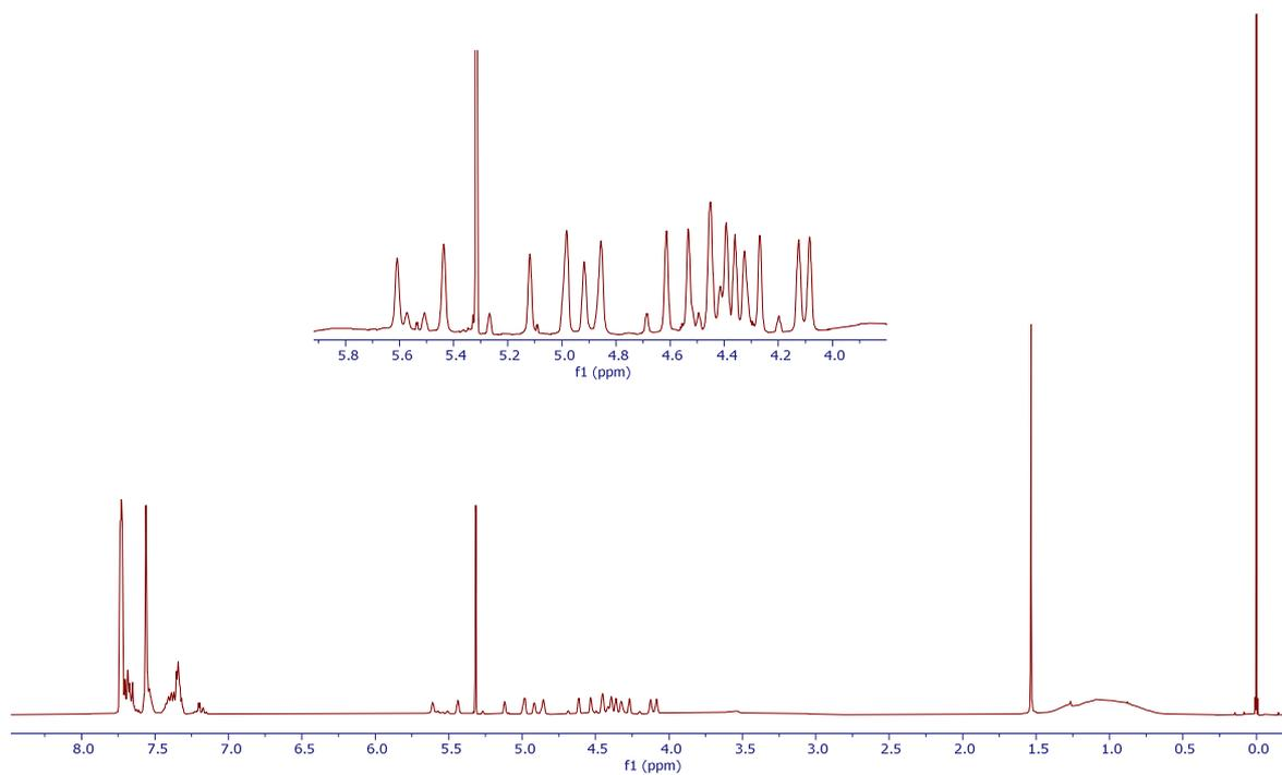
**Figure S34.** <sup>1</sup>H NMR spectrum (400 MHz, CD<sub>2</sub>Cl<sub>2</sub>) of **5**. The spectrum was recorded immediately after dissolving a crystalline sample.
