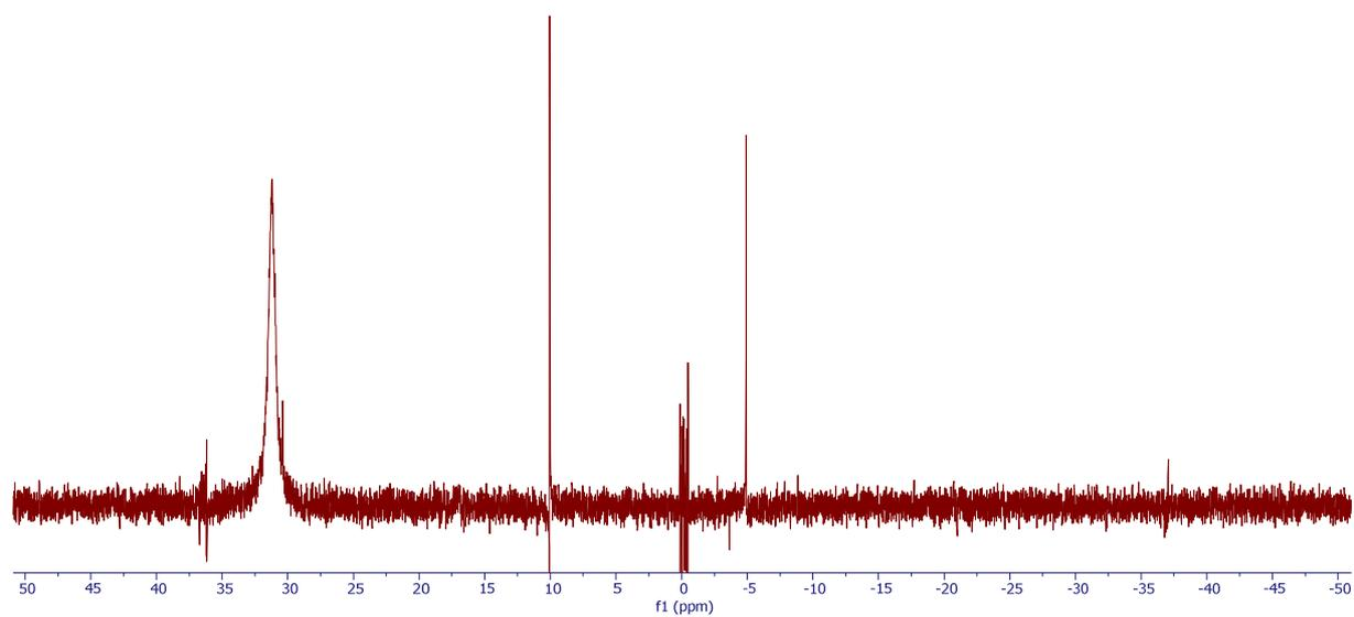
**Figure S51.**  $^{31}\text{P}\{^1\text{H}\}$  NMR spectrum (162 MHz,  $\text{CD}_2\text{Cl}_2/\text{CD}_3\text{OD}$ ) of **10**. The sharp signals at 10 ppm and near 0 ppm are spikes (electronic artefacts).
