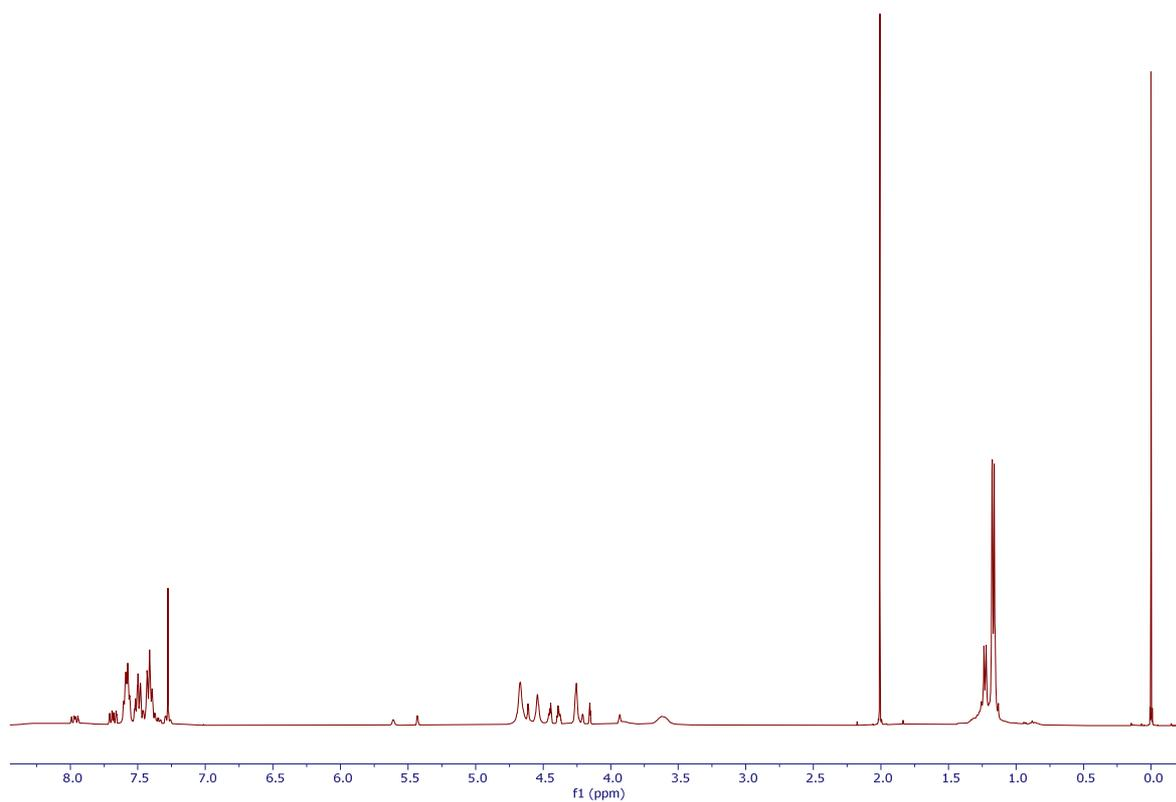
**Figure S44.** <sup>1</sup>H NMR spectrum (400 MHz, CDCl<sub>3</sub>) of the reaction mixture obtained by mixing (**1**<sup>iPr</sup>H)Cl (2 equiv.) and [PdCl<sub>2</sub>(MeCN)<sub>2</sub>] (1 equiv.). The major product is **9**-Cl.
