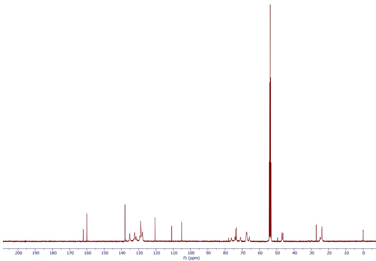
**Figure S39.**  $^{13}\text{C}\{^1\text{H}\}$  NMR spectrum (101 MHz,  $\text{CD}_2\text{Cl}_2$ ) of **6**
