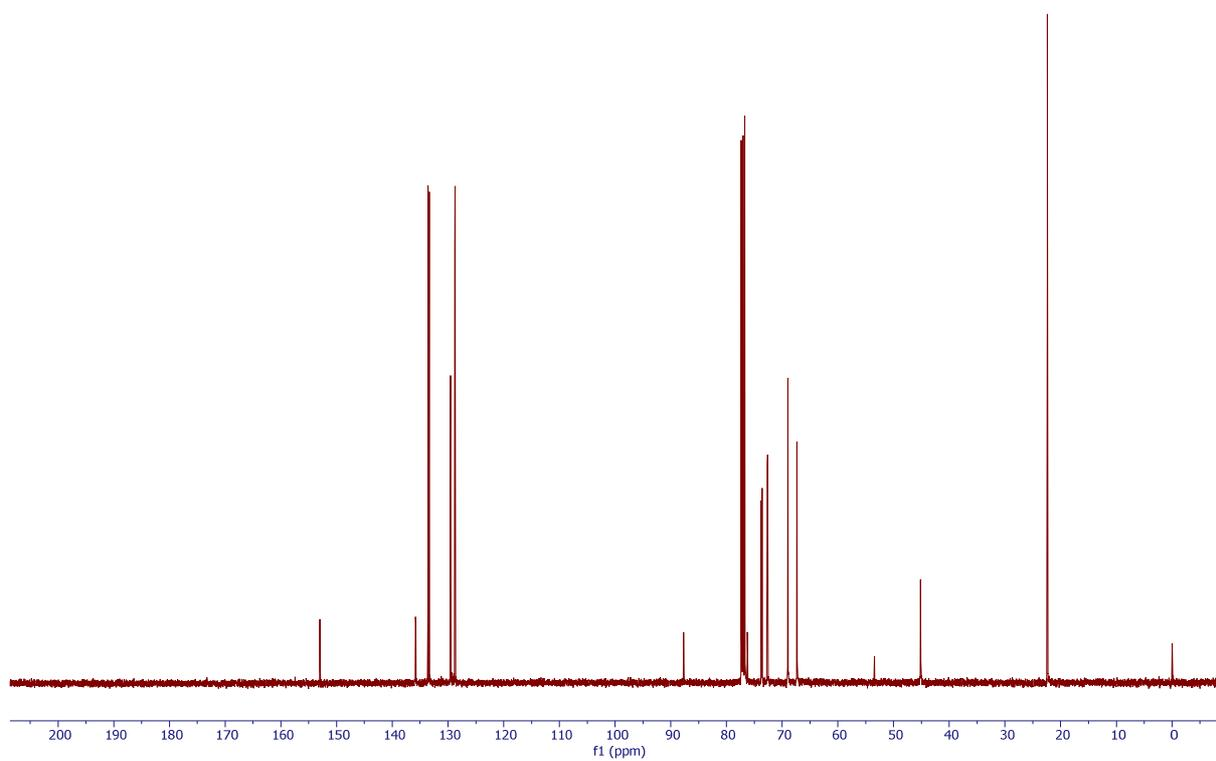
**Figure S29.**  $^{13}\text{C}\{^1\text{H}\}$  NMR spectrum (101 MHz,  $\text{CDCl}_3$ ) of  $(\mathbf{1}^{\text{iPrH}})[\text{SbF}_6]$
